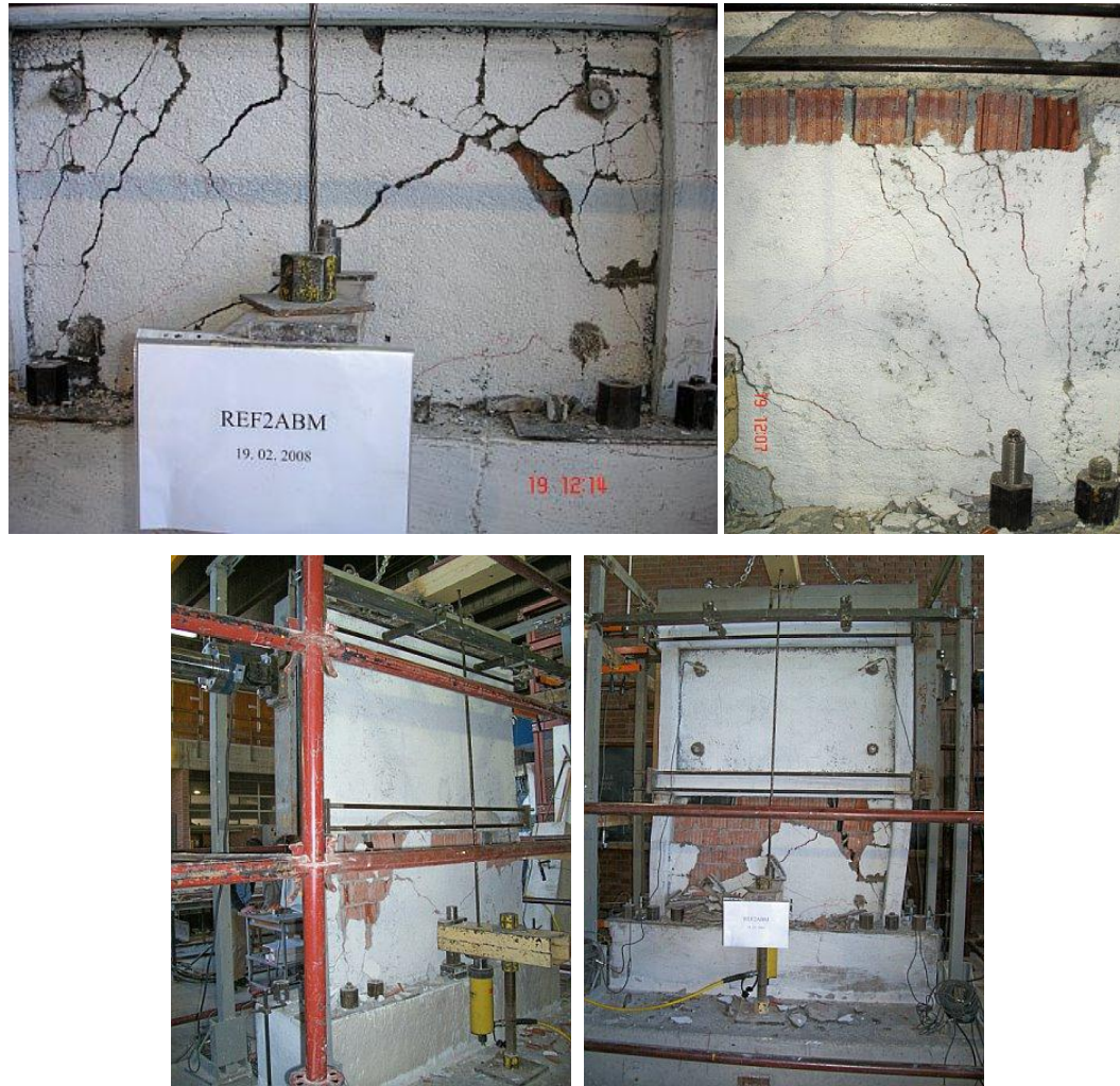
Figure 4.30 Views of TS7 (REF2ABM) Specimen during the Test
