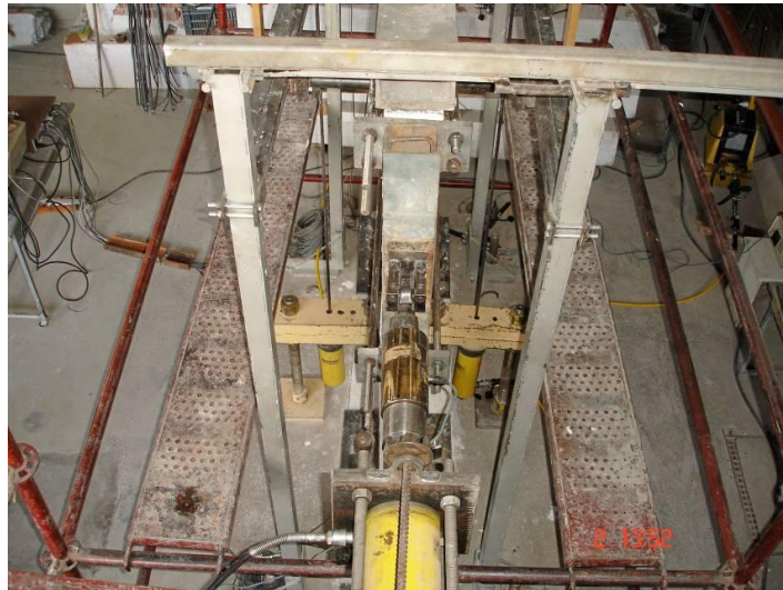
Figure 3.19 Appearance of Guide Frame
