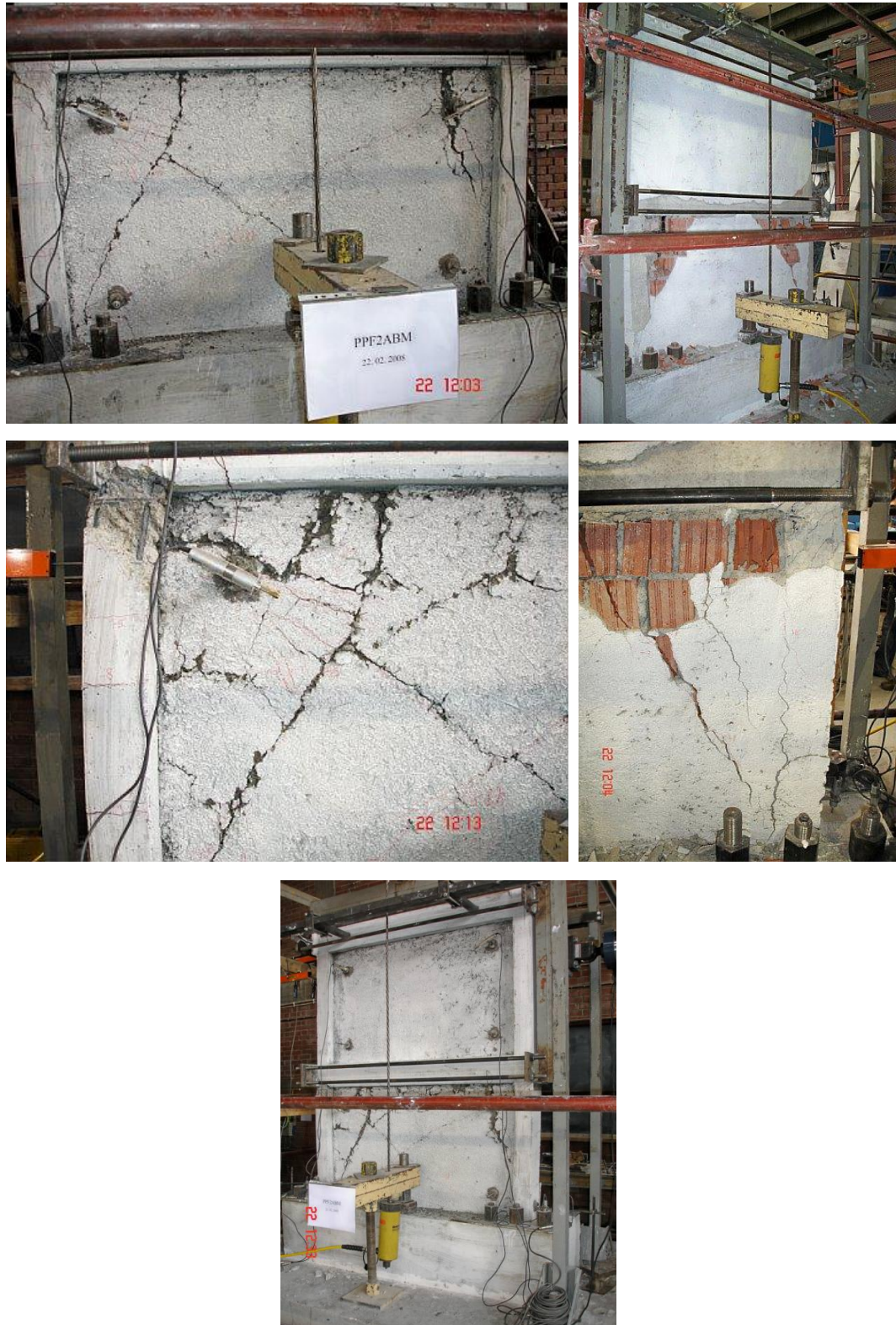
Figure 4.70 Views of TS8 (PPF2ABM) Specimen during the Test
