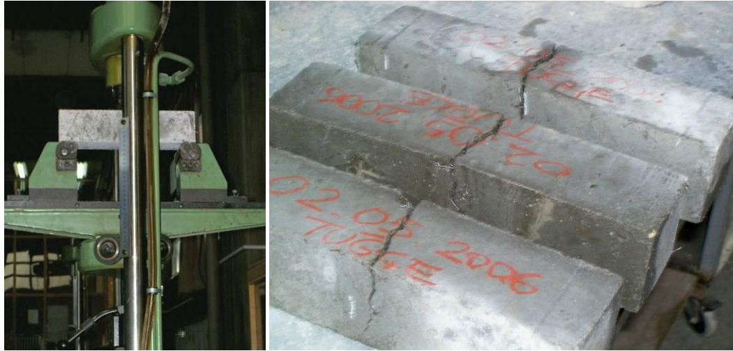
Figure 3.3 Views of Flexural Tensile Strength Testing
