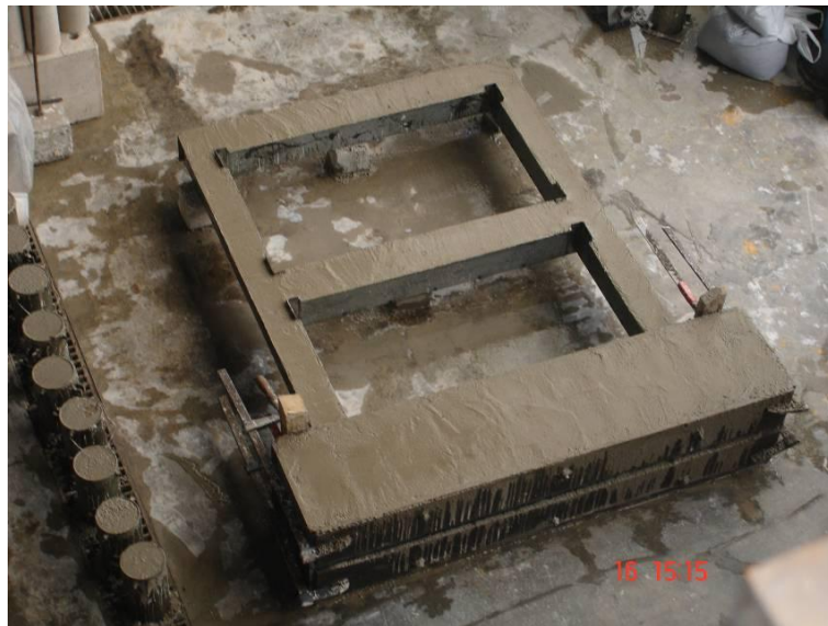
Figure 3.12 View of Frame Specimen after Concrete Casting
