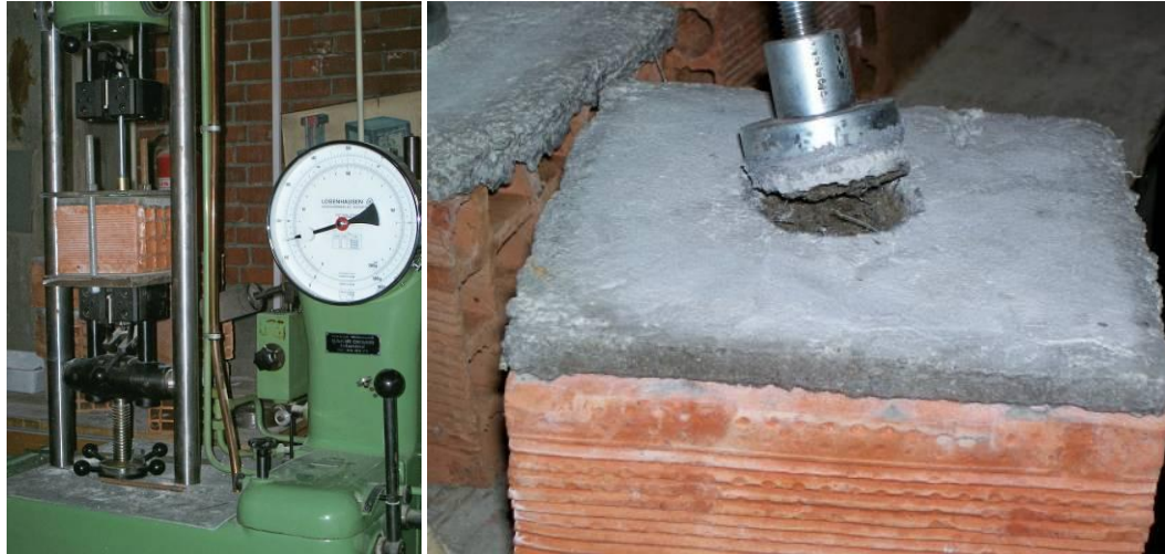
Figure 3.4 Views of Adhesion Strength Testing
