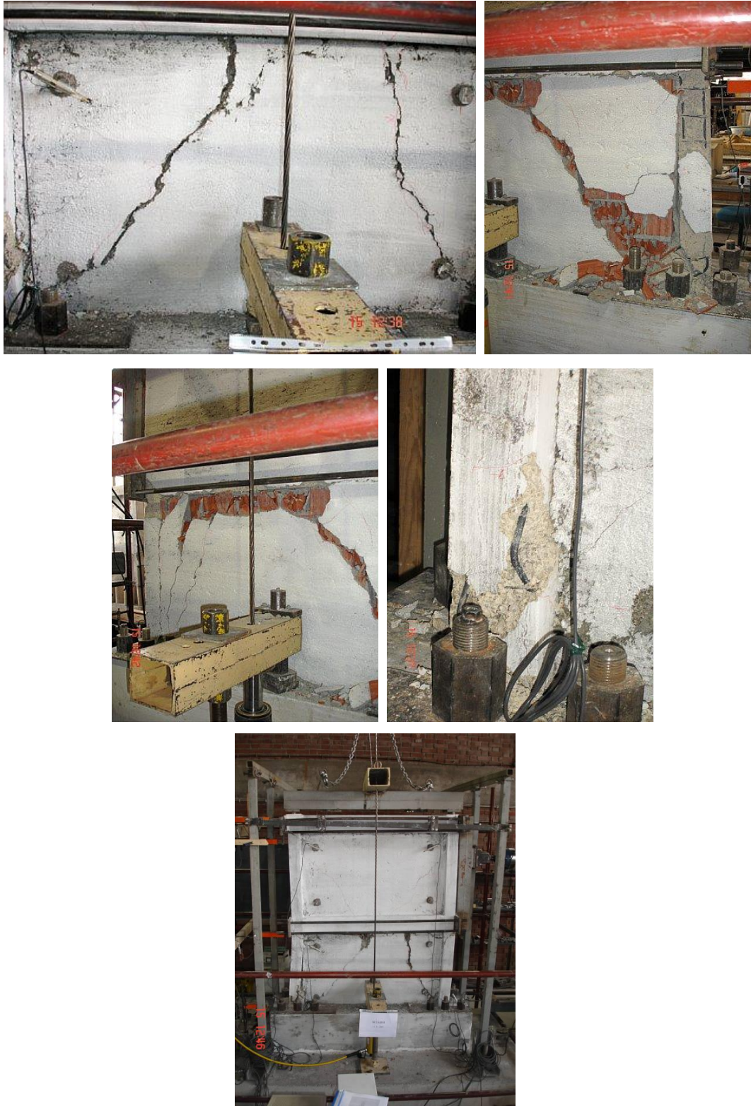
Figure 4.62 Views of TS4 (SF2ABM) Specimen during the Test
