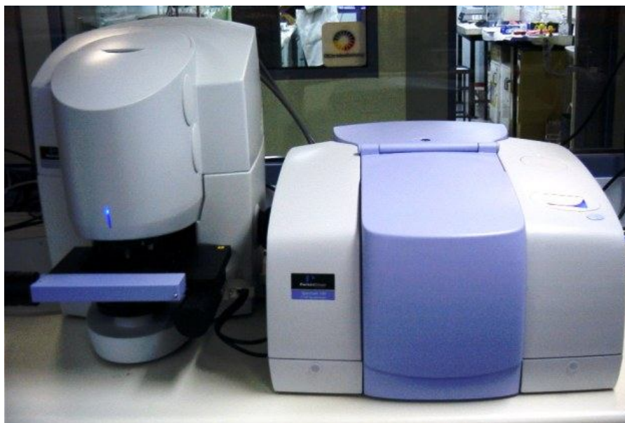
Figure 8. Perkin Elmer Spectrum Spotlight 400 imaging FTIR microscope
