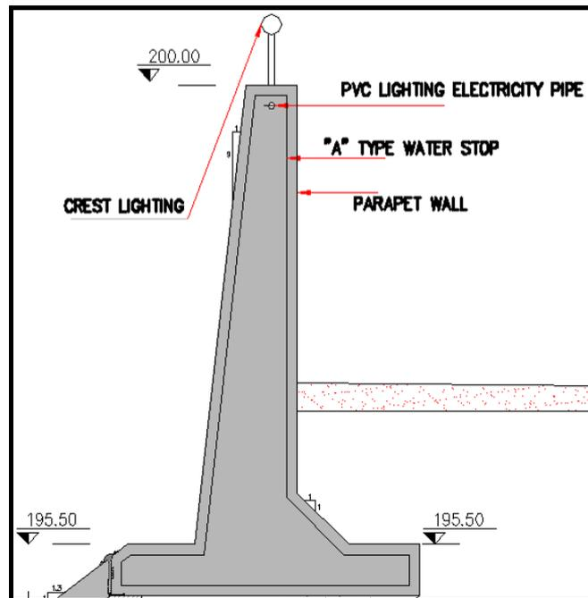
Figure 4.12 Details of parapet wall for Gökçeler Dam
