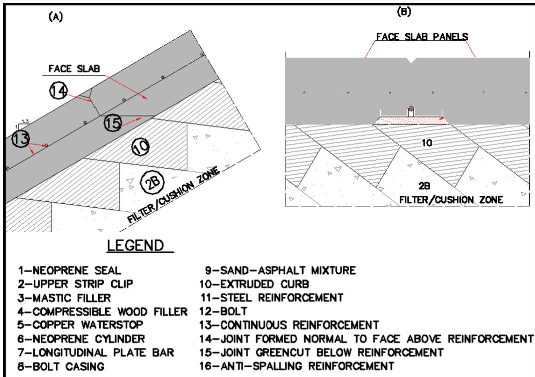
Figure 4.11 Horizontal construction and vertical contraction joints (Hidro Dizayn, 2007-c)
