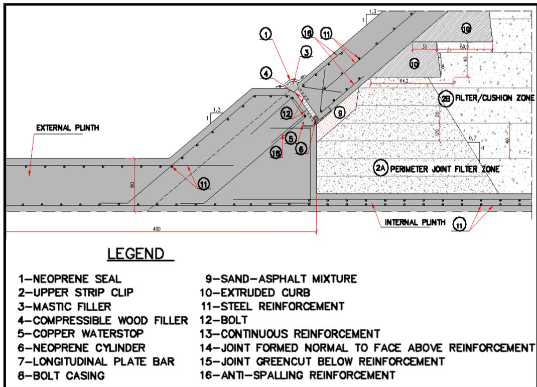
Figure 4.9 Horizontal plinth cross-section of Gökçeler Dam (Hidro Dizayn, 2007-c)
