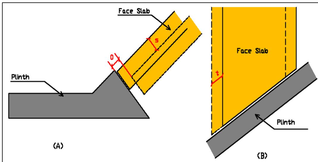
Figure 2.11 Perimeter joint movements (Hedien, 2005-a)
