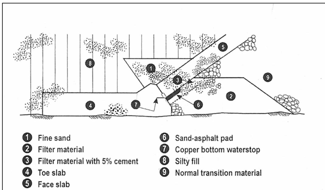
Figure 2.13 Upper barrier of cohesionless fine deposit (Hedien, 2005-a)
