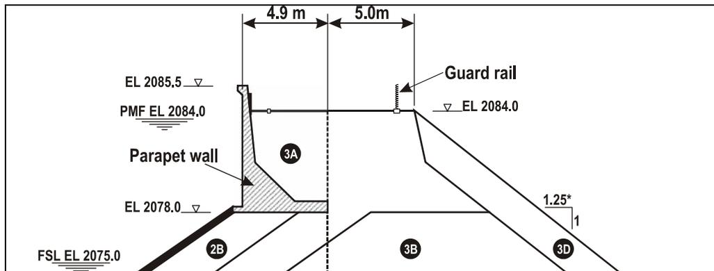
Figure 2.16 Parapet wall of Mohale Dam (Sundaram and Kleiner, 2005)
