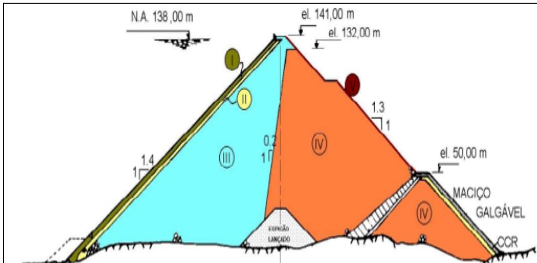
Figure 3.9 Main cross-section of Xingó Dam (Souza, 2007)
