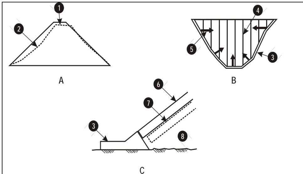
Figure 2.14 Embankment and face slab behavior (Hedien, 2005-b)
