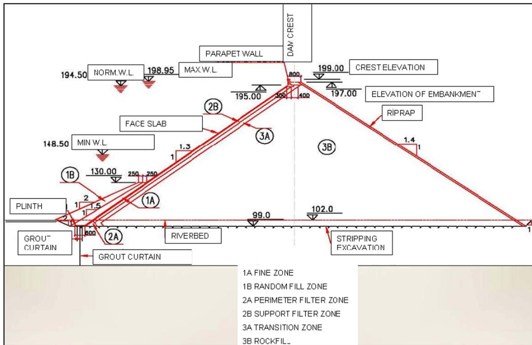
Figure 4.8 Main cross-section of CFRD type (Hidro Dizayn, 2007-b)
