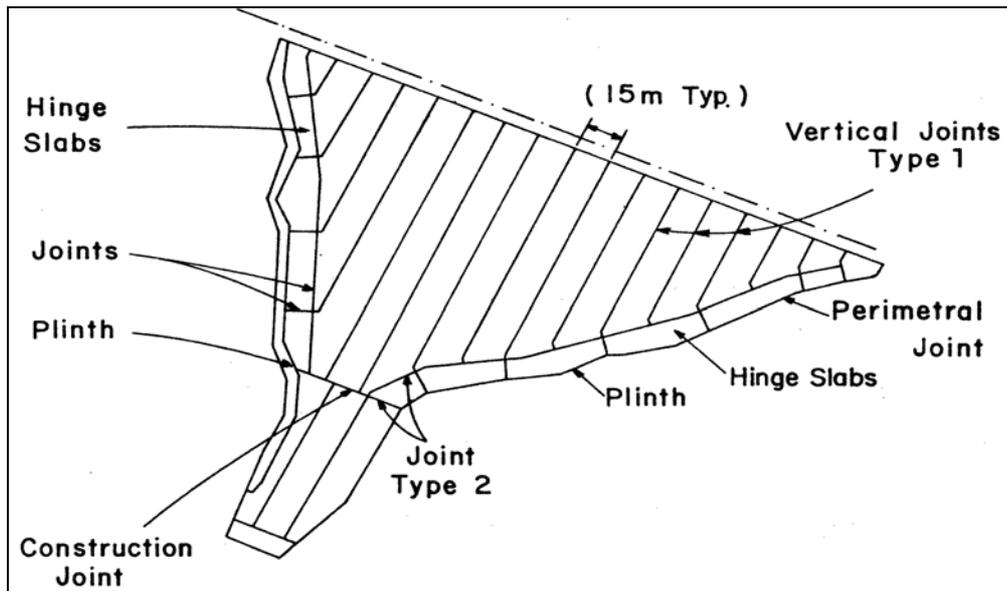
Figure 3.5 Face slab layout of Alto Anchicaya Dam (Materon, 1985).
