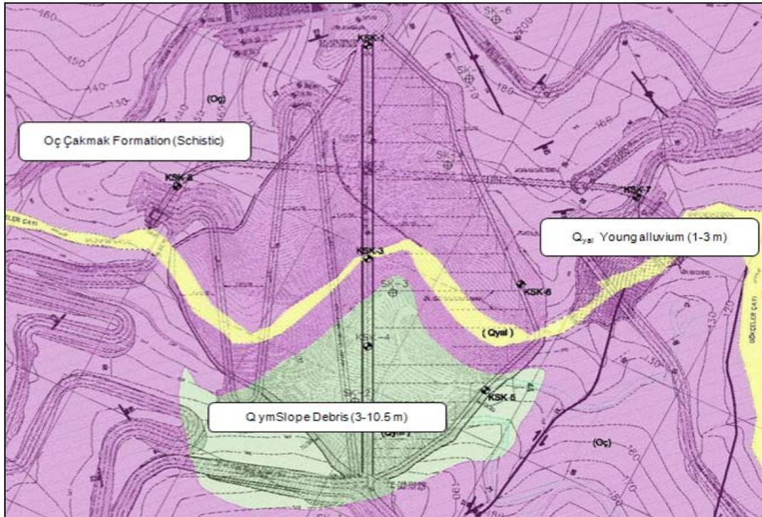
Figure 4.3 Geologic layout of Gökçeler Dam site ( Hidro Dizayn, 2007-b)
