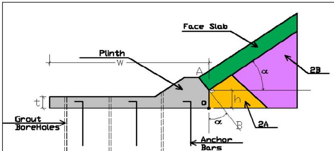
Figure 2.6 Basic geometry of conventional plinth (Cooke, 2000-b).
