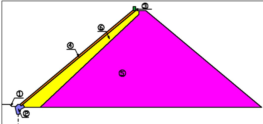
Figure 2.1 Features of traditional CFRD design (ICOLD, 1989-b)
