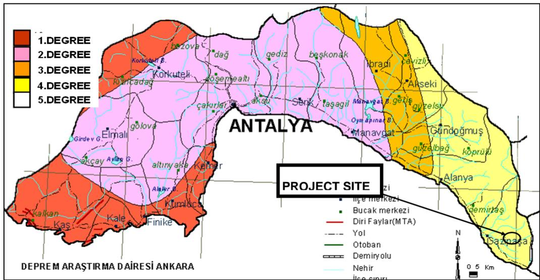
Figure 4.4 Earthquake map of Antalya (Hidro Dizayn, 2007-b)
