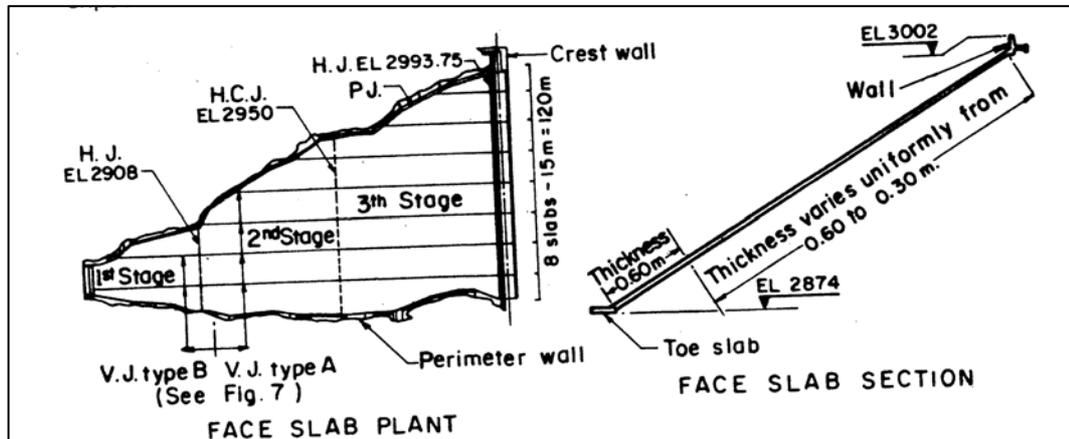
Figure 3.6 Face slab layout of Golillas Dam (Marulanda and Amaya, 1985)
