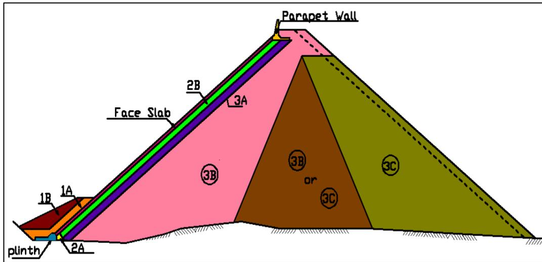
Figure 2.4 Current cross-section of conventional CFRD (Kleiner, 2005-c)
