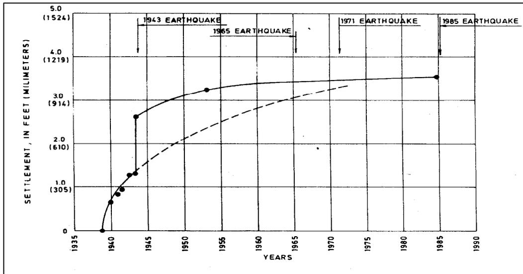
Figure 3.3 Crest settlement curve for Cogoti Dam (Arrau et al., 1985).
