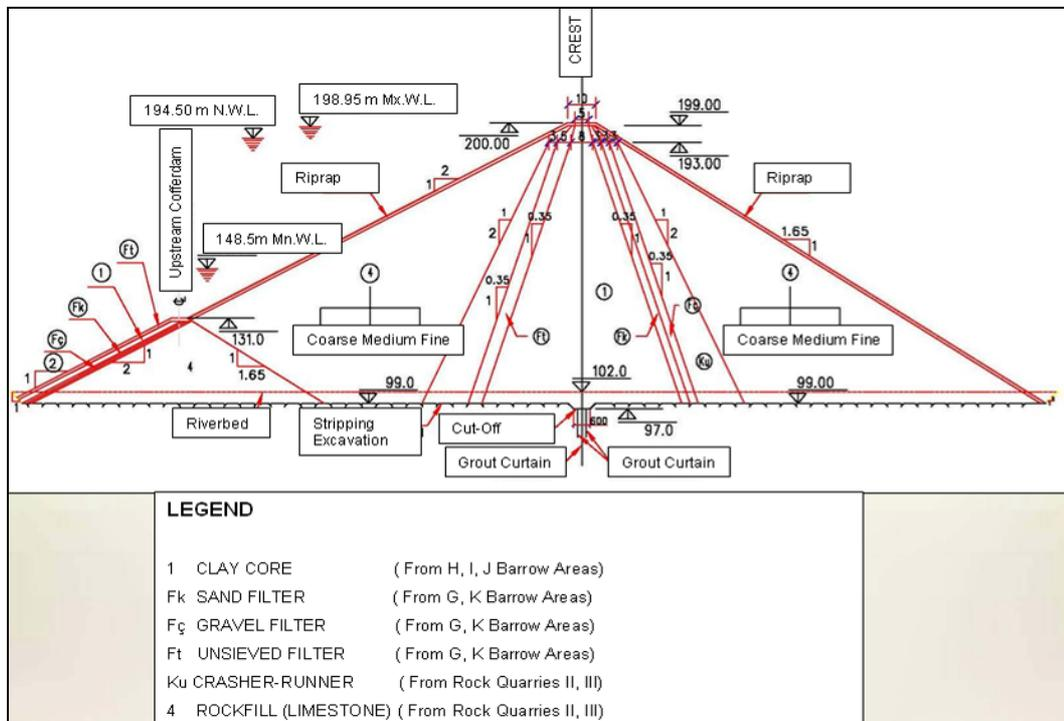
Figure B.2 Main cross-section ECRD type (Hidro Dizayn, 2007-b)
