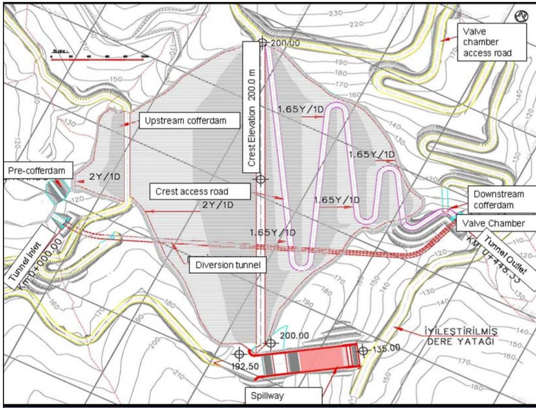
Figure B.1 General layout of ECRD formulation (Hidro Dizayn, 2007-b)
