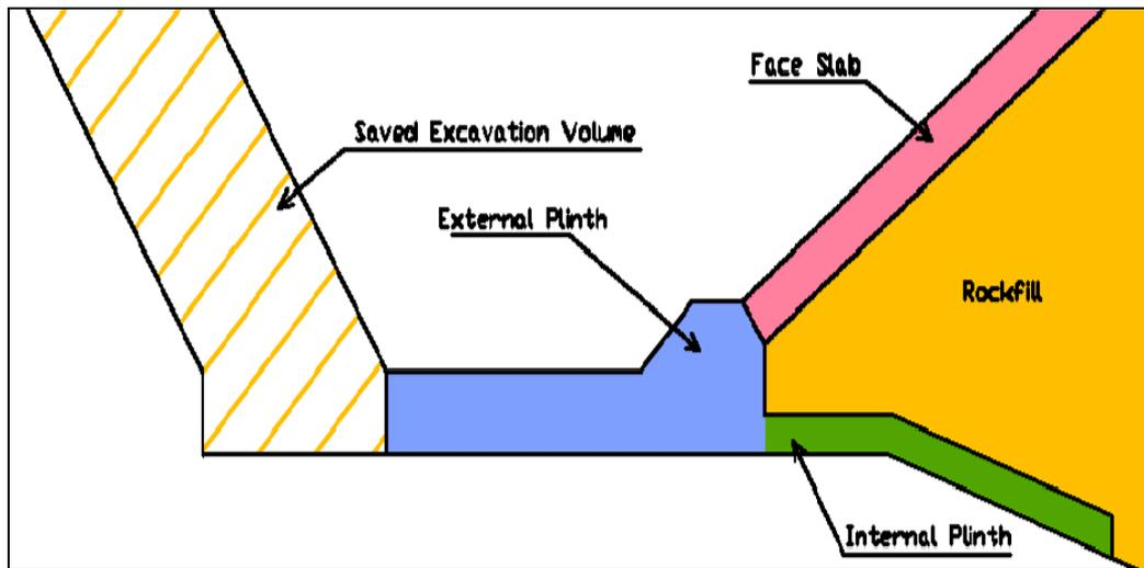
Figure 2.8 Internal and external plinth combination (Kleiner, 2005-d)
