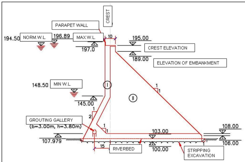
Figure C.2 Main cross-section of RCC type (Hidro Dizayn, 2007-b)
