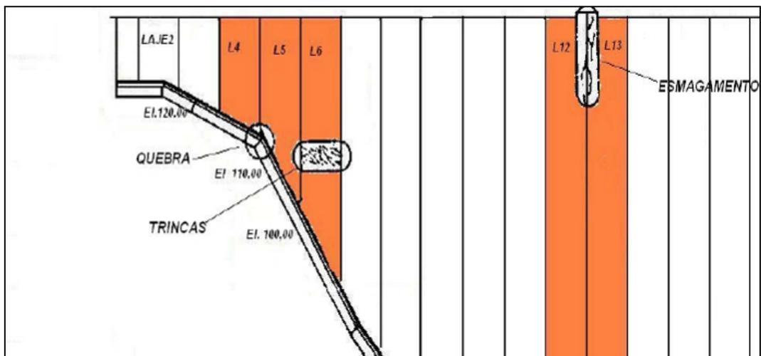
Figure 3.11 Face slab cracks of Xingó Dam (Souza, 2007)
