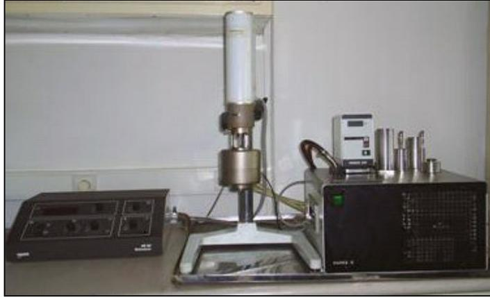
Figure 4.1 Haake viscometer
