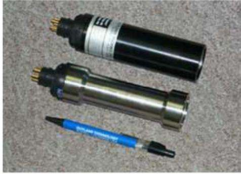
Figure 7.2: Outland Tech. UWC-300 underwater cameras (black cylinder, top)
