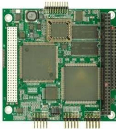
Figure 7.1: Eurotech CTR-1472 frame grabber and MPEG-4 Compressor
