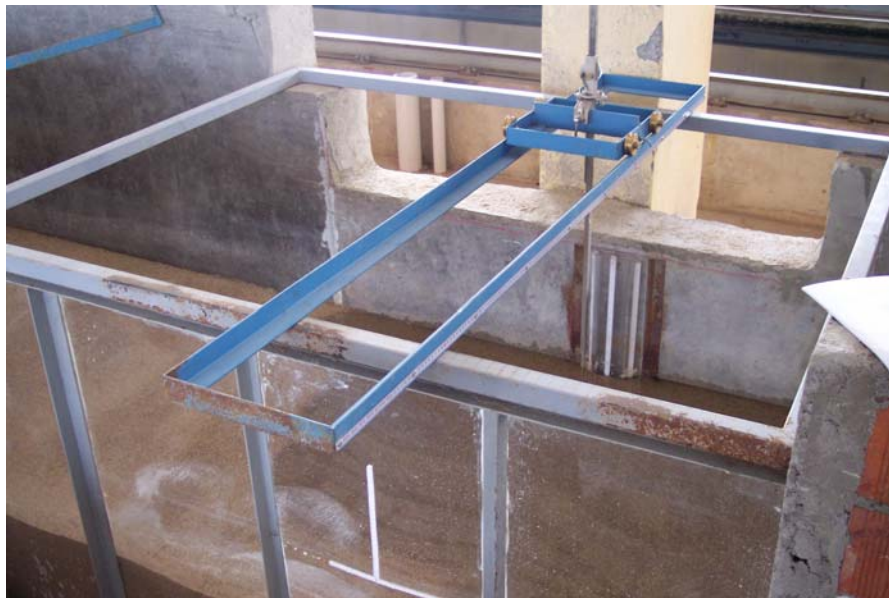
Figure 3.3. Measurement equipment for taking scour hole coordinates
