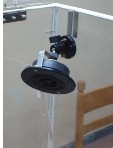
Figure 5.8 – Microphone and preamplifier attached to the holder (left) and one of the loudspeakers (right)
