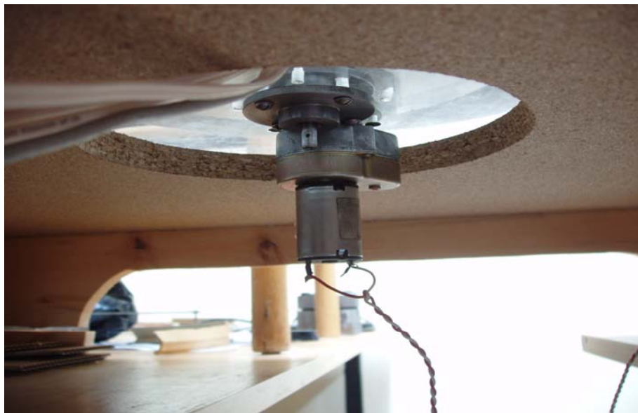
Figure 5.7 – Bottom view of the reverberation room and the DC motor
