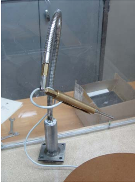
Figure 5.8 – Microphone and preamplifier attached to the holder (left) and one of the loudspeakers (right)
