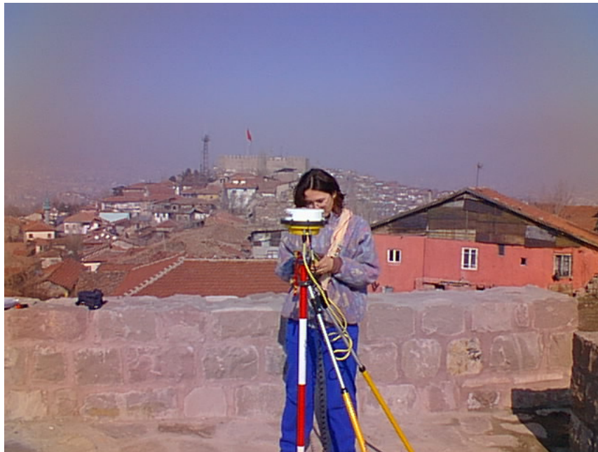
Figure 2. Nurdan Atalan is setting up base station of the GPS receiver
