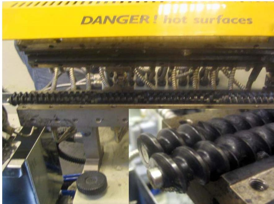
**Figure 3.7-b** Screw Configuration of Thermo Prism TSE 16 TC twin screw extruder
