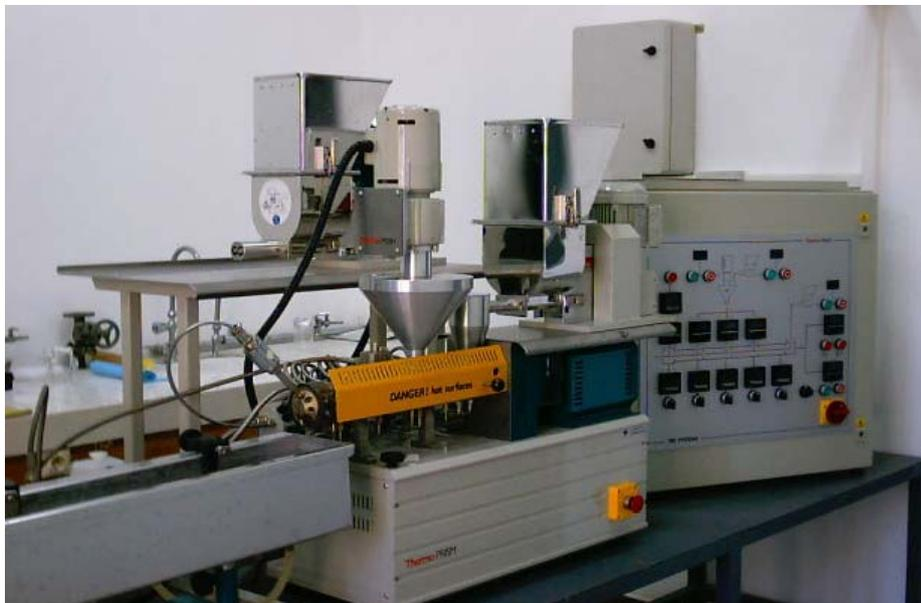
**Figure 3.7-a** Thermo Prism TSE 16 TC twin screw extruder
