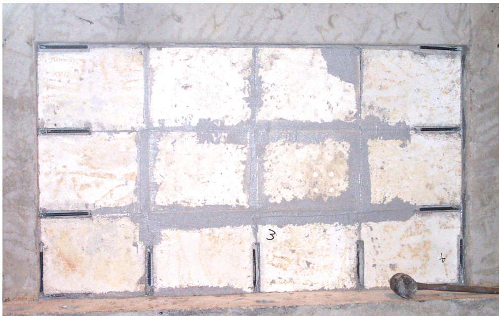
Figure 4.21. Type C panels before filling the gaps with epoxy mortar, Specimen CIC3
