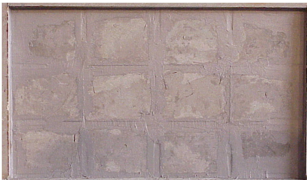
Figure 4.25. Type C panels after filling the gaps with epoxy mortar, Specimen CIC4
