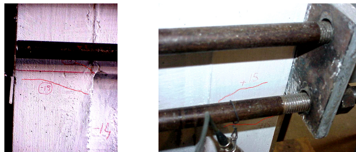
Figure 5.54. Cracks at first story beam-column joints in the tenth cycle
