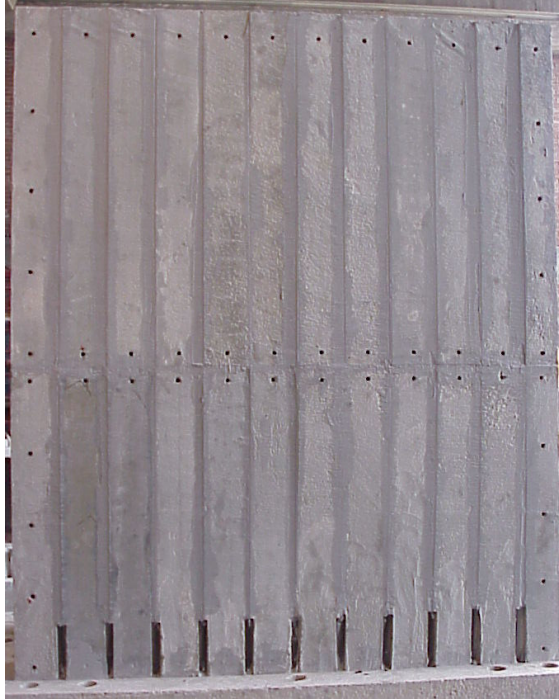
Figure 4.33. Specimen CEF4 before filling the gaps between the adjacent panels around the anchorage bars with epoxy mortar and placing \phi 8 bolts
