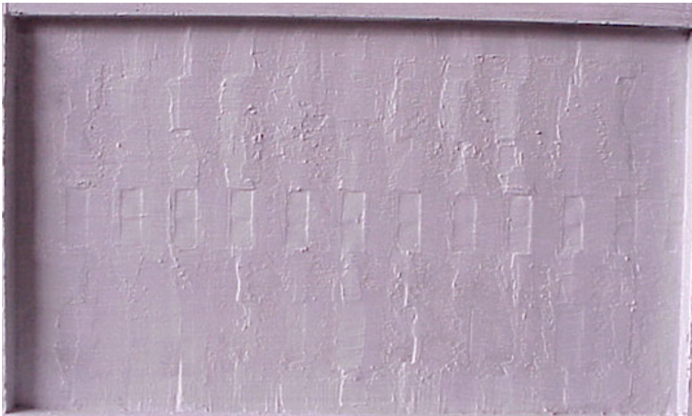
Figure 4.9. Type B panels after filling the gaps with epoxy mortar
