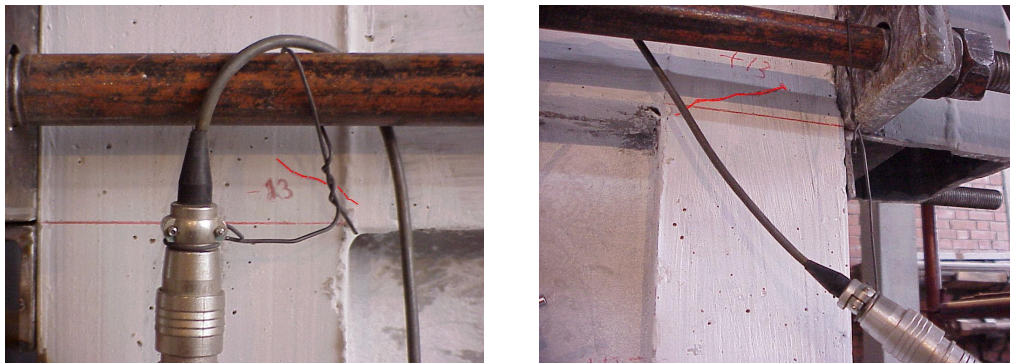
Figure 5.73. First crack at first story beam-column joints in the thirteen cycle
