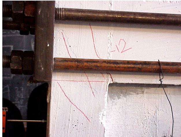
Figure 5.135. First story beam-south column joint in the twelfth forward cycle
