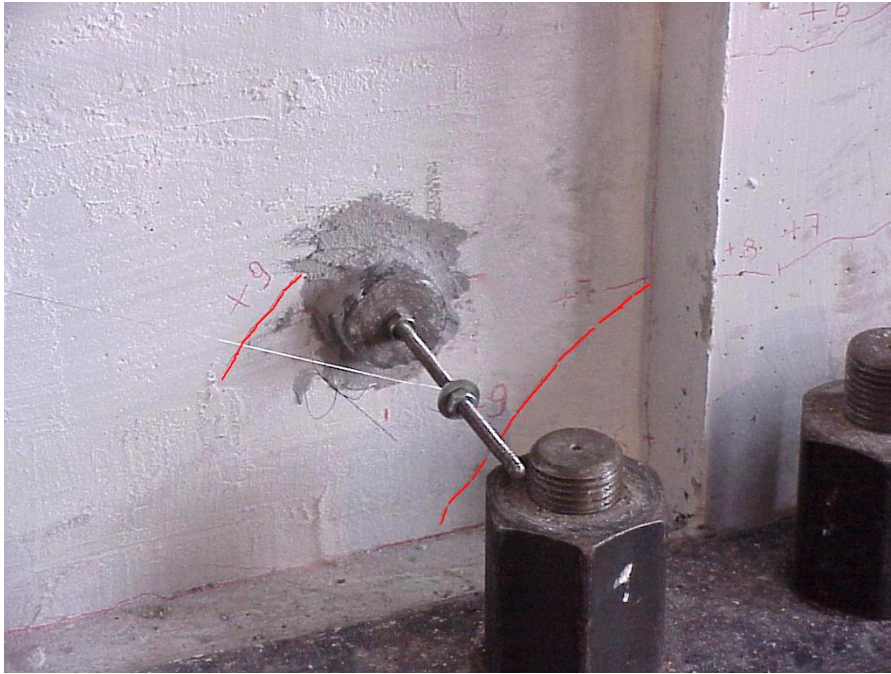
Figure 5.72. Crack occurred on the panel in the ninth forward cycle
