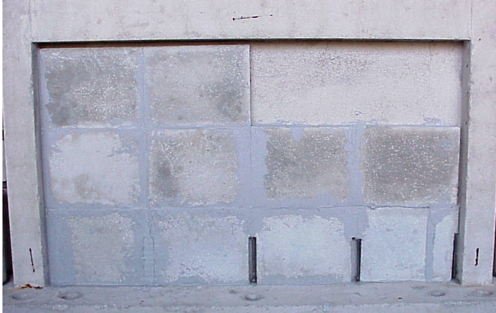
Figure 4.12. Type C panels before filling the gaps with epoxy mortar
