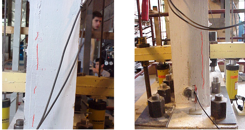
Figure 5.95. Plaster-column connection cracks in the third cycle
