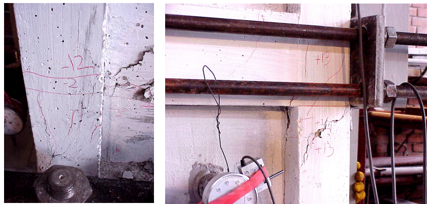
Figure 5.136. Cracks in the thirteenth forward cycle
