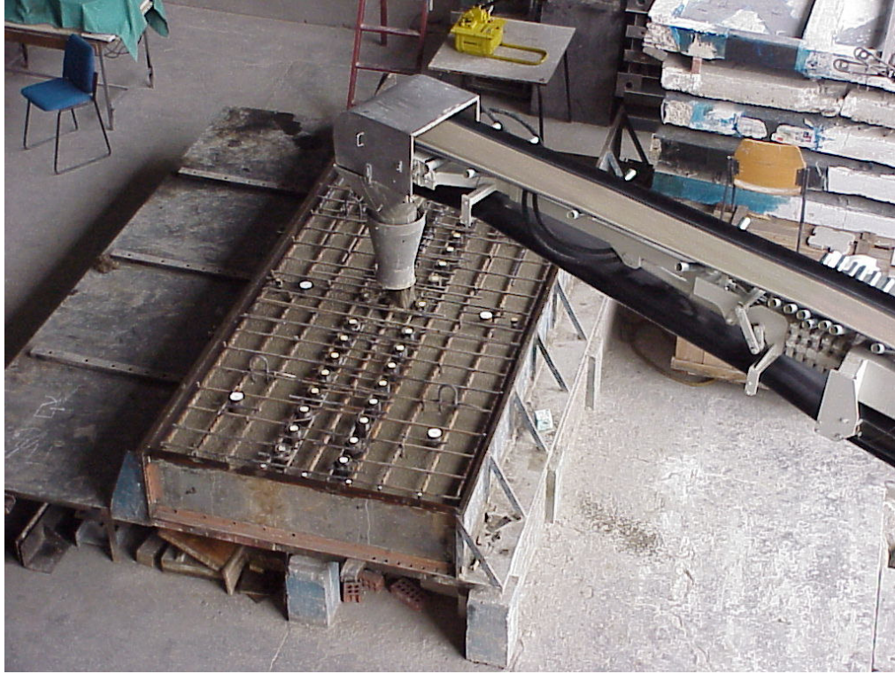
Figure 3.12. Moulding ready mixed concrete of the universal base
