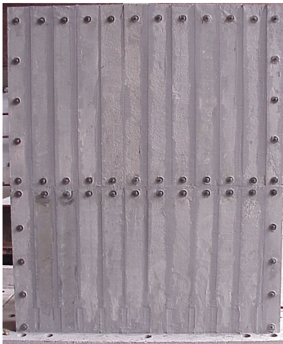
Figure 4.34. Specimen CEF4 with \phi 8 bolts
