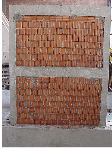
Figure 3.14. Hollow brick used as infill material
