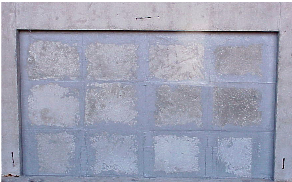
Figure 4.13. Type C panels after filling the gaps with epoxy mortar
