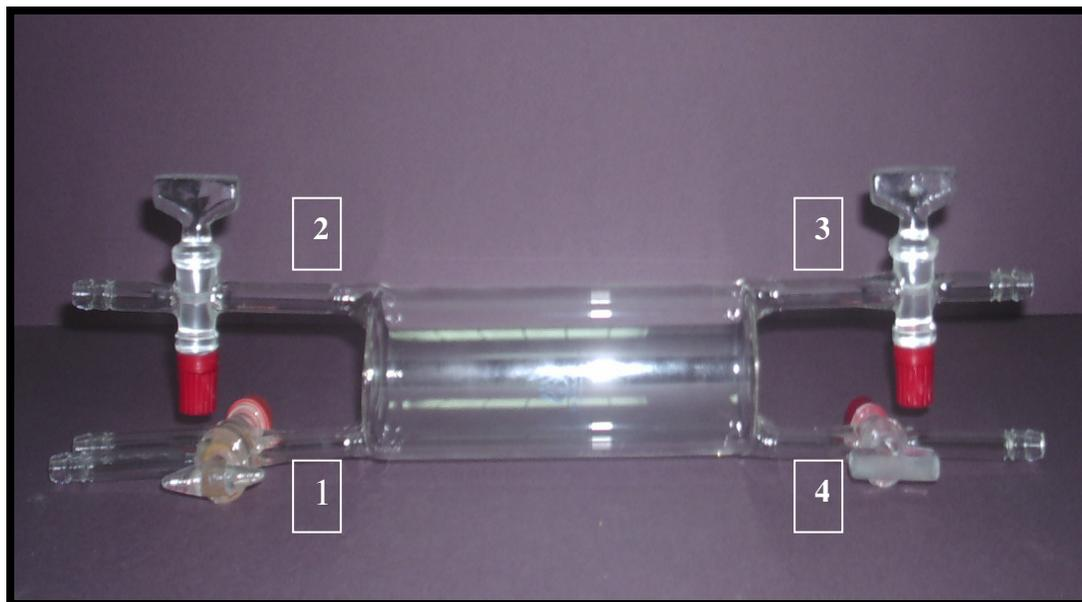
**Fig. 2.8** The Reaction Chamber Used in System 4.
