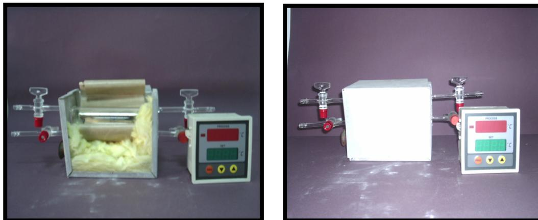
**Fig. 2.9** The Home-Made Oven Used in System 4.
