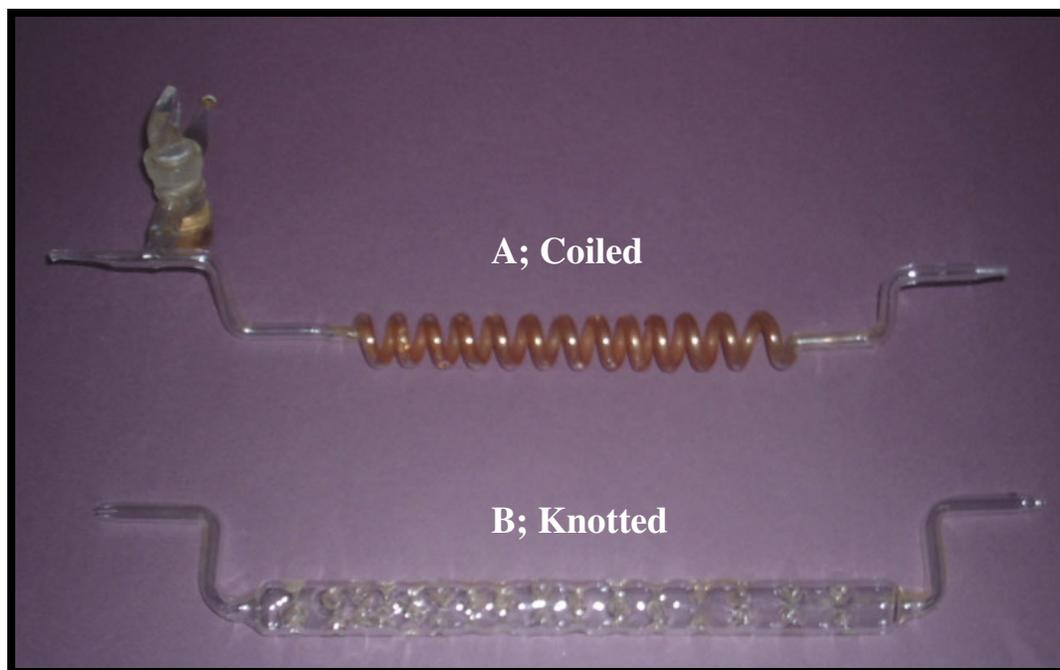
**Fig. 2.2** The Reaction Coils Used in System 1 (Coiled and Knotted).
