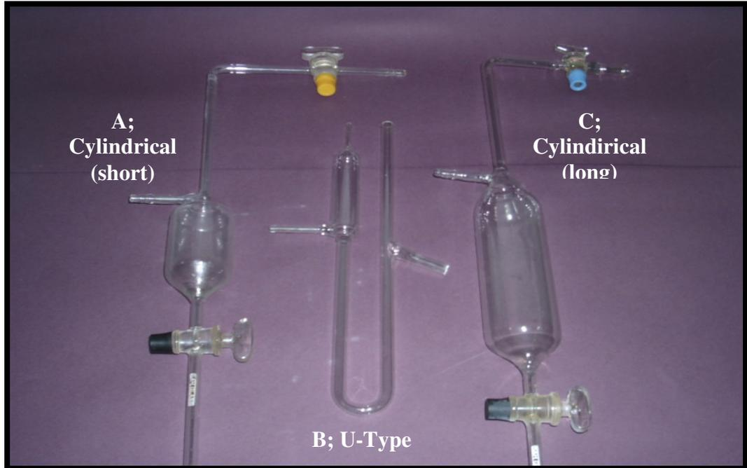
**Fig. 2.3** Different Types and Sizes of Gas-Liquid Separators Used in System 1.
