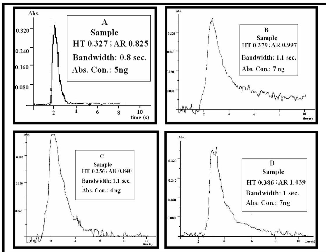
**Fig. 3.5** The sample analytical signals obtained for  $1 \mu\text{g L}^{-1}$  Ge solutions with different sample volumes
