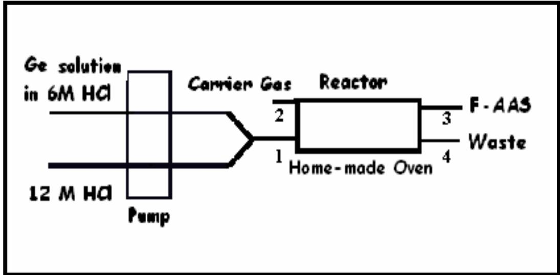
Fig. 2.10 Schematic Representation of Chloride Generation System 4.
