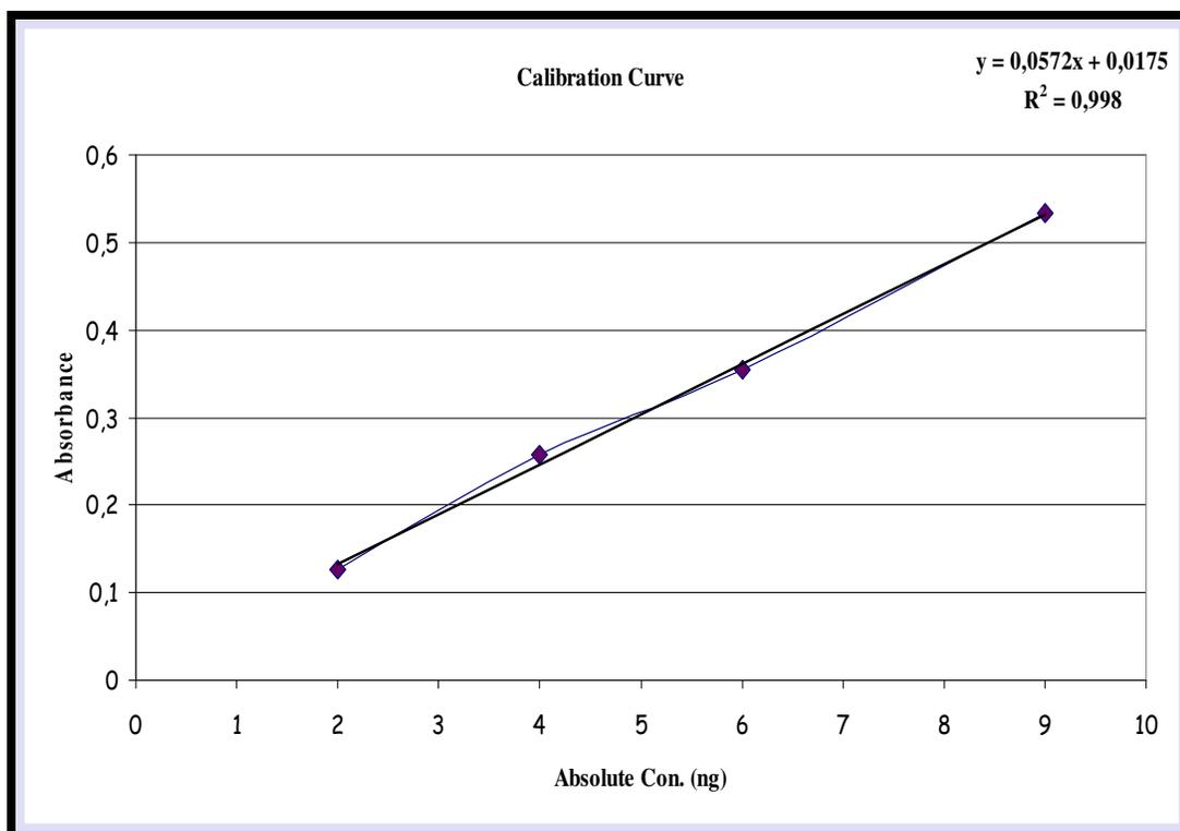
**Fig. 3.6** Calibration Graph Obtained Using Different Concentration Standards of Ge Prepared in 6 M HCl.
