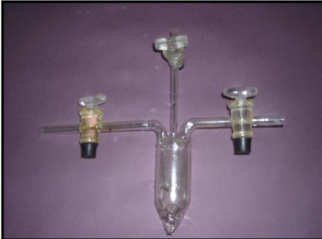
**Fig. 2.7** The Reaction Chamber Used in System 3.
