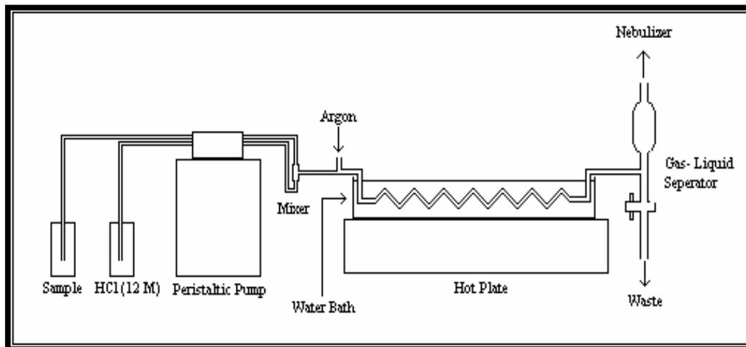
**Fig. 2.1** Schematic Representation of Chloride Generation System 1
