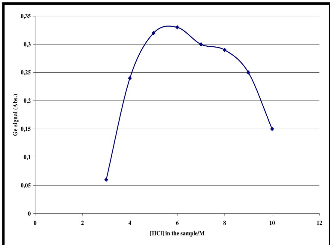
**Fig. 3.1** Influence of Sample Acidity on  $\text{GeCl}_4$  Production ( $\text{Ge}$ ,  $1\mu\text{g L}^{-1}$ , 5 mL)
