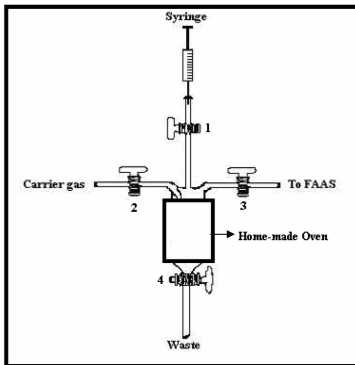
**Fig. 2.6** Schematic Representation of Chloride Generation System 3.
