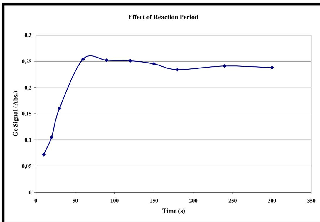
**Fig. 3.3** Effect of Reaction Period (Ge 1 $\mu$ g L<sup>-1</sup>, 4 mL)
