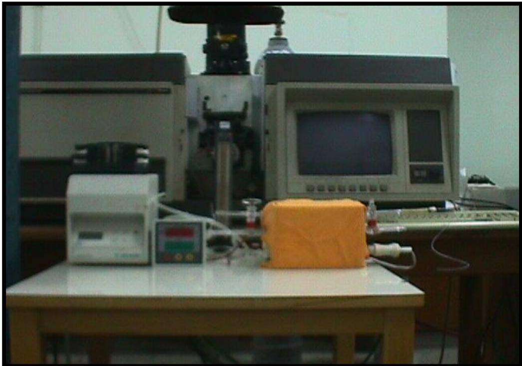
Fig. 2.11 Chloride Generation System 4 Coupled with FAAS.
