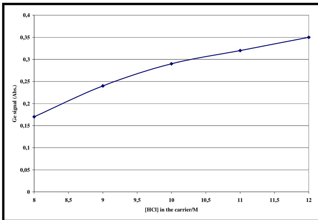
**Fig. 3.2** Influence of Carrier Acidity on  $\text{GeCl}_4$  Production ( $\text{Ge}, 1\mu\text{g L}^{-1}$ , 5 mL)
