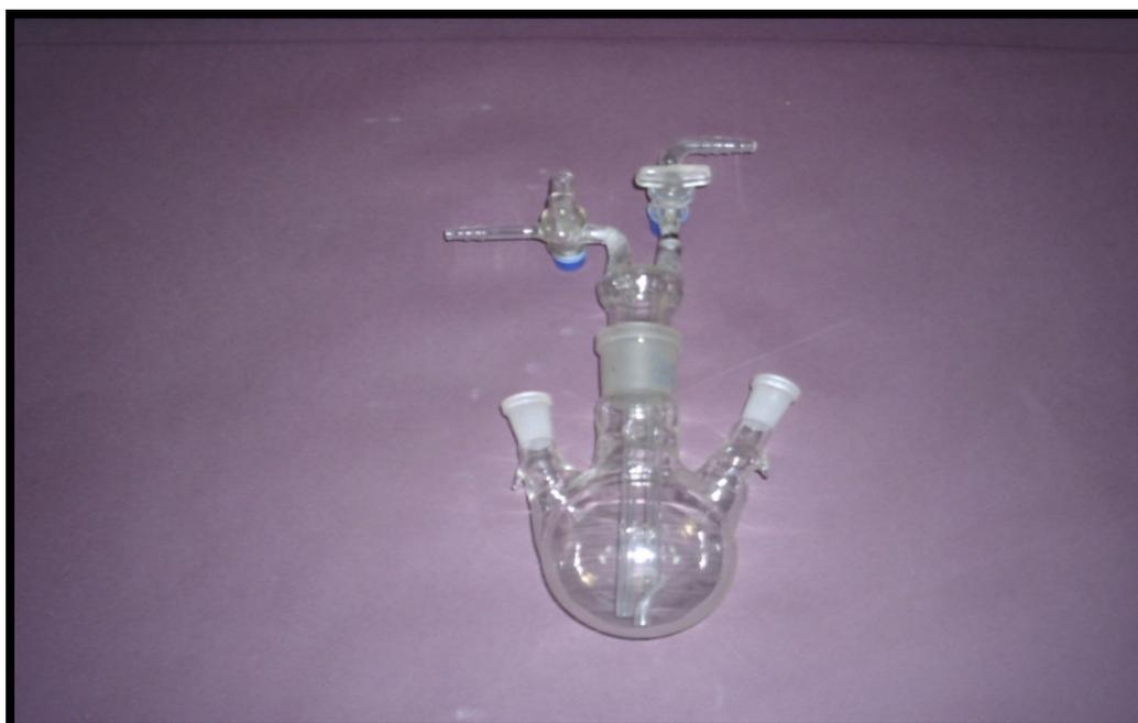
**Fig. 2.5** The Reaction Chamber Used in System 2.
