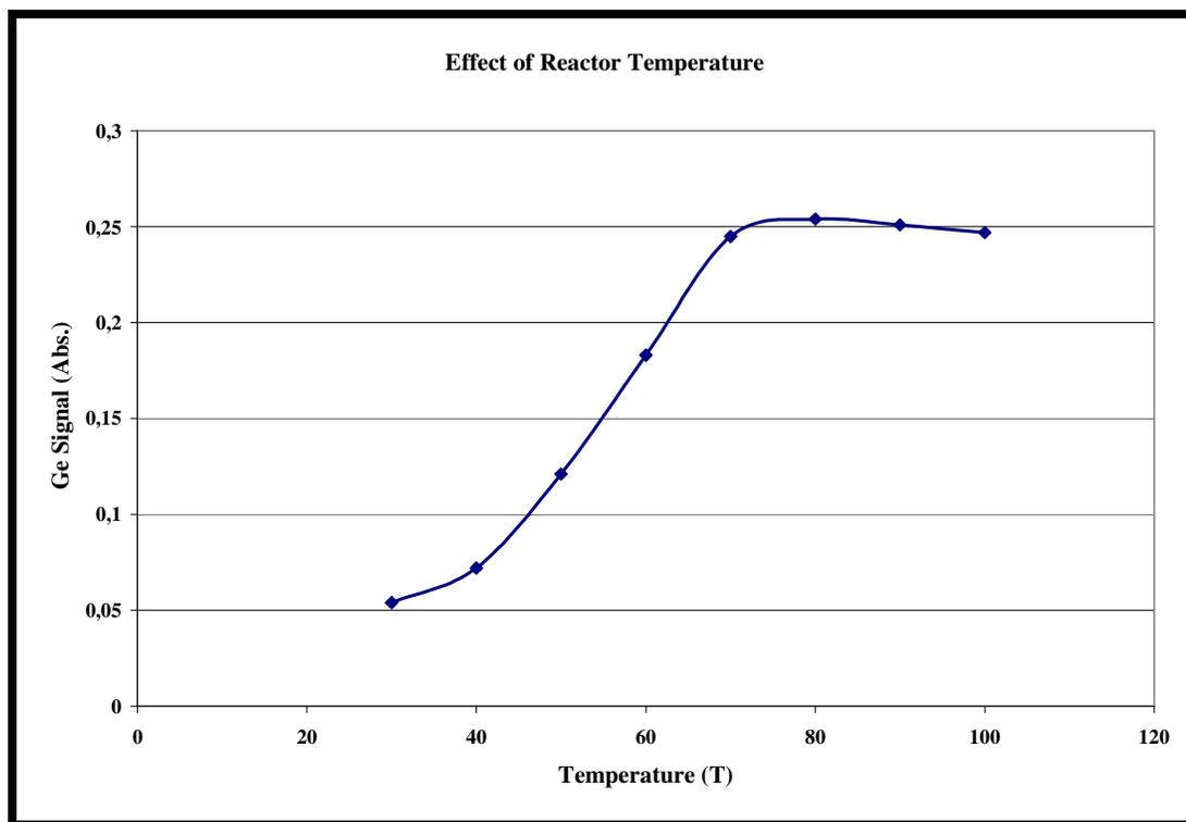
**Fig. 3.4** Effect of Reactor Temperature (Ge 1 $\mu$ g L<sup>-1</sup>, 4 mL)
