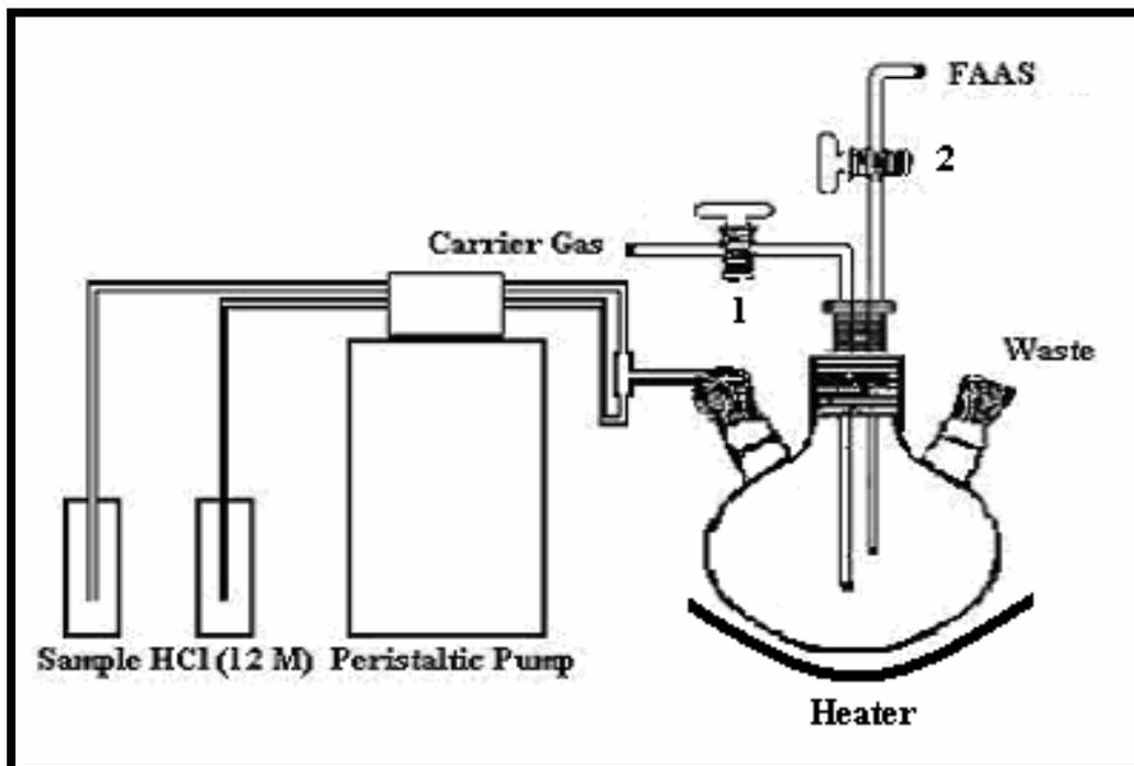
**Fig. 2.4** Schematic Representation of Chloride Generation System 2
