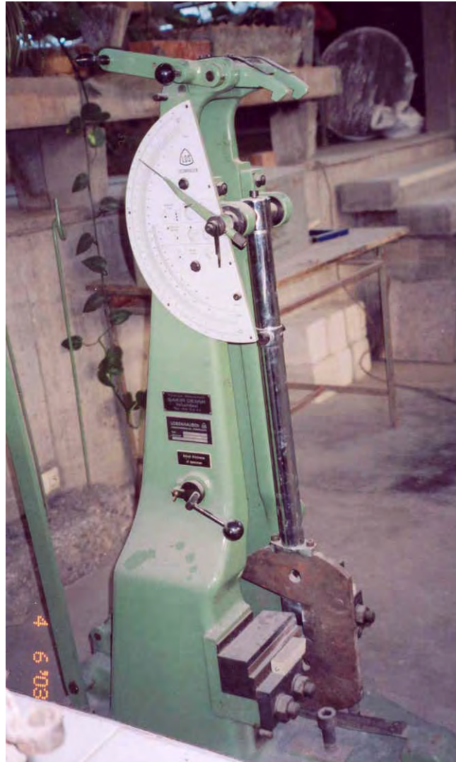
Figure 3.9 Brook’s Model IT 3U Pendulum Impact Tester
