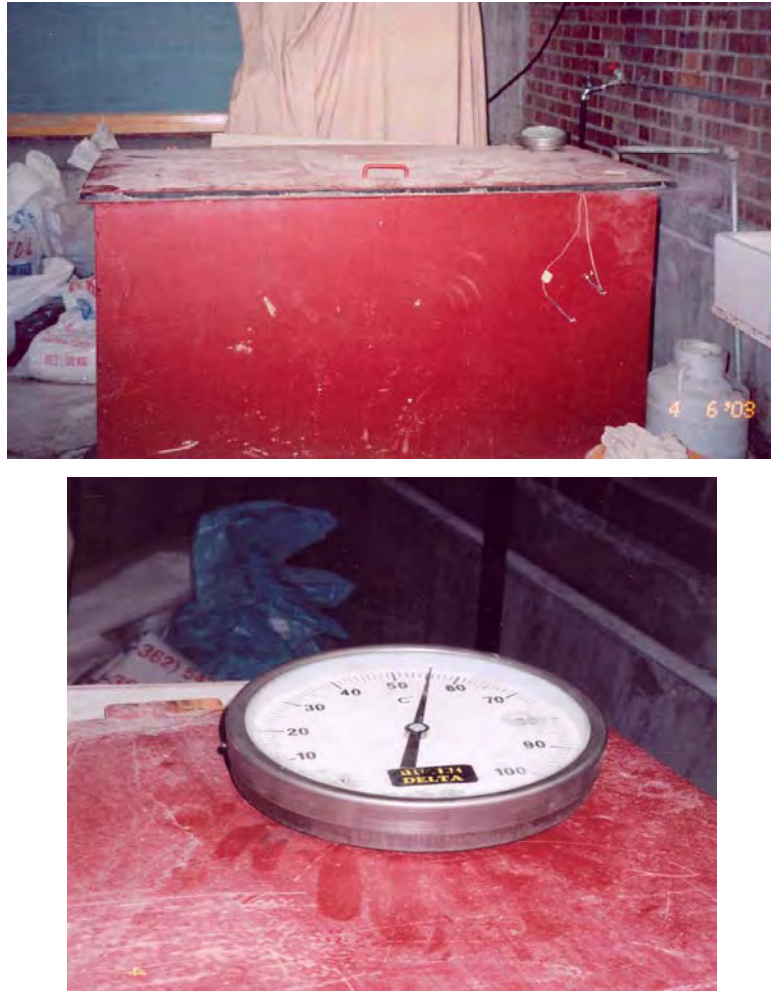
Figure 3.5 Intermittent low pressure steam curing machine at 55°C
