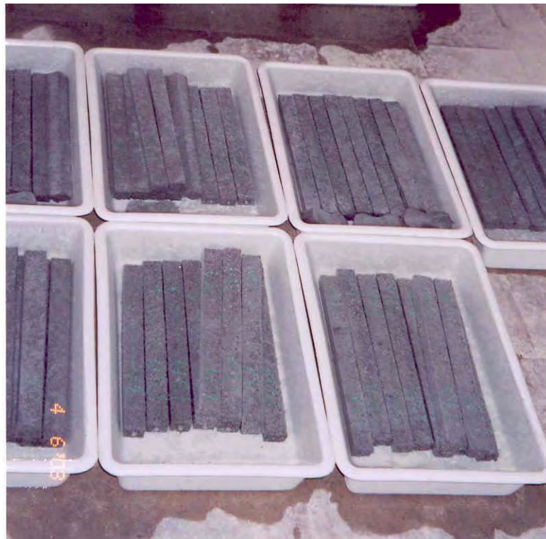
Figure 3.3 The specimens that are immersed in saturated lime water in the curing room
