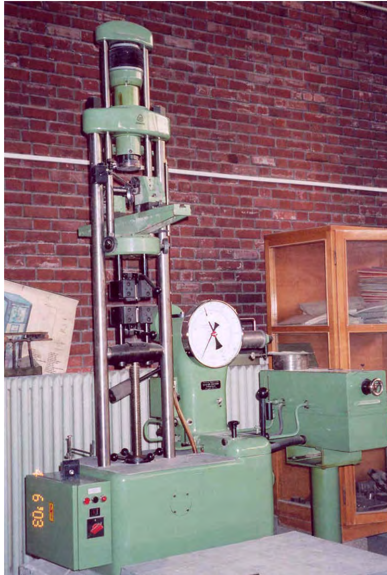
Figure 3.7 The hydraulic Losenhausen model testing machine used in the flexural strength measurement of 25x25x300 mm concrete specimens
