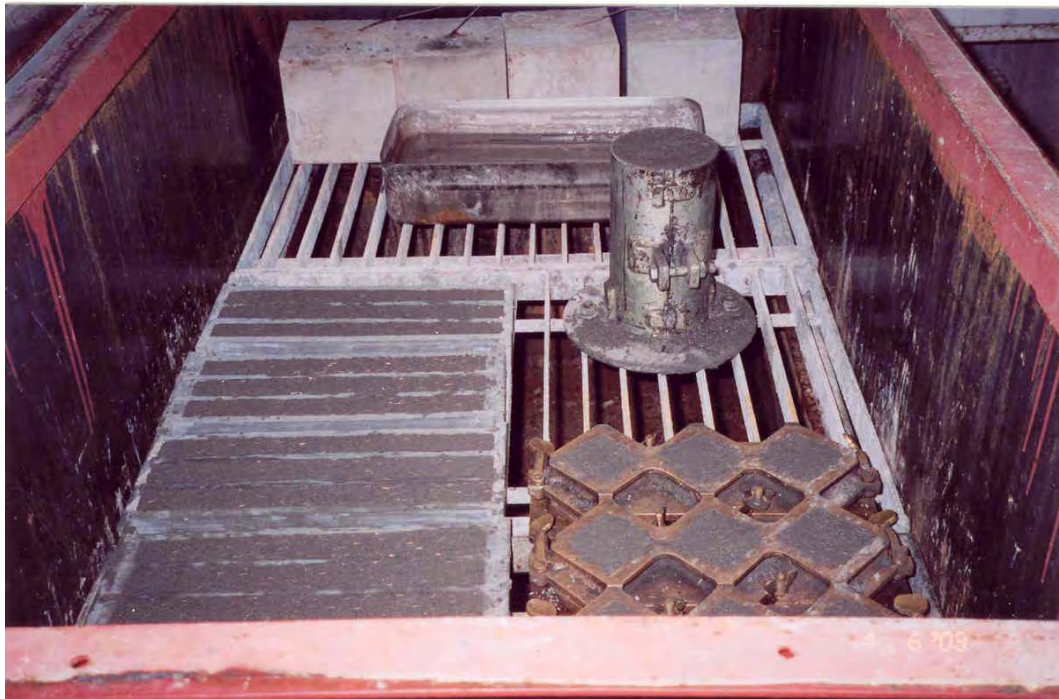
Figure 3.4 The specimens that are placed in the steam chamber after the initial setting
