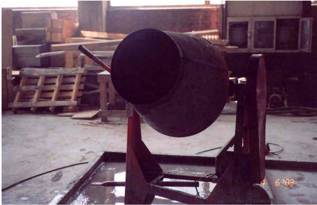
Figure 3.1 The power-driven tilting revolving drum mixer
