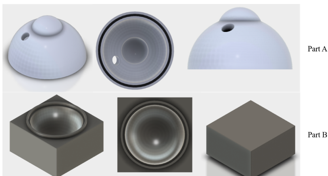
Figure 2.3 Molds of the eye model designed for in vitro extraction experiments, part A (upper part of the figure) features a hole to inject the agarose mixture (similar to the contact lens type thin film mold), two parts of the mold combined via an interlocking mechanism
