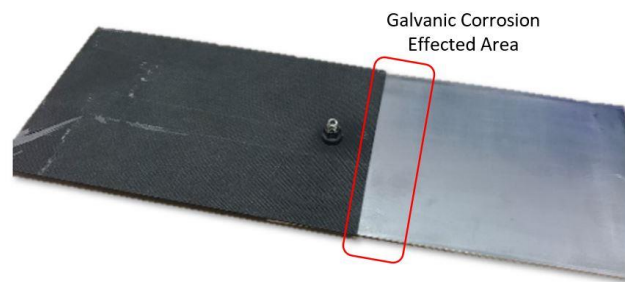
Figure 4.6. The region where the galvanic corrosion effect was examined on the aluminum AA2024-T3.
