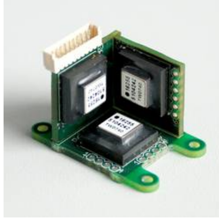
Figure 2.6: Multi Wafer hybrid integration: Rover IMU I taken from [11]
