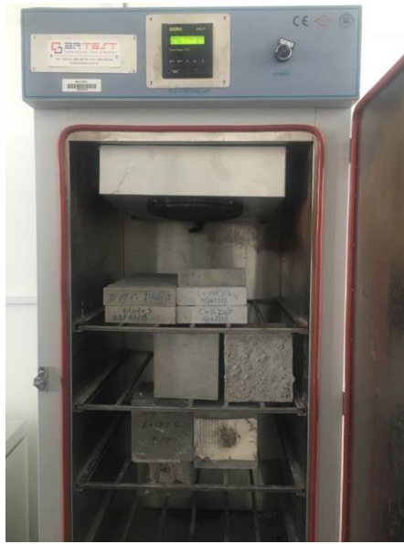
Figure 4.4: Freeze and thaw chamber
