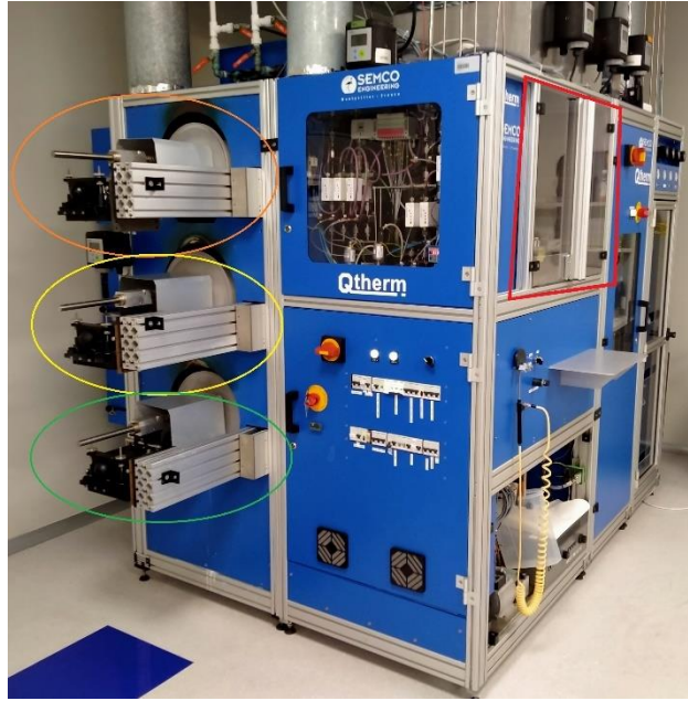
Figure 25 The image of SEMCO furnace with PECVD unit on the right side (red rectangle). On the left side, from top to bottom BCl 3 (orange circle), oxidation (yellow circle) and POCl 3 (green circle) furnaces are shown.
