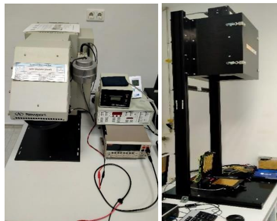
Figure 32 The images of the continuous (left) and flash (right) solar simulators.
