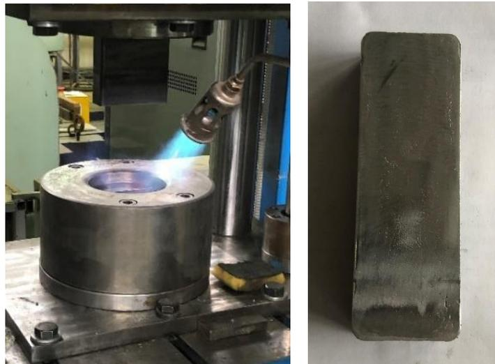
**Figure 4.7.** Preheated die and 90S10B composite after aluminum pressure melt infiltration process
