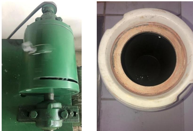
**Figure 4.2.** Ball milling machine and jar filled with ingredients
