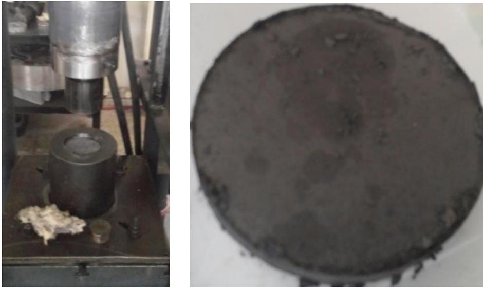
**Figure 4.3.** Pressing operation and green ceramic body
