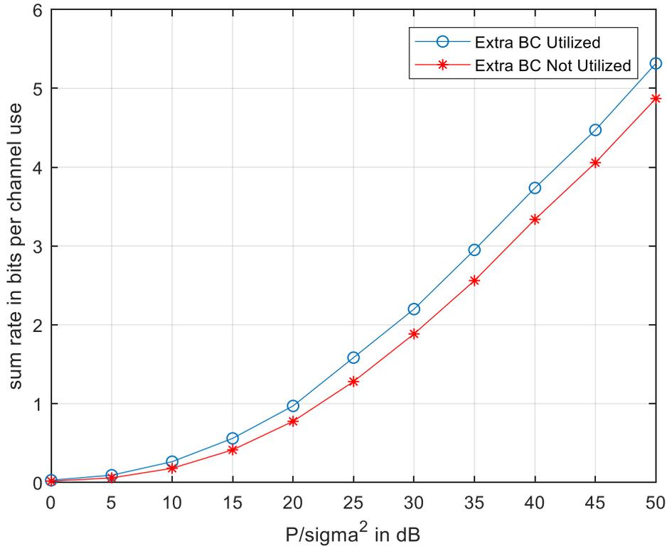
Figure 3.5. Utilizing Extra BC Phases for group with less nodes
