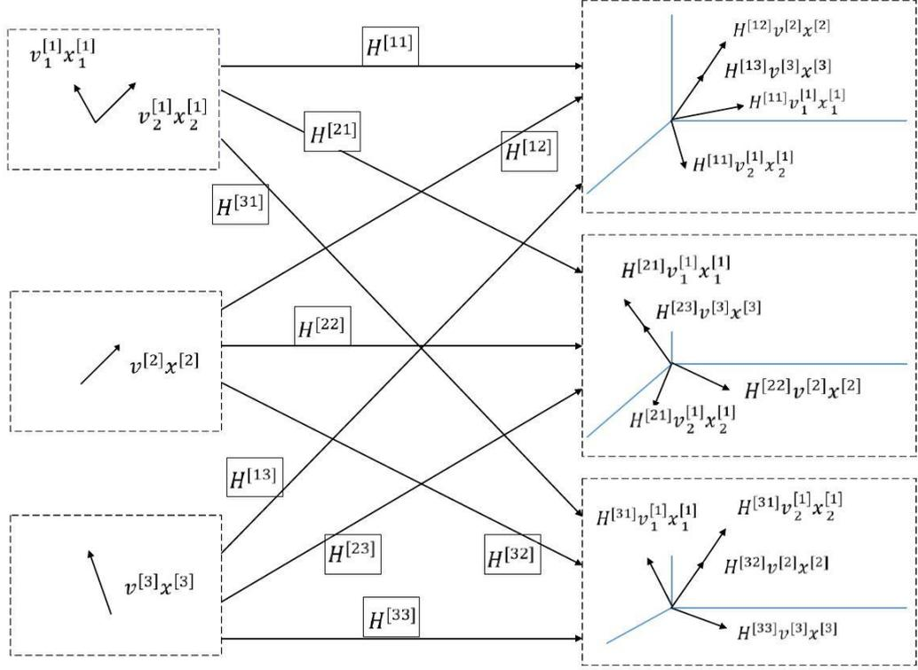
Figure 2.1. Interference Alignment for 3-User Interference Channel
