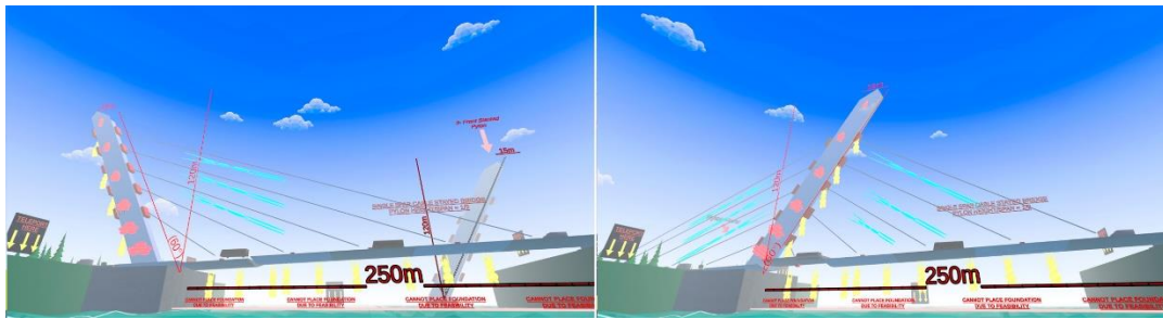
Figure 3.19. Back and front leaning single spar bridges under loading
