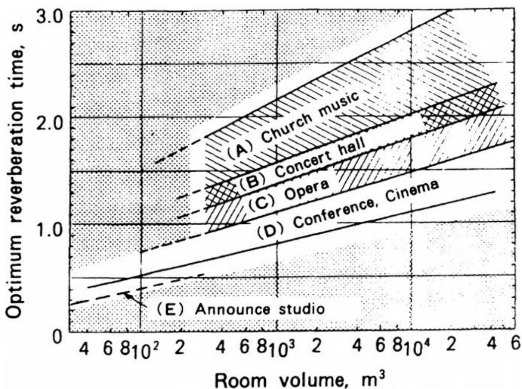
Figure 2.2. Optimum reverberation times at 500 Hz for different types of spaces (Maekawa, 1994)
