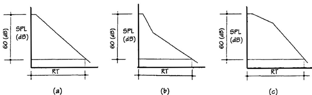
Figure 2.3. Graphs of different sound decays of rooms with equal RT values (Mehta et al, 1999)
