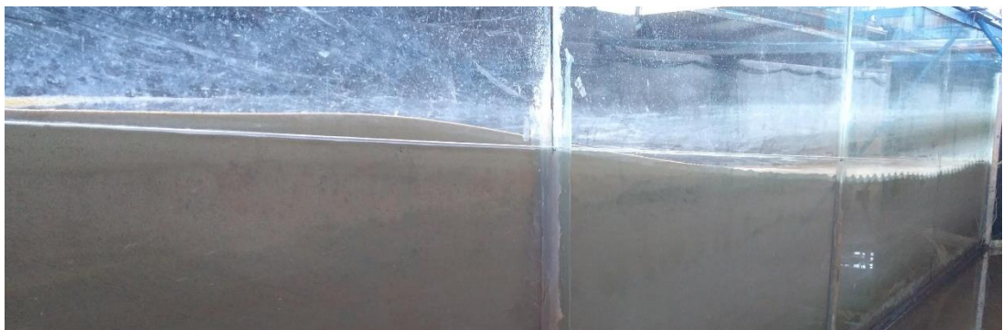
Figure 4.4. Post-Storm Profile of Wave-(ii) ( H_s=2\text{m} and s=0.04 on Prototype Scale)
