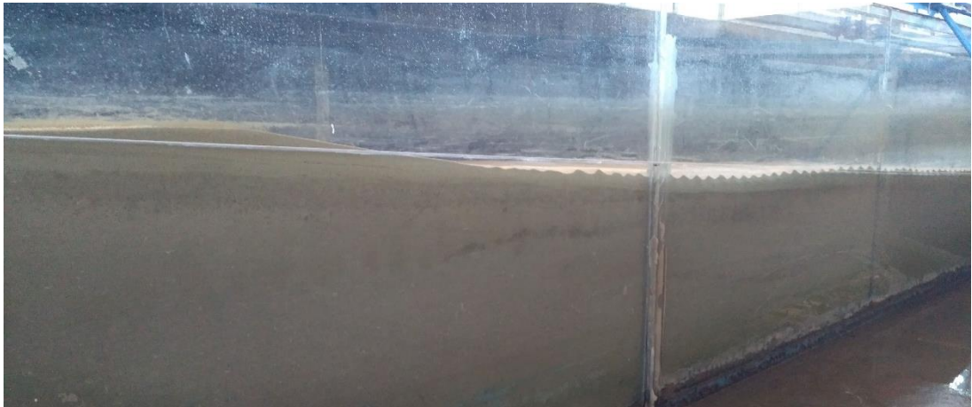
Figure 4.8. Post-Storm Profile of Wave-(iv) ( H_s=1 m and s=0.03 on Prototype Scale)
