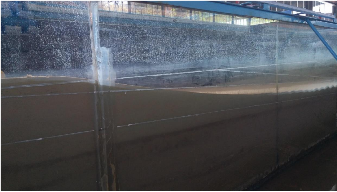
Figure A.14. Post-Storm Bottom Profile of Erosive Waves onto 1:10 Beach Fill
