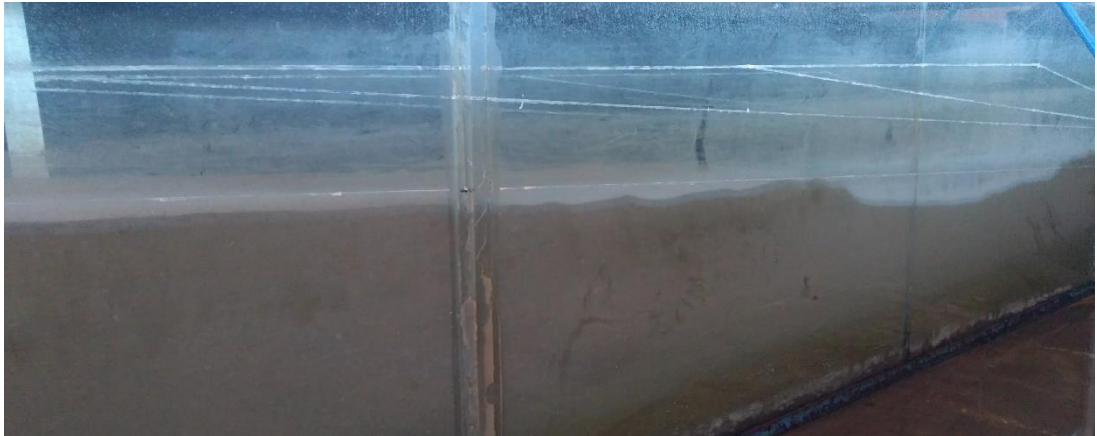
Figure 4.14. Post-Storm Profile of Erosive Waves ( H_s=3\text{m} and s=0.04 on Prototype Scale)
