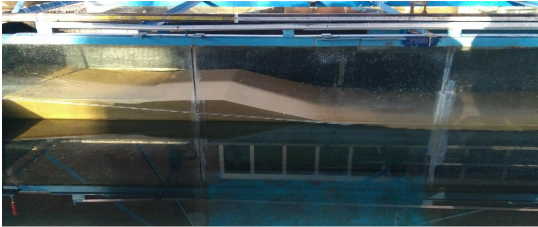
Figure 4.13. Post-Storm Profile of Accretive Waves ( H_s=1\text{m} and s=0.01 on prototype scale)
