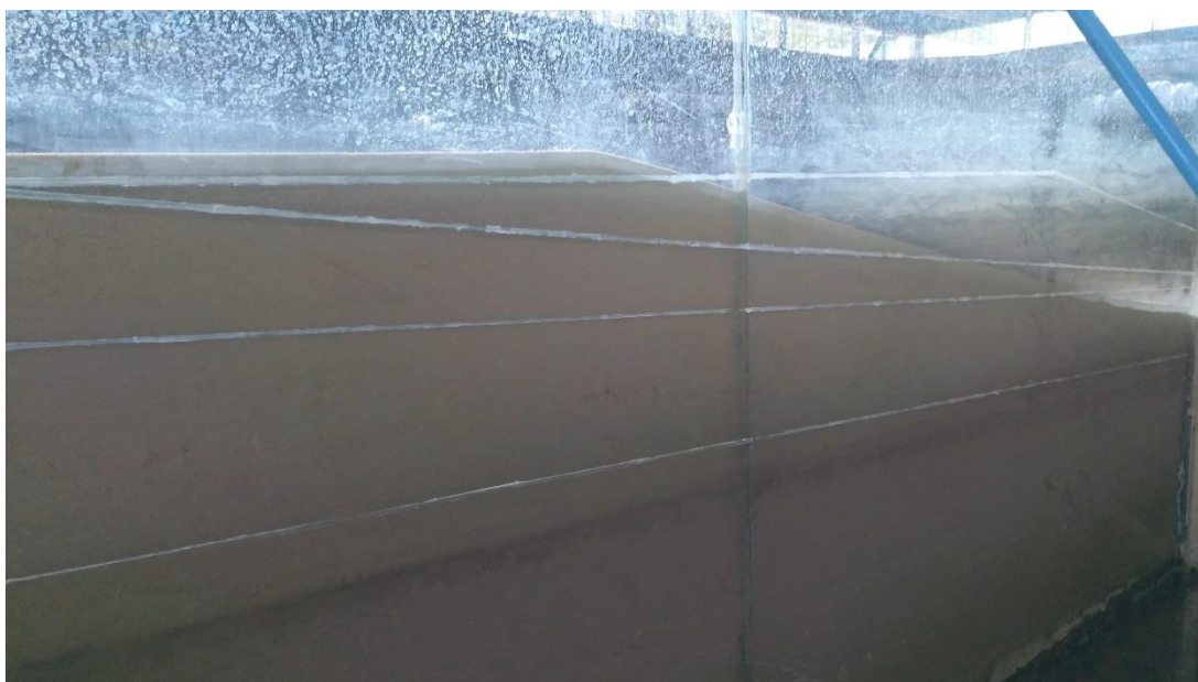
Figure A.12. Post-Storm Bottom Profile of Accretive Waves onto 1:10 Beach Fill
