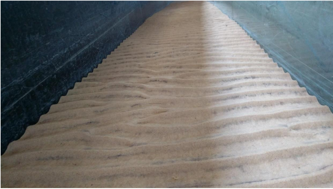
Figure A.3. Ripples Due to Wave-(iv) ( H_s=1\text{m} and s=0.03 )
