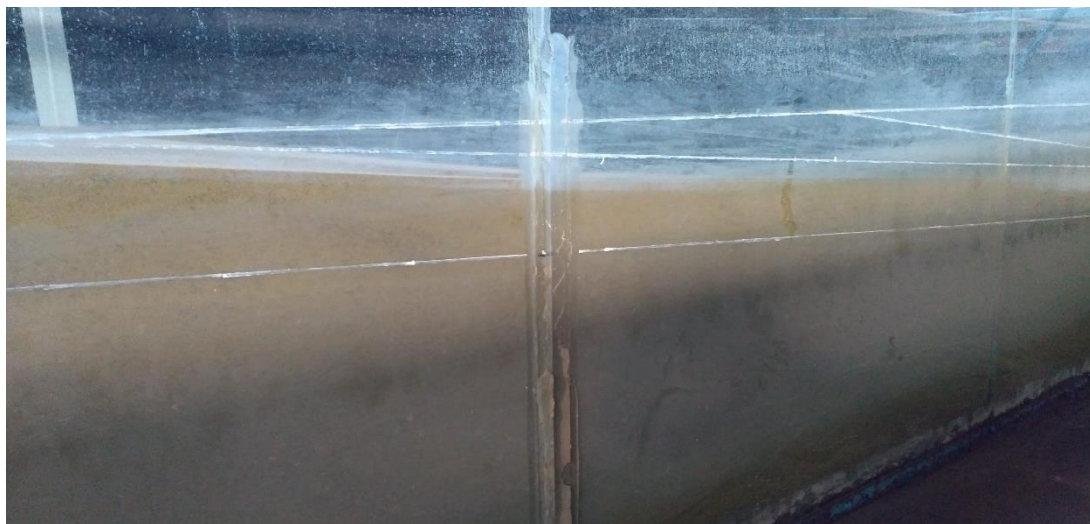
Figure 4.24. Post-Storm Profile of Erosive Waves Impacting on 1:15 Beach Fill
