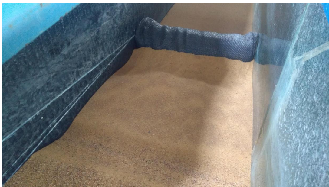
Figure A.24. Post-Storm Bottom Profile around Geotextile Tube After Accretive Waves
