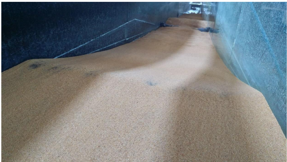
Figure 4.26. Post-Storm Profile of Erosive Waves Impacting on 1:5 Beach Fill
