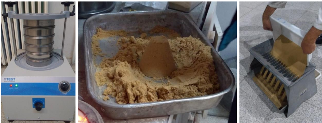
Figure 3.10. Laboratory Tests, Respectively: Sieve Analysis, Moisture Content, Sample Splitting
