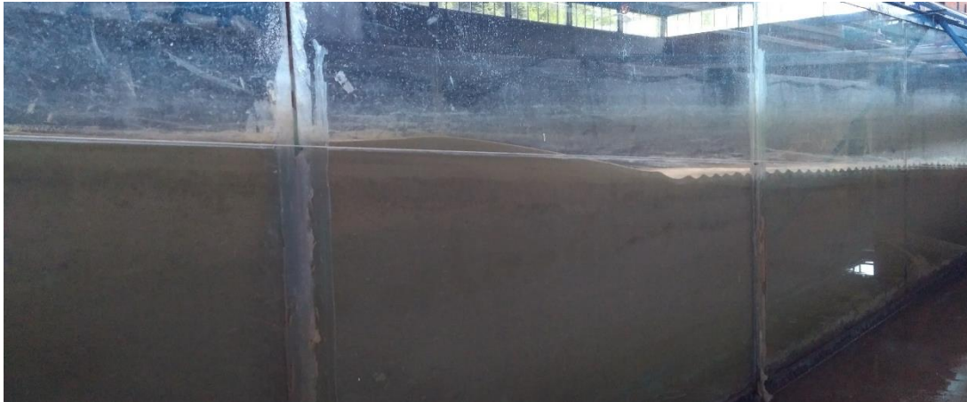
Figure 4.9. Post-Storm Profile of Wave-(v) ( H_s=1\text{m} and s=0.02 on Prototype Scale)
