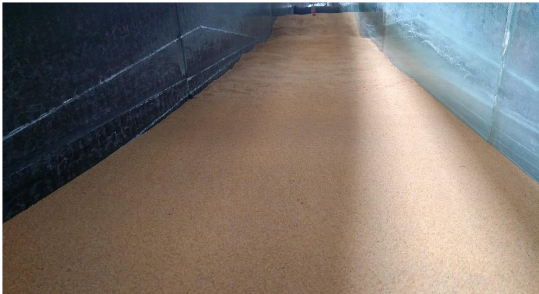
Figure 4.34. Post-Storm Profile of Erosive Waves Impacting on Small Submerged Breakwater
