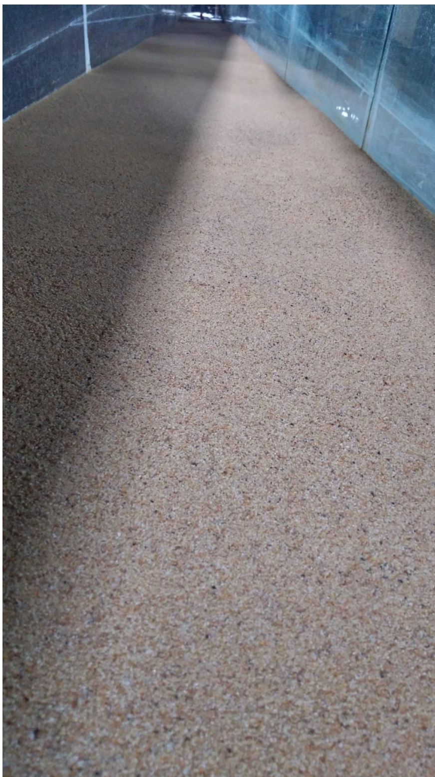
Figure A.20. Natural Beach Slope of 1:15 Consist of Coarse Sand
