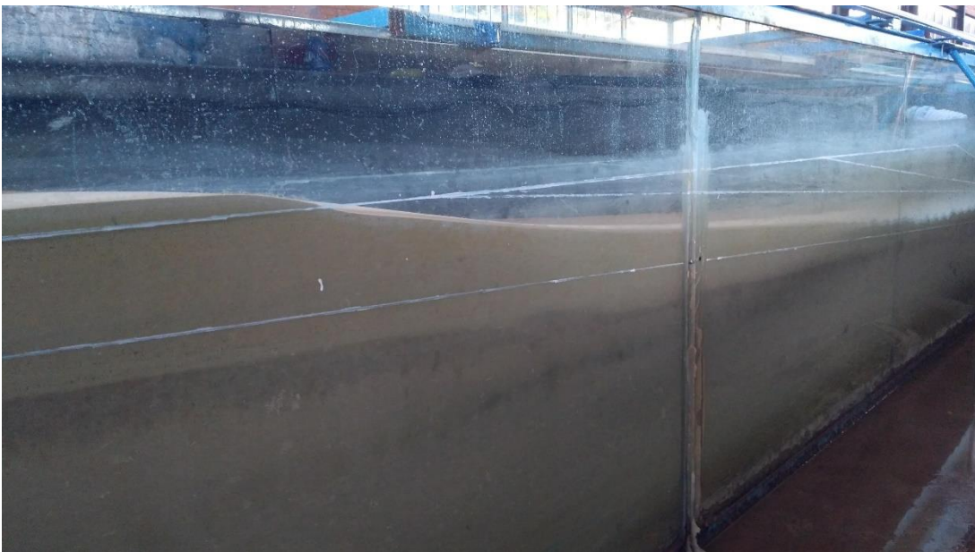
Figure A.8. Post-Storm Bottom Profile of Erosive Waves onto 1:15 Beach Fill
