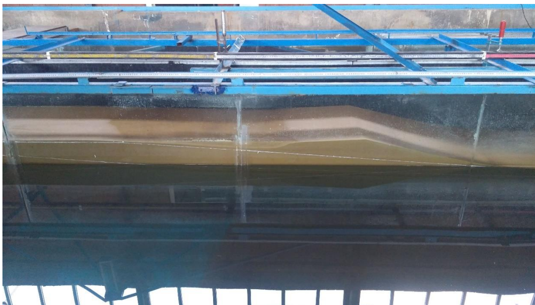
Figure A.6. Post-Storm Bottom Profile of Accretive Waves onto 1:15 Beach Fill
