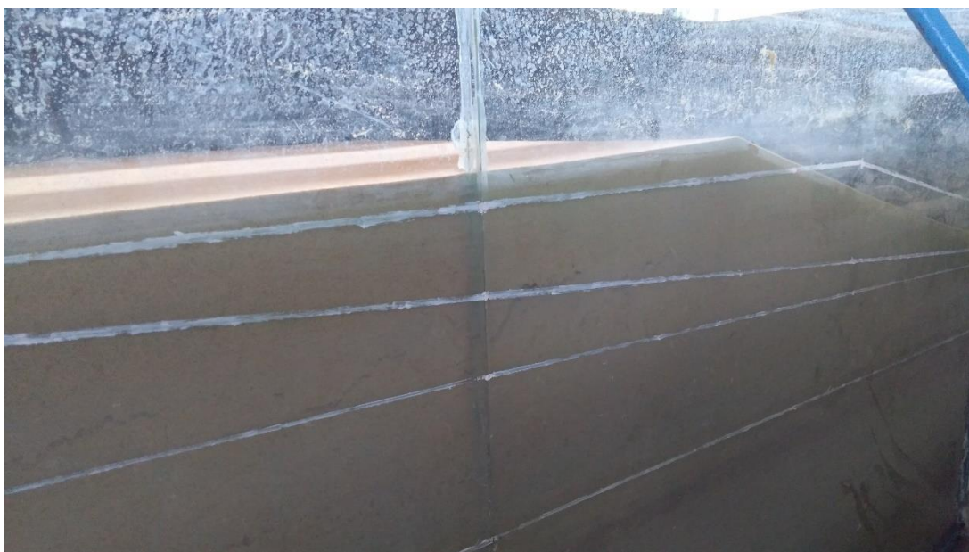
Figure A.16. Post-Storm Bottom Profile of Accretive Waves onto 1:5 Beach Fill
