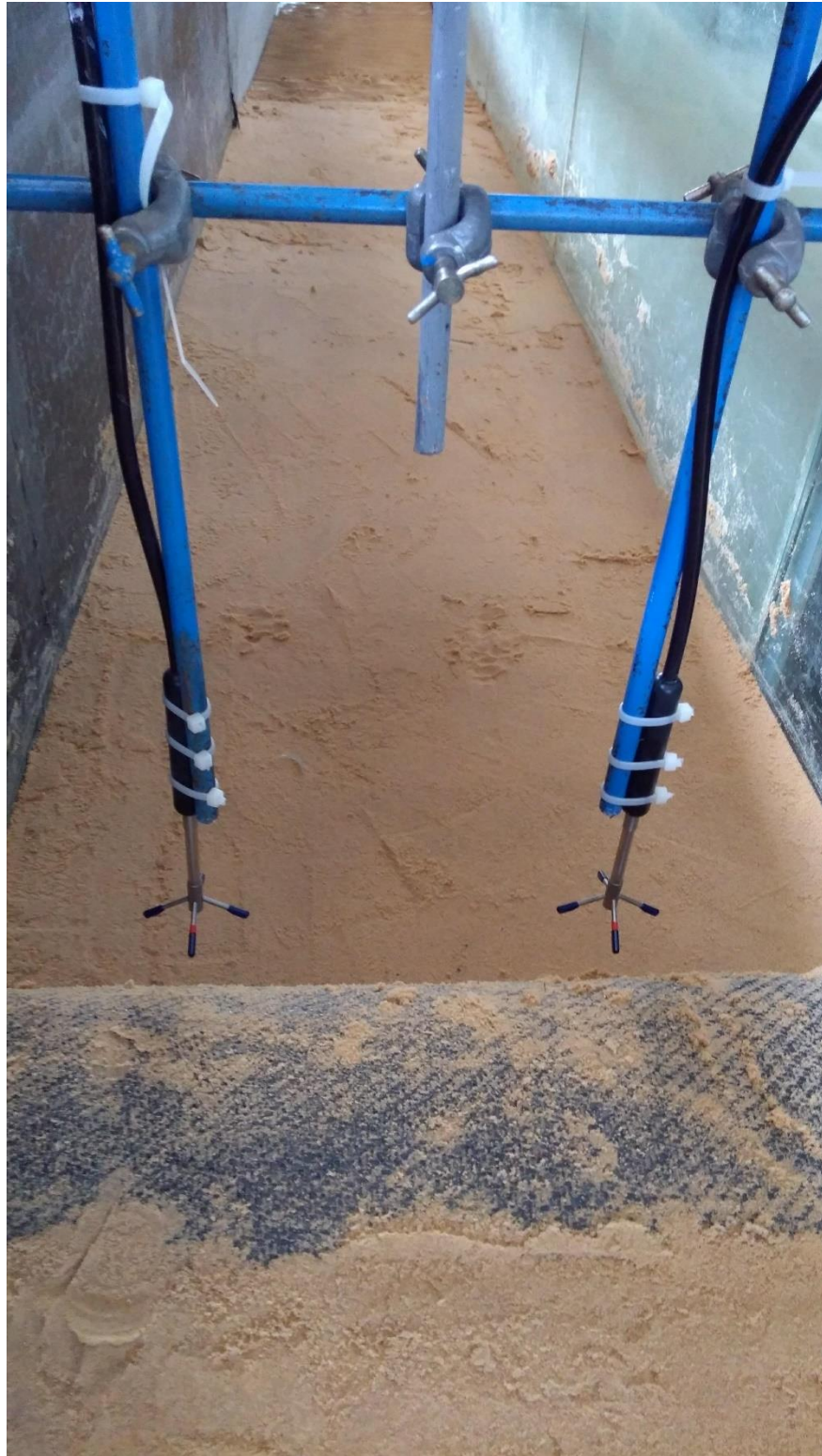
Figure A.19. Acoustic Doppler Velocimetry Setup
