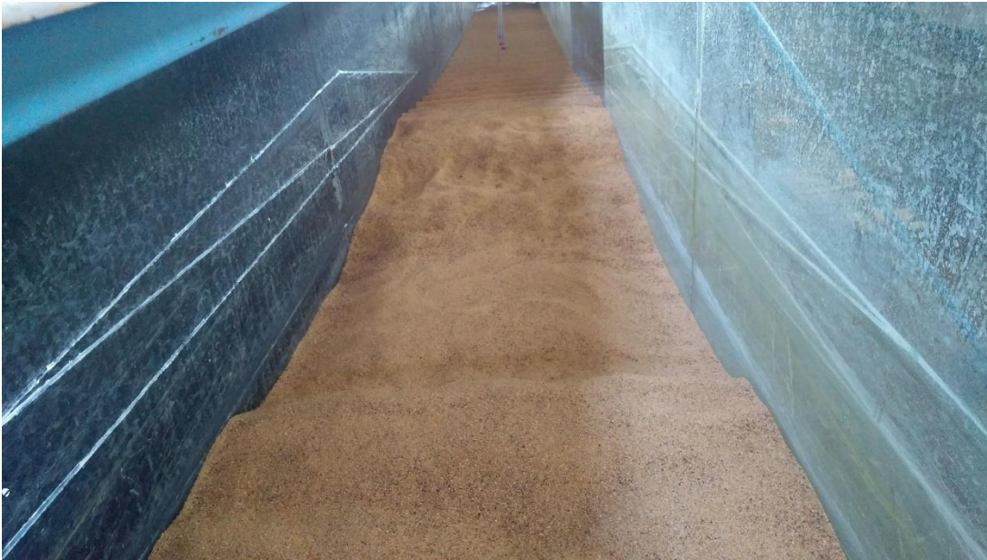
Figure A.22. Sand Bar Formation Due to Erosive Waves
