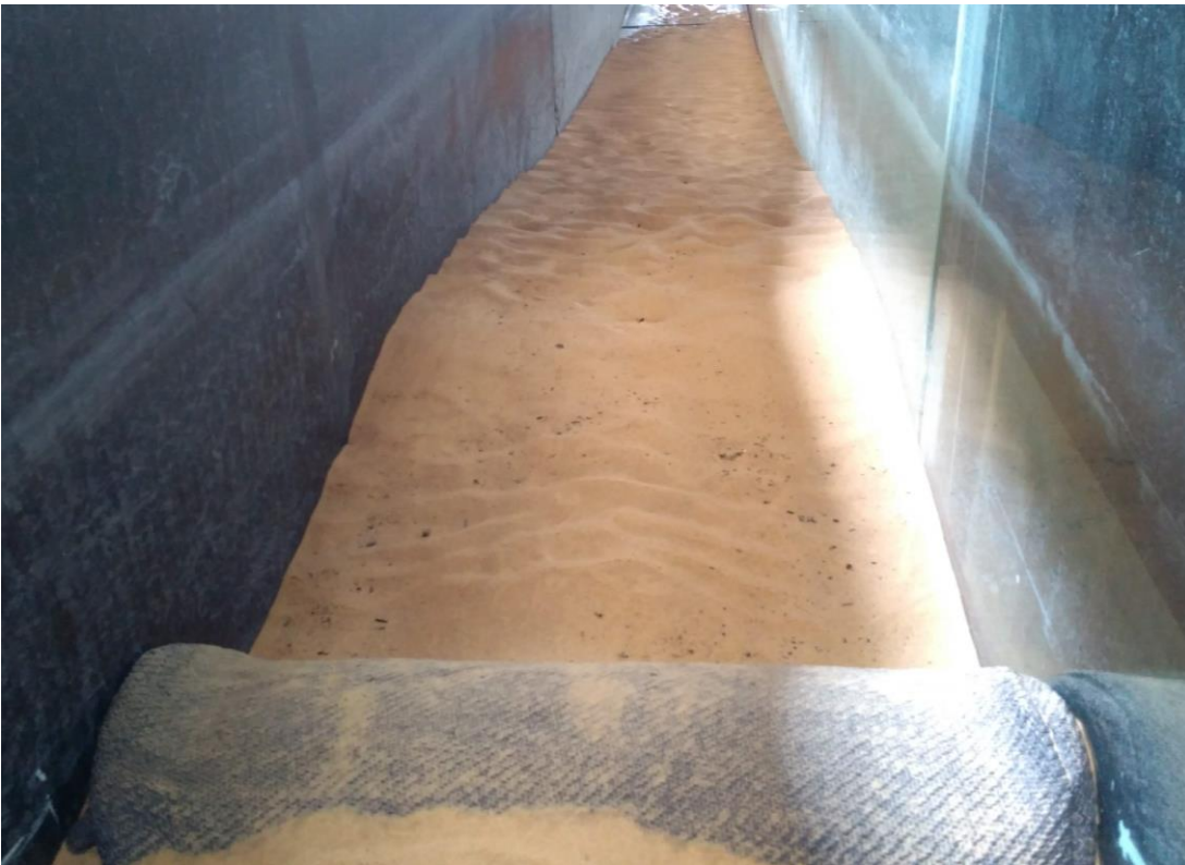
Figure A.15. Sand Bar Formation near Closure Depth under the Influence of Erosive Waves
