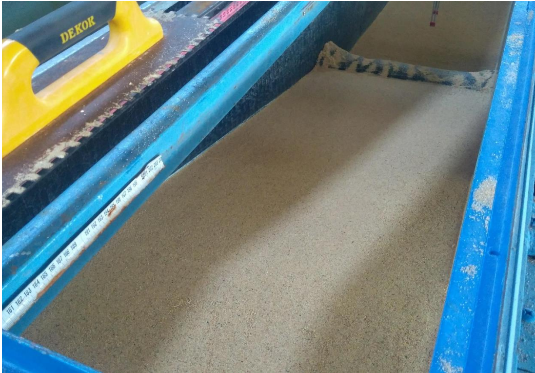
Figure 4.25. Pre-Storm Profile of 1:5 Beach Fill
