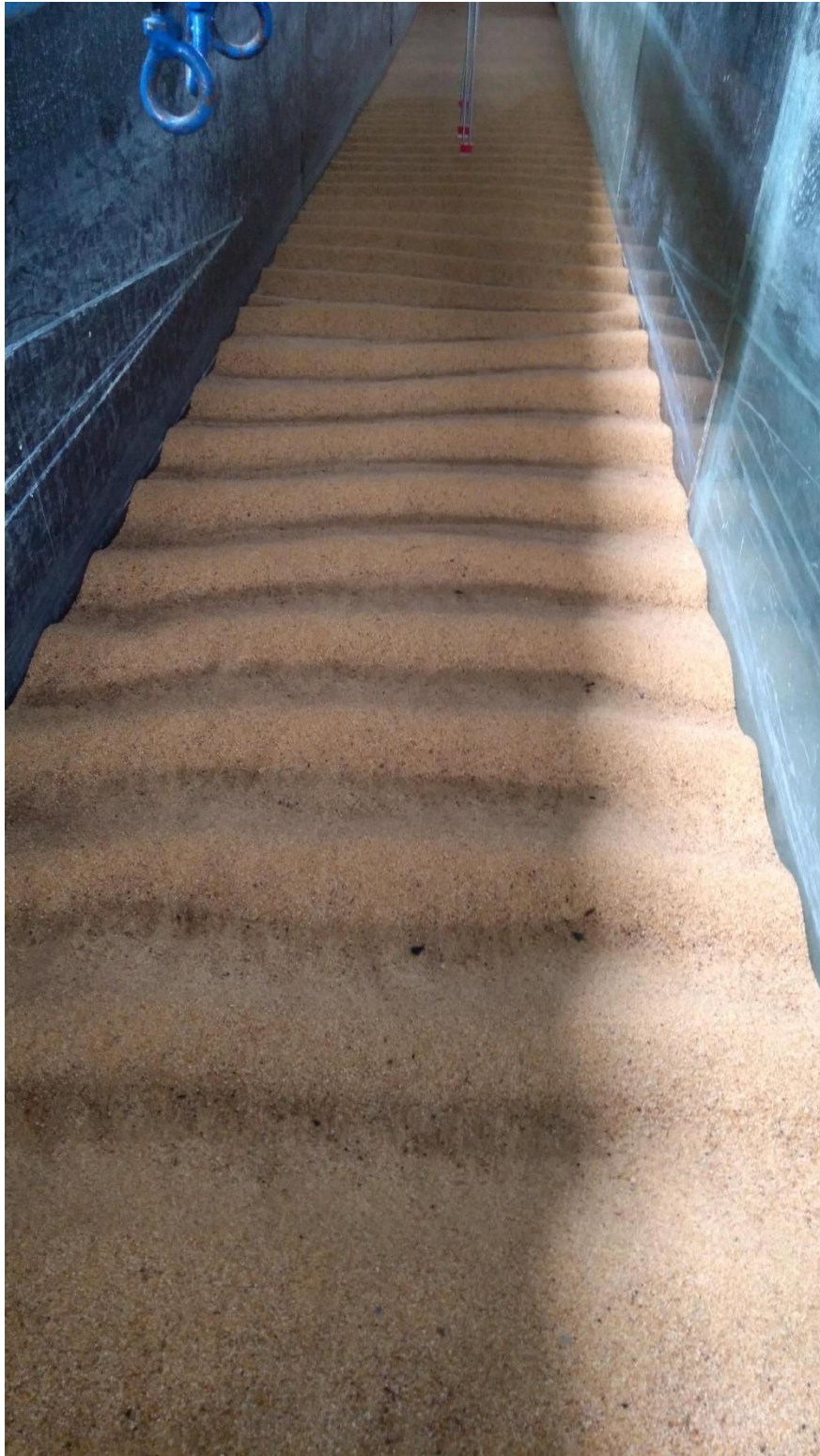
Figure A.21. Ripples Formed onto Coarse Sand Due to Erosive Waves
