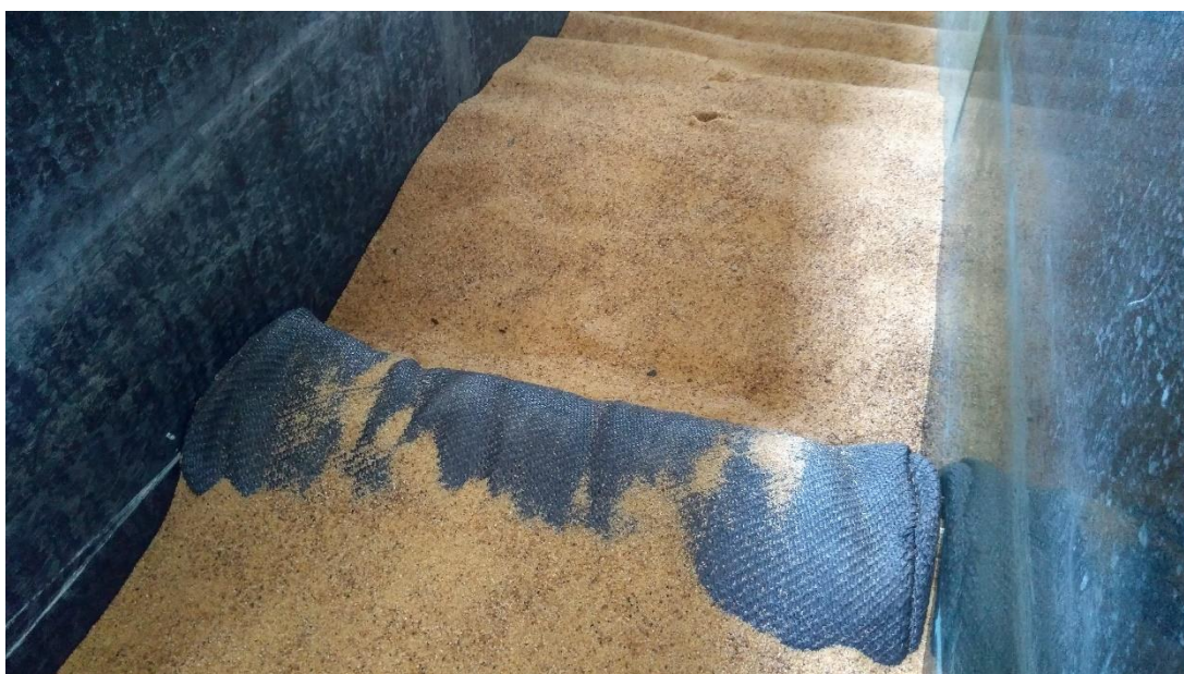
Figure A.25. Post-Storm Bottom Profile around Geotextile Tube After Erosive Waves
