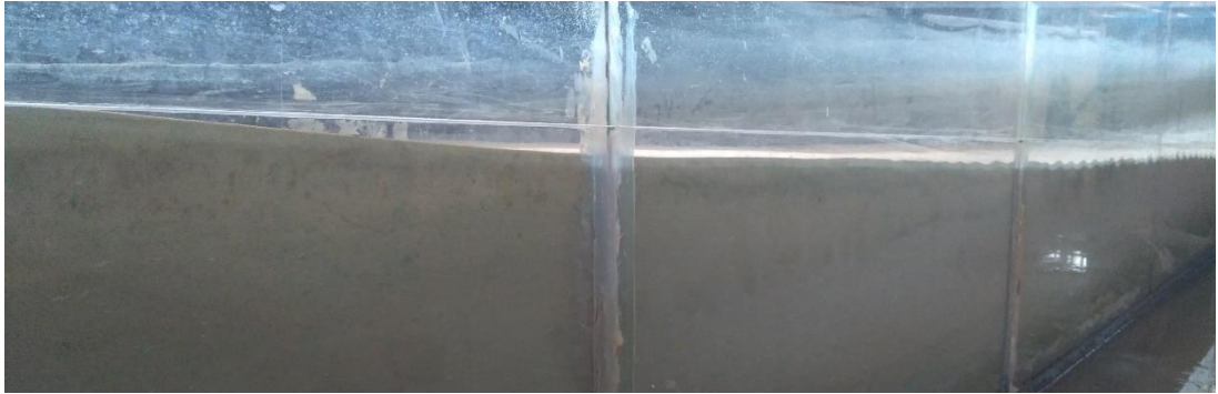
Figure 4.3. Post-Storm Profile of Wave-(i) ( H_s=3\text{m} and s=0.04 on Prototype Scale)
