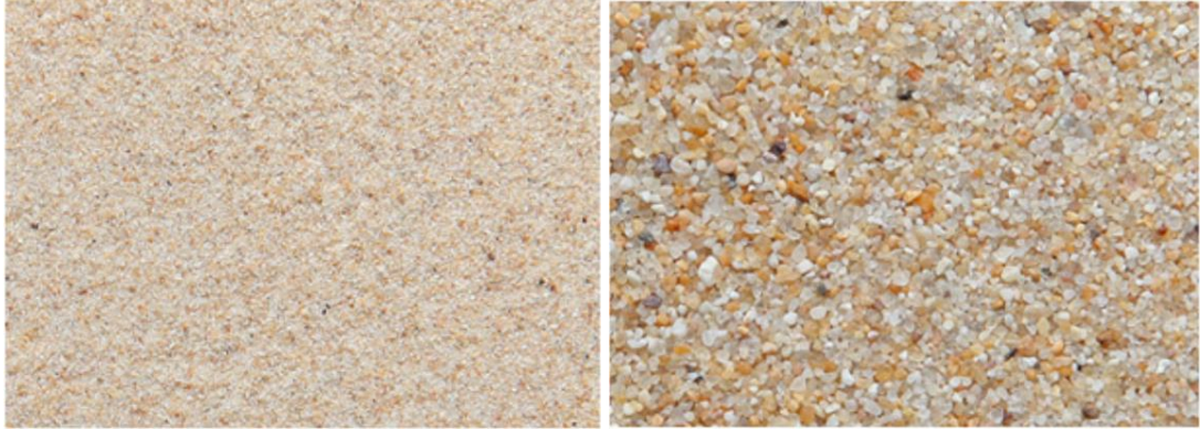
Figure 3.9. AFS 60-70 as Fine Sand (Left) and AFS 20-30 as Coarse Sand (Right)
