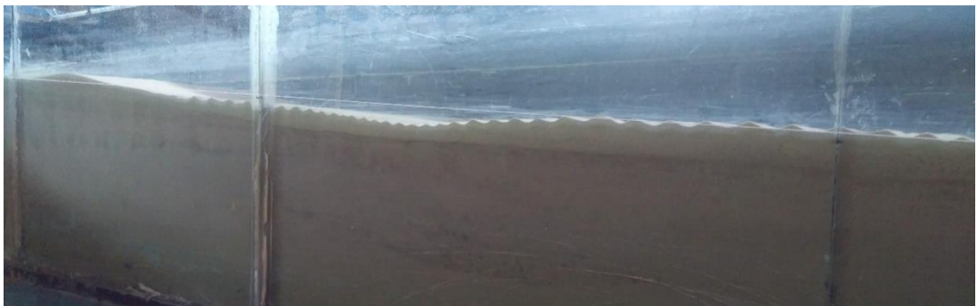
Figure 4.5. Post-Storm Profile of Wave-(iii) ( H_s=1\text{m} and s=0.04 on Prototype Scale)
