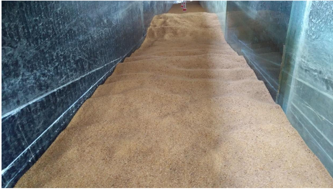
Figure 4.40. Post-Storm Profile of 1:10 Beach Fill without a Toe Structure
