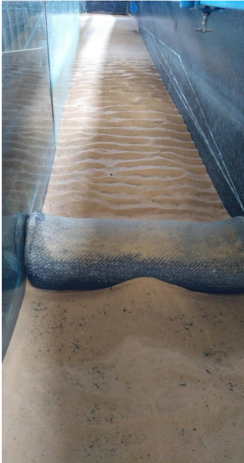
Figure A.11. Post-Storm Bottom Profile of Erosive Waves onto 1:15 Beach Fill
