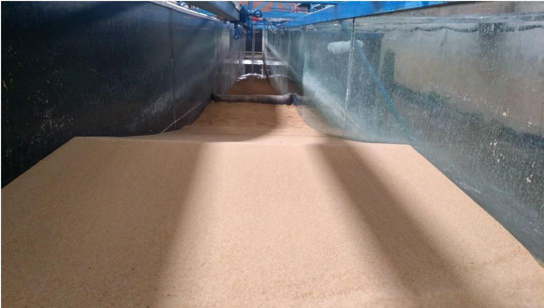
Figure A.7. Sand Berm and Bottom Profile of Summer Waves Acting on 1:15 Beach Fill
