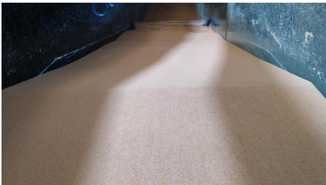
Figure A.17. Sand Berm and Bottom Profile of 1:5 Beach Fill after Accretive Waves
