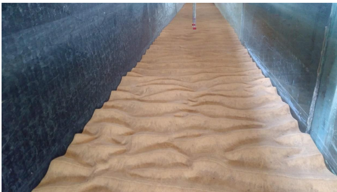
Figure A.5. Ripples Due to Wave-(vi) ( H_s=1\text{m} and s=0.01 )
