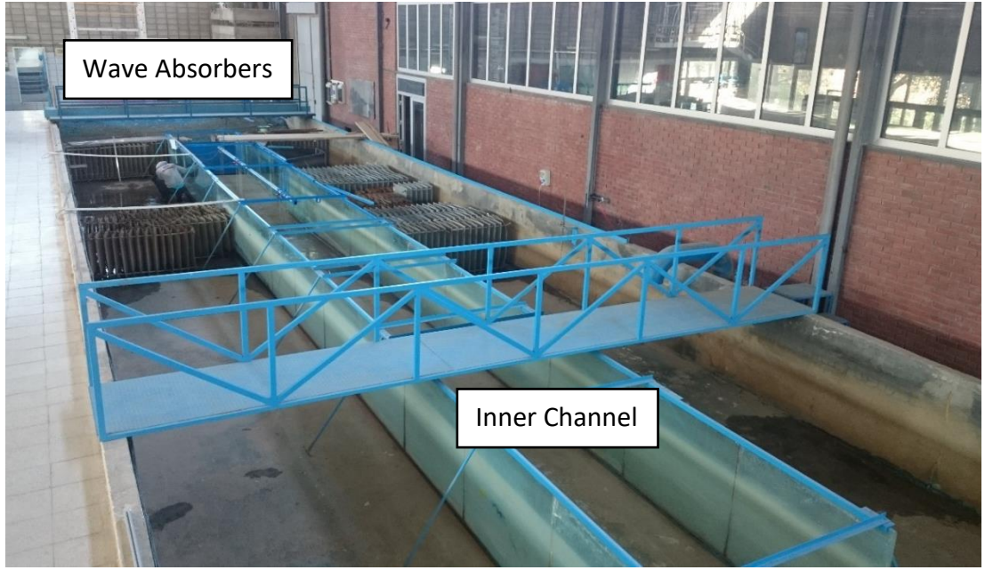
Figure 3.2. Wave Channel at METU Coastal and Ocean Engineering Laboratory
