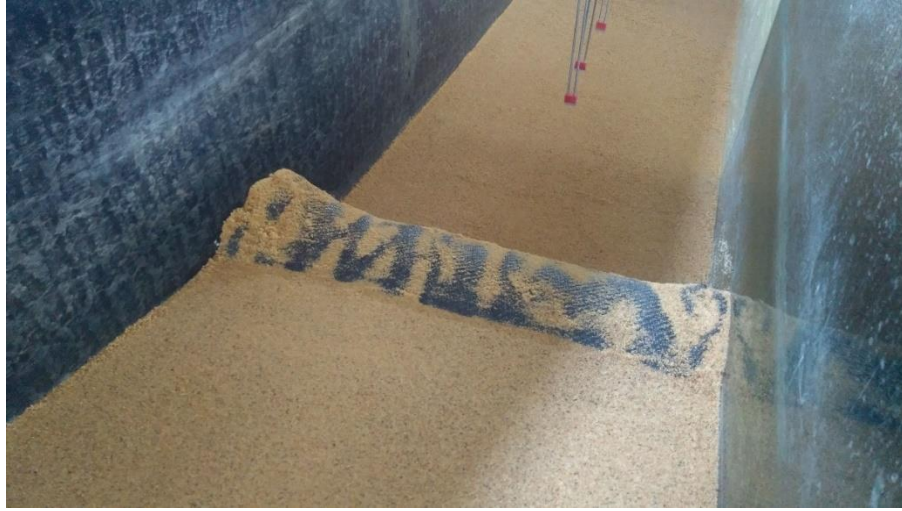
Figure 3.6. Model-Scale Geotextile Tube as Toe Structure of Beach Nourishment
