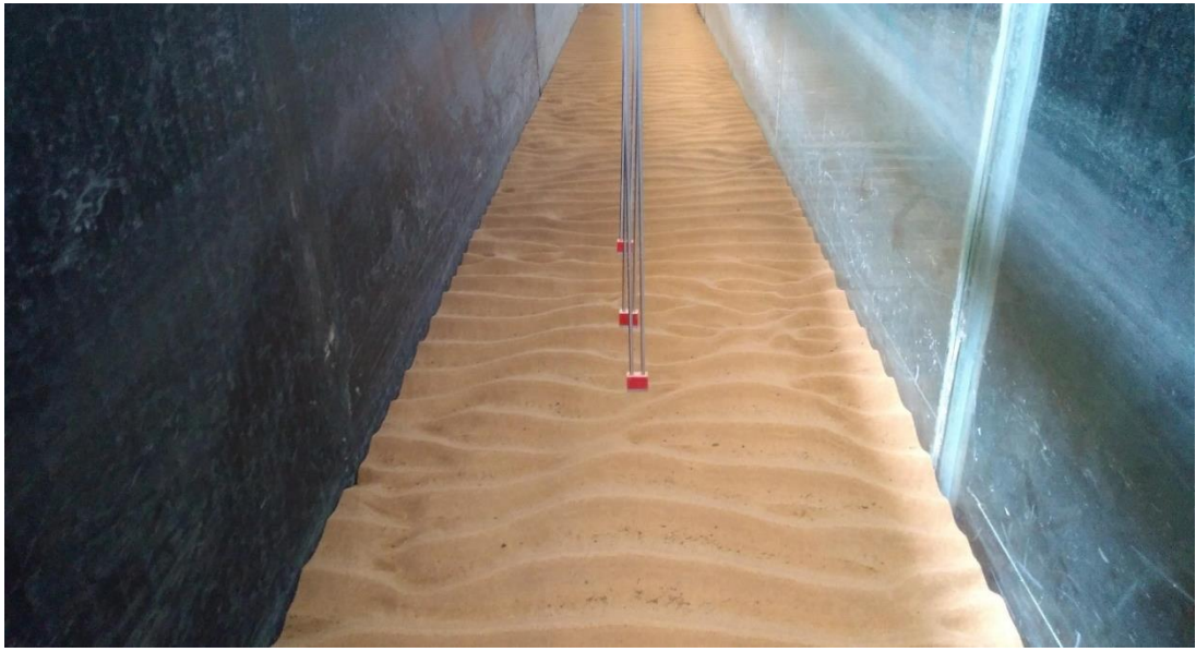
Figure A.1. Ripples Due to Wave-(ii) ( H_s=2\text{m} and s=0.04 )
