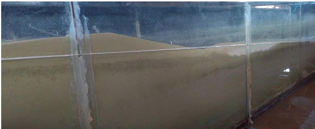
Figure 4.10. Post-Storm Profile of Wave-(vi) ( H_s=1\text{m} and s=0.01 on Prototype Scale)
