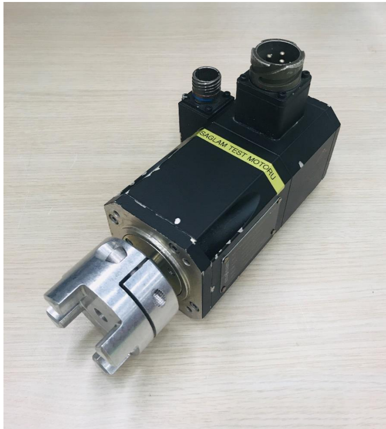
Figure 3.1. The Test Motor (400W PMSM)
