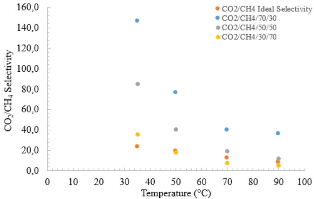
Figure 4.13 CO<sub>2</sub>/CH<sub>4</sub> selectivity versus temperature graph of M1 membrane with different feed gas compositions
