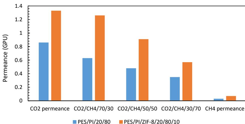
Figure 4.20 Filler material (ZIF-8) effect on permeances of PES/PI/20/80 blend and PES/PI/ZIF-8/20/80/10 mixed matrix membranes (IR time: 80 sec.)
