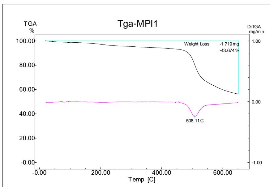
Figure F.2 Thermogram of M-PI1-P1
