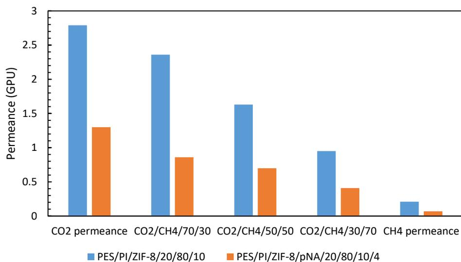
Figure 4.22 Compatibilizer (pNA) effect on permeances of PES/PI/ZIF-8/20/80/10 mixed matrix and PES/PI/ZIF-8/pNA/20/80/10/4 membranes (IR time: 40 sec.)
