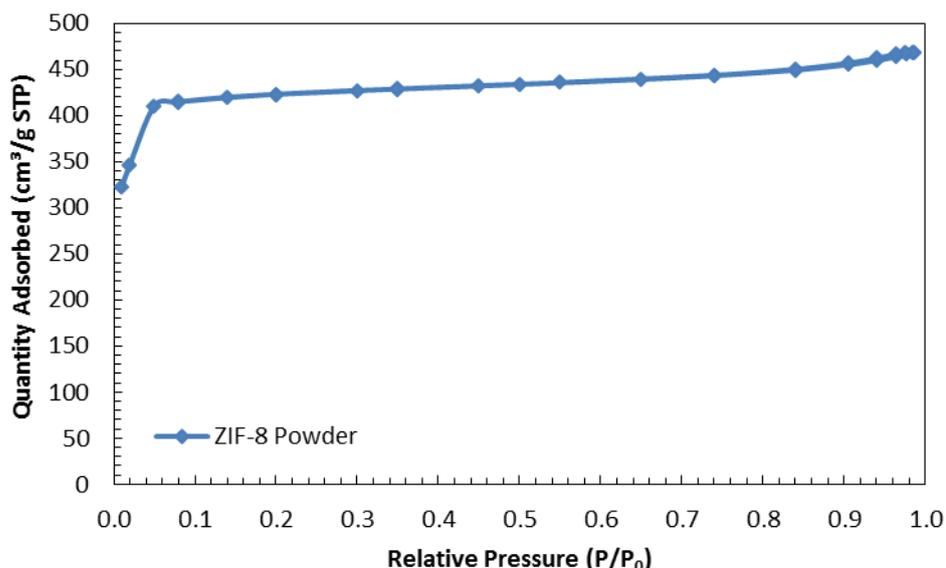
Figure 4.3 Nitrogen adsorption isotherm of ZIF-8 powder at 77 K
