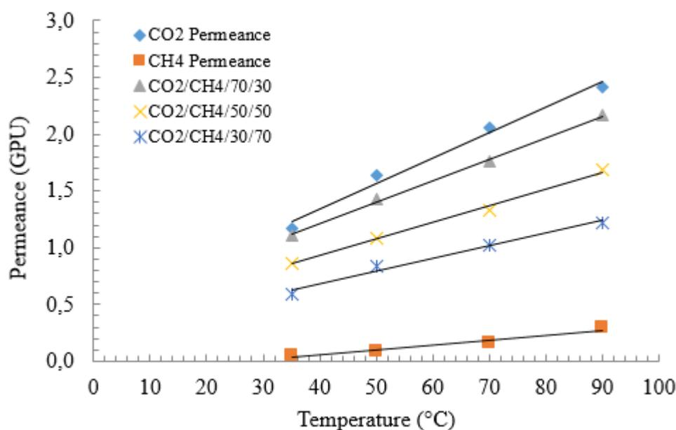
Figure 4.12 Permeance versus temperature graph of M1 membrane with different feed gas compositions
