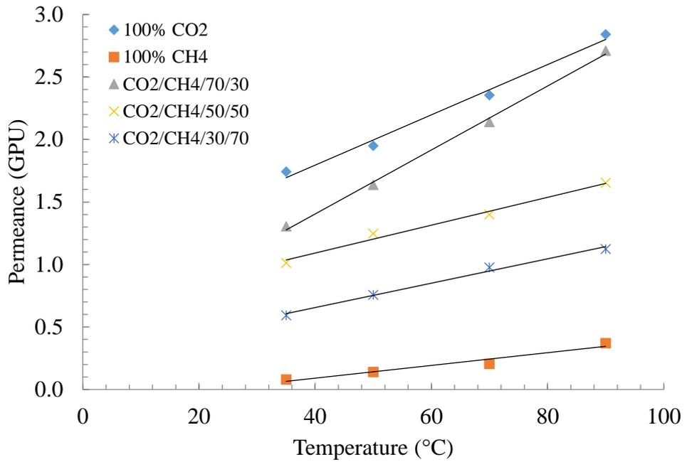
Figure 4.28 Permeance versus temperature graph of M8 membrane with different feed gas compositions
