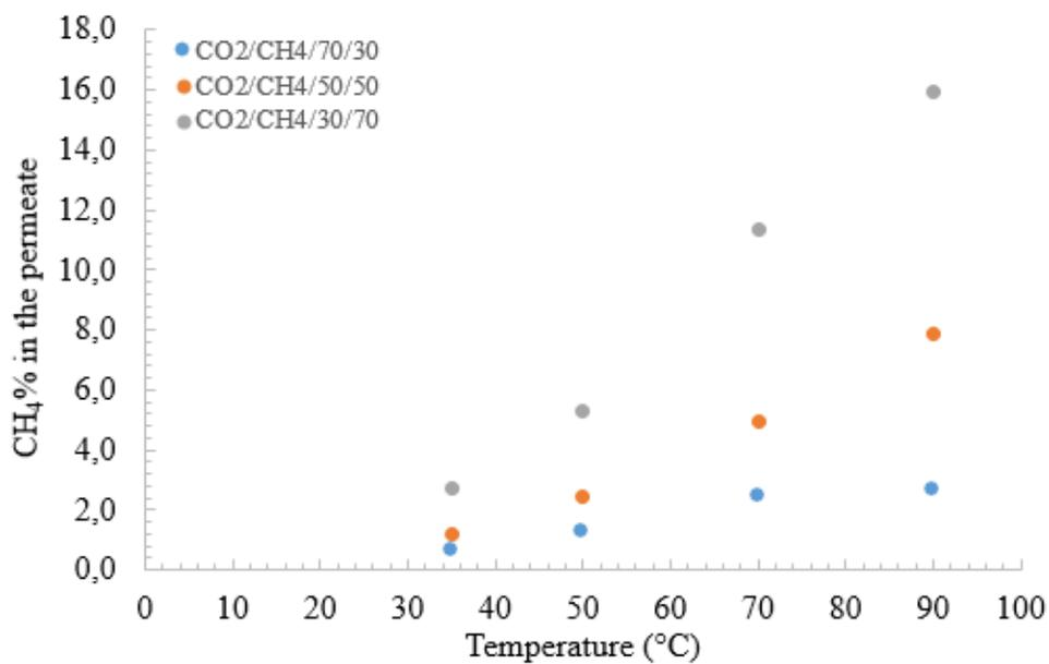
Figure 4.15 CH<sub>4</sub>% in the permeate vs temperature graph of M1 membrane for different feed gas compositions
