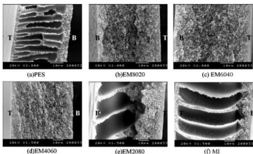
Figure 2.7 The SEM images of membrane cross-sections for different blend compositions by using DMF [17]
