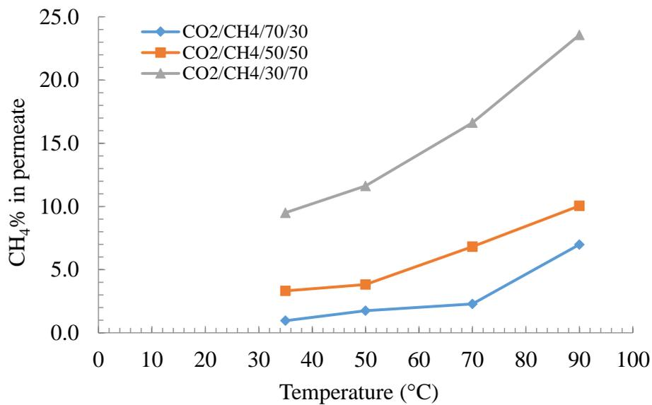
Figure 4.27 CH<sub>4</sub>% in the permeate vs temperature graph of M7 membrane for different feed gas compositions
