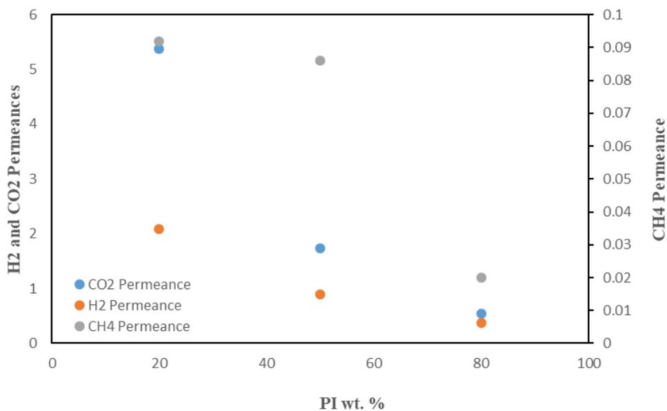
Figure 4.9 H<sub>2</sub>,CO<sub>2</sub> and CH<sub>4</sub> permeances vs PI wt.% graph for the produced blend membrane with 120 sec. IR lamb
