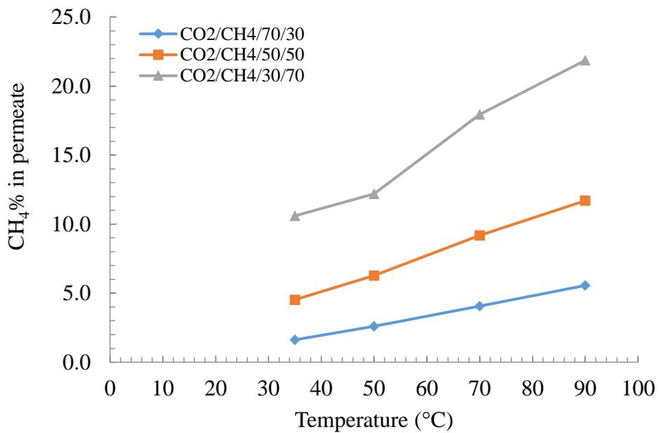
Figure 4.31 CH<sub>4</sub>% in the permeate vs temperature graph of M8 membrane for different feed gas compositions
