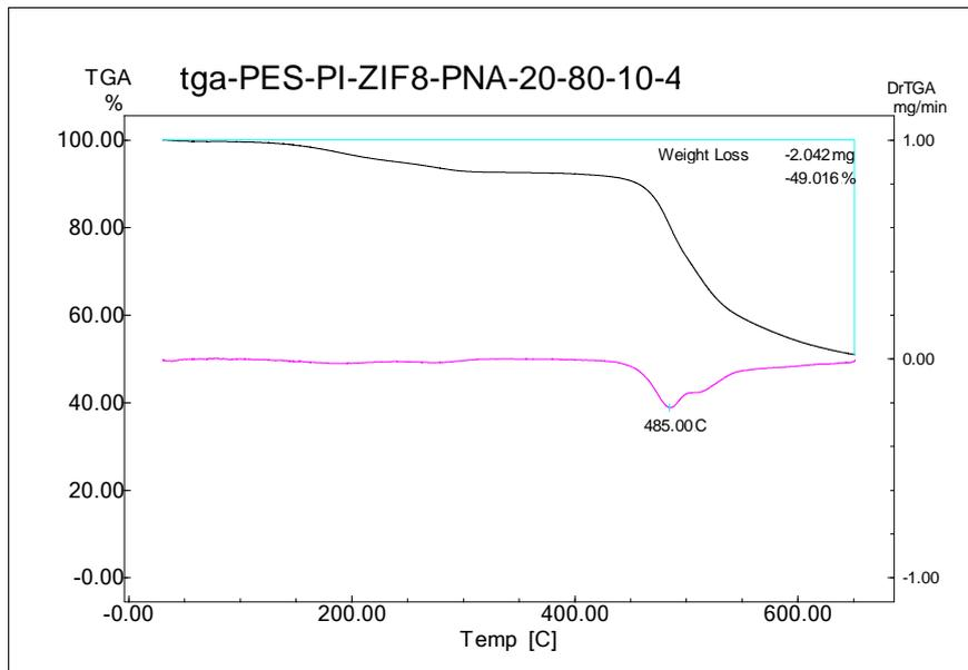
Figure F.7 Thermogram of PES/PI/ZIF8/pNA/20/80/10/4
