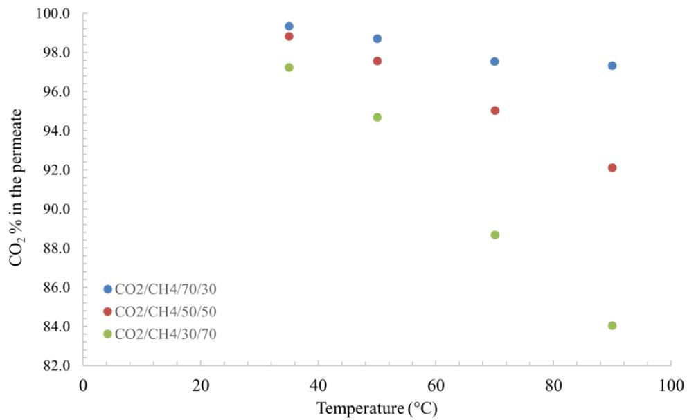
Figure 4.14 CO<sub>2</sub>% in the permeate vs. temperature graph of M1 membrane for different feed gas compositions
