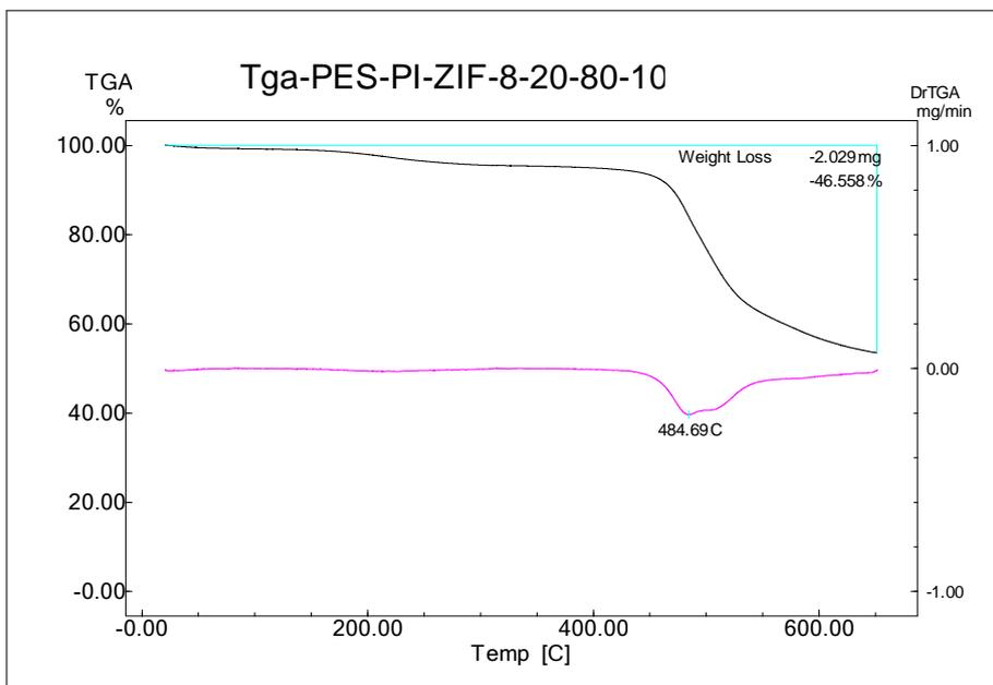
Figure F.6 Thermogram of PES/PI/ZIF-8/20/80/10
