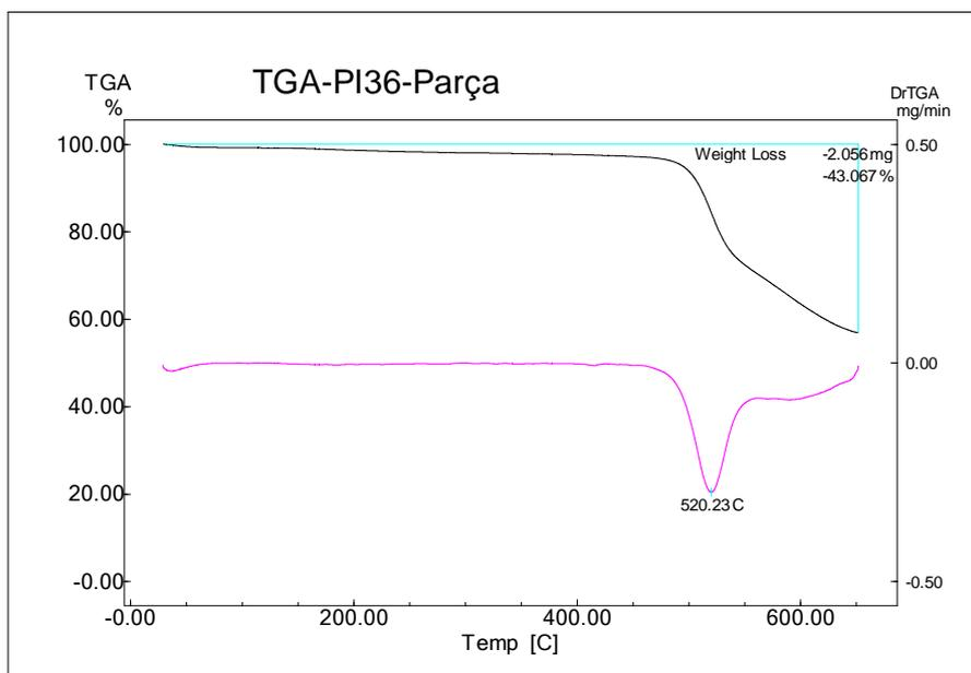
Figure F.1 Thermogram of pure PI (PI36)
