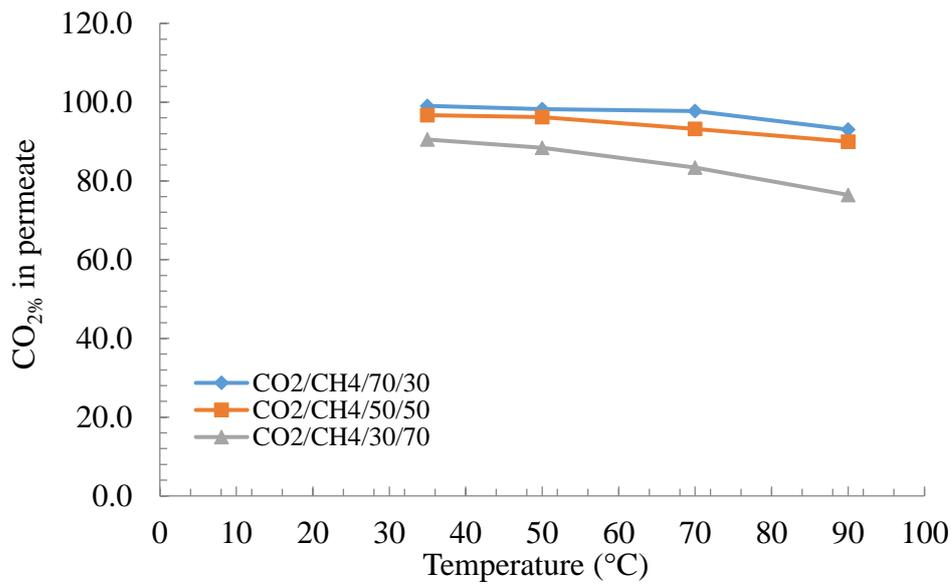
Figure 4.26 CO<sub>2</sub>% in the permeate vs. temperature graph of M7 membrane for different feed gas compositions
