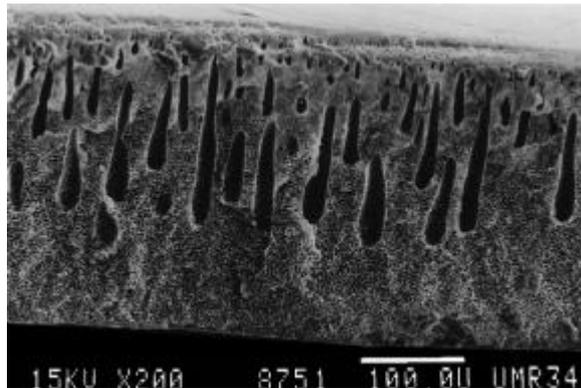
Figure 2.4 The cross-sectional SEM image of PSf membrane produced by coagulating in water by wet phase inversion [12]
