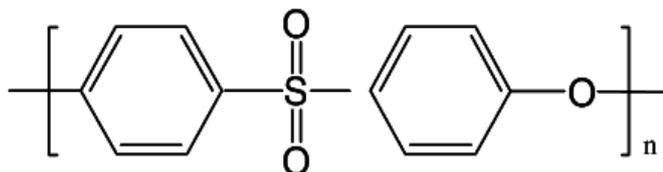
Figure 3.1 Molecular Structure of PES [24]
