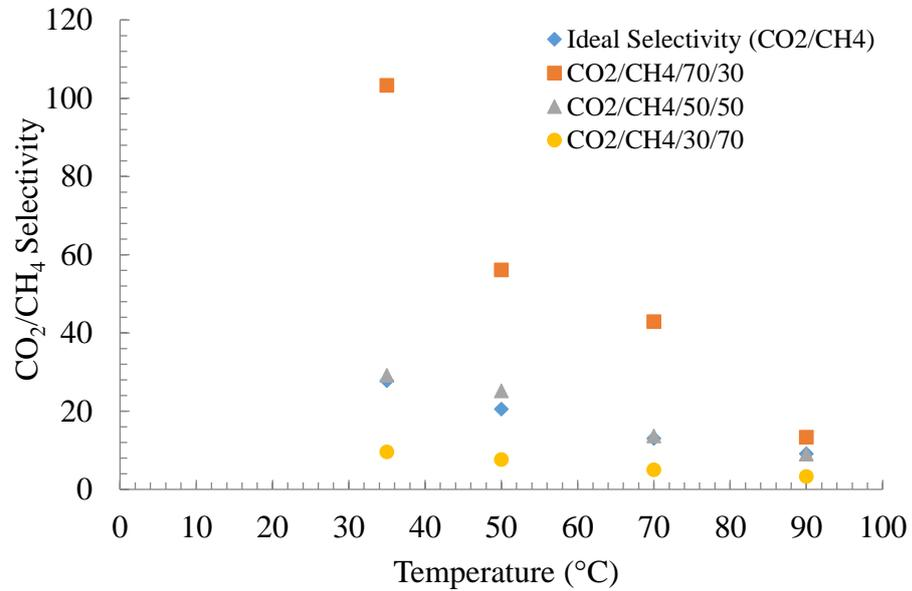
Figure 4.25 CO<sub>2</sub>/CH<sub>4</sub> selectivity versus temperature graph of M7 membrane with different feed gas compositions
