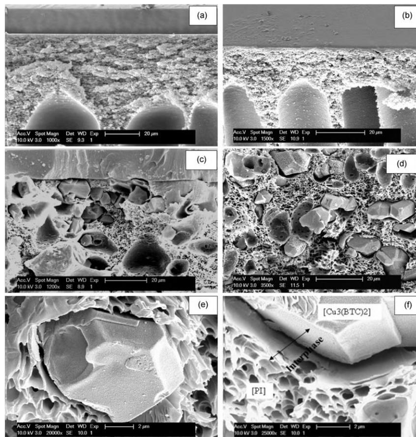
Figure 2.9 (a) unfilled PI membrane (b) unfilled PI/PSf/3/1 membrane (c) PI/Cu<sub>3</sub>(BTC)<sub>2</sub>-30% coated with PDMS (d) PI/Cu<sub>3</sub>(BTC)<sub>2</sub>-30% membrane at low magnification (e) PI/Cu<sub>3</sub>(BTC)<sub>2</sub>-30% membrane at high magnification (f) PI/Cu<sub>3</sub>(BTC)<sub>2</sub> interface [22]
