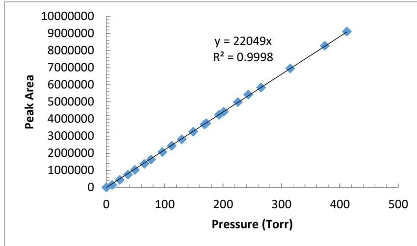
Figure E.1 Calibration curve for CO<sub>2</sub> gas
