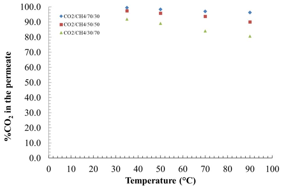
Figure 4.18 CO<sub>2</sub>% in the permeate vs. temperature graph of M3 membrane for different feed gas compositions
