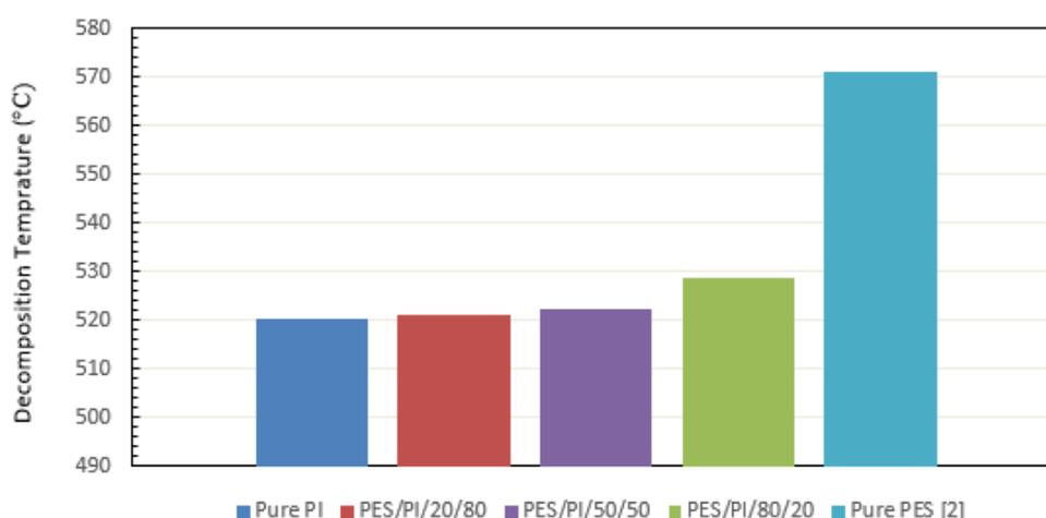
Figure 4.6 Decomposition temperatures of Pure PI, PES/PI/20/80, PES/PI/50/50, PES/PI/80/20 and pure PES [2] membranes
