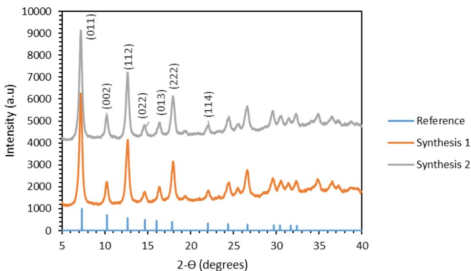
Figure 4.1 X-Ray Pattern of ZIF-8 crystals and reference pattern [26]
