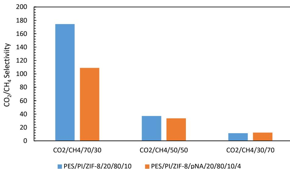
Figure 4.23 Compatibilizer (pNA) effect on CO<sub>2</sub>/CH<sub>4</sub> selectivities of PES/PI/ZIF-8/20/80/10 mixed matrix and PES/PI/ZIF-8/pNA/20/80/10/4 membranes (IR time: 40 sec.)
