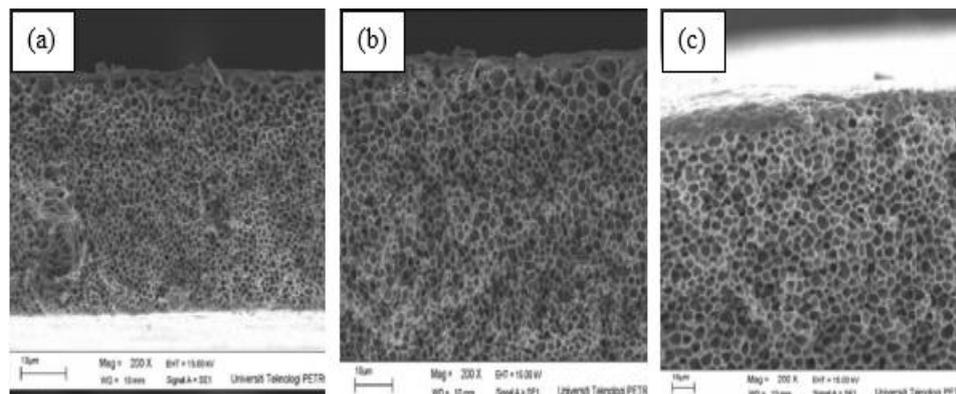
Figure 2.8 SEM photographs of PSf/PI-20% membranes with DCM/NMP (a) 80/20, (b) 50/50 and (c) 20/80 [18]
