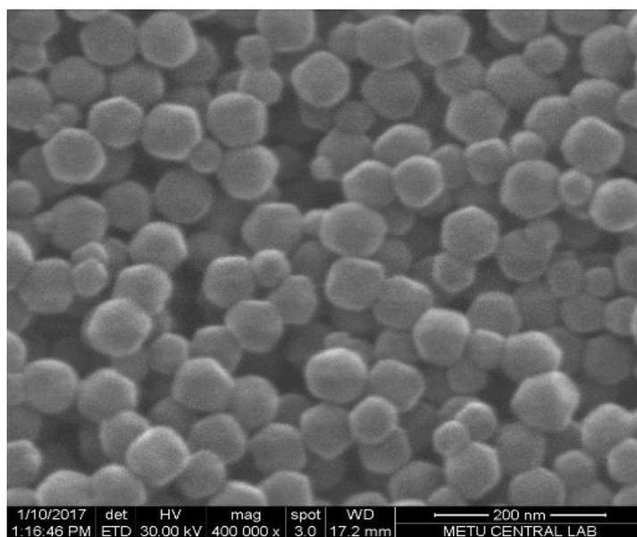
Figure 4.2 The SEM images of the synthesized ZIF-8 crystals
