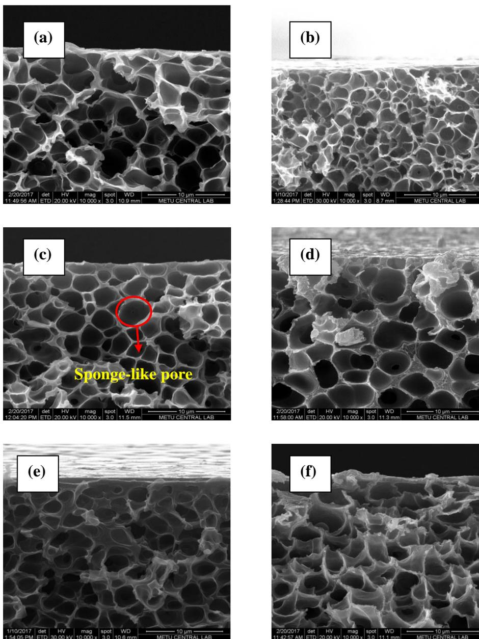
Figure 4.4 (a) PES/PI/20/80, (b) PES/PI/50/50, (c) PES/PI/80/20, (d) PES/PI/ZIF8/20/80/10, (e) PES/PI/ZIF8/PNA/20/80/0/4, (f) PES/PI/ZIF8/PNA/20/80/10/4 without IR
