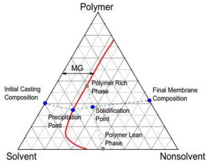
Figure 2.2 Schematic ternary system phase diagram [10]
