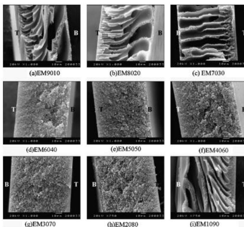
Figure 2.6 The SEM images of membrane cross-sections for different blend compositions [17]
