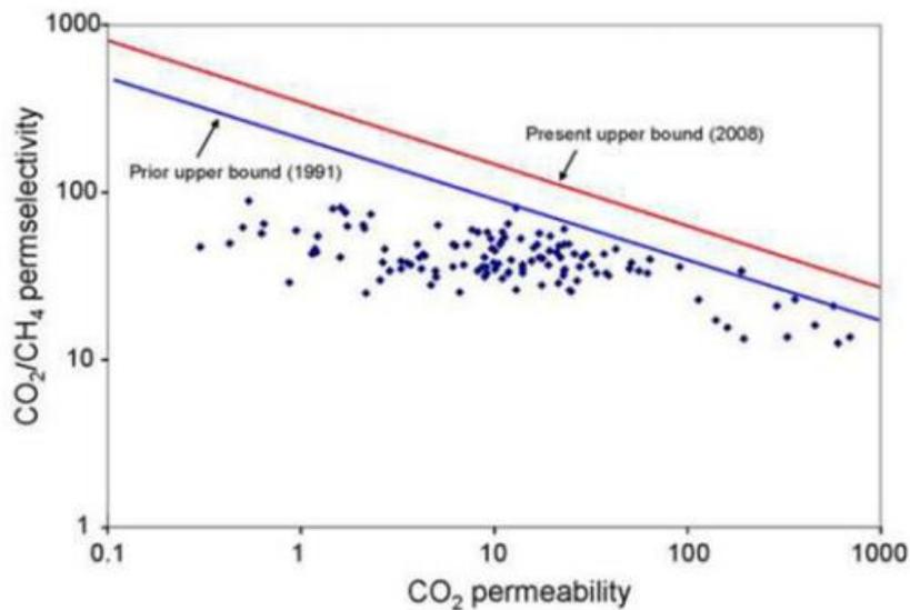
Figure 1.2: Robeson's tradeoff curve for CO<sub>2</sub>/CH<sub>4</sub> pair [3]
