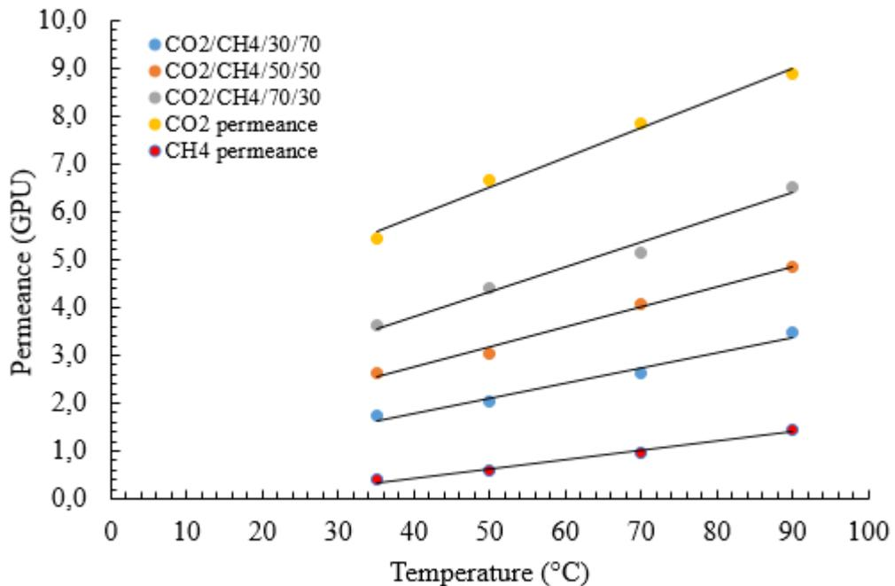
Figure 4.16 Permeance versus Temperature graph of M3 membrane with different feed gas compositions
