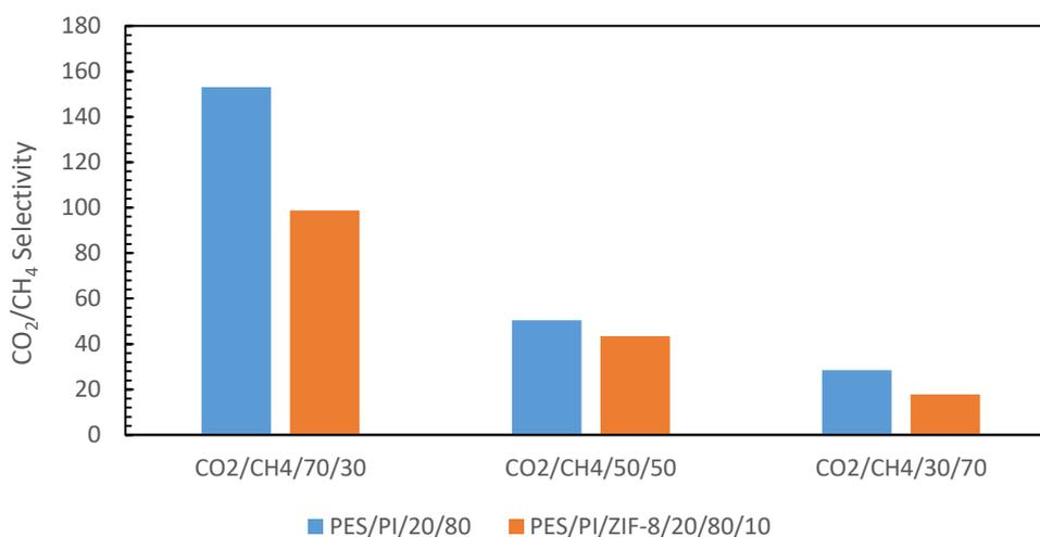
Figure 4.21 Filler material (ZIF-8) effect on CO<sub>2</sub>/CH<sub>4</sub> selectivities of PES/PI/20/80 blend and PES/PI/ZIF-8/20/80/10 mixed matrix membranes (IR time: 80 sec.)
