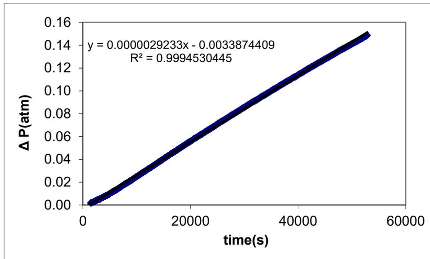
Figure A.1 CO<sub>2</sub> permeance test at 35°C for PES/PI/20/80
