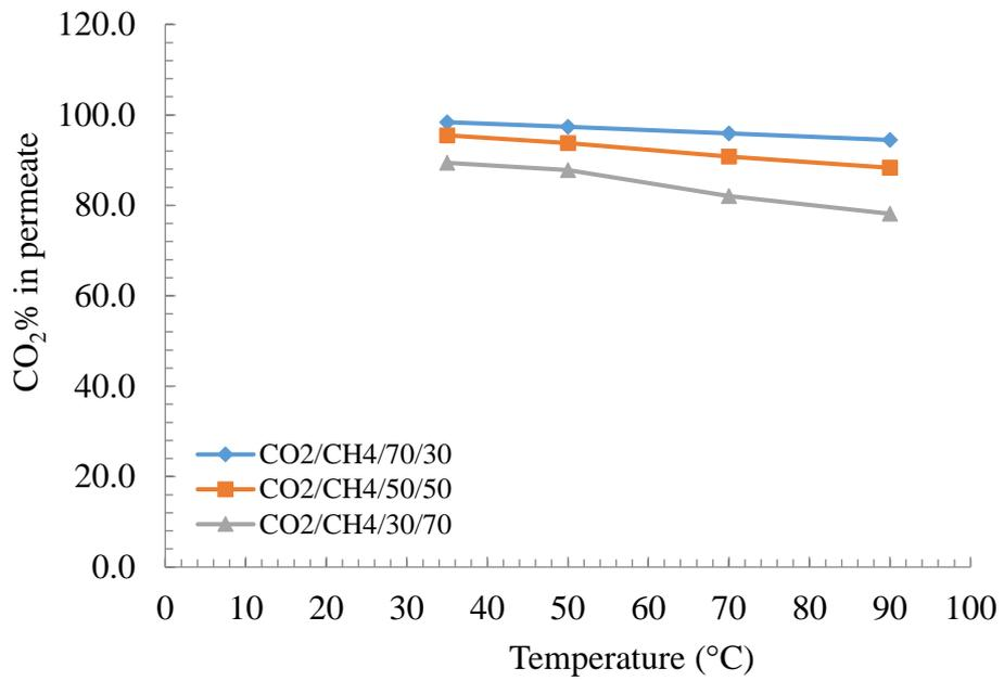
Figure 4.30 CO<sub>2</sub>% in the permeate vs. temperature graph of M8 membrane for different feed gas compositions
