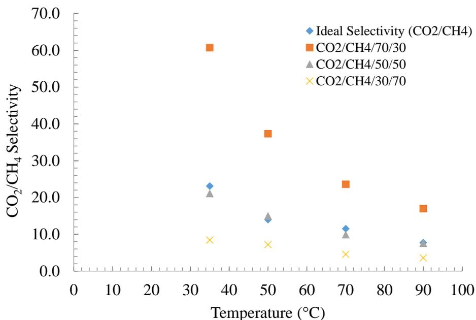
Figure 4.29 CO<sub>2</sub>/CH<sub>4</sub> selectivity versus temperature graph of M8 membrane with different feed gas compositions
