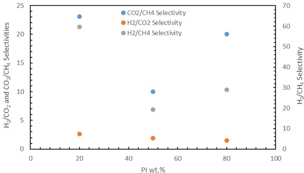
Figure 4.10 H<sub>2</sub>/CO<sub>2</sub>, CO<sub>2</sub>/CH<sub>4</sub> and H<sub>2</sub>/CH<sub>4</sub> selectivities vs PI wt.% graph for blend membranes with 120 sec. IR lamb
