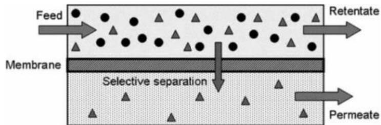
Figure 1.1 The schematic representation of feed, permeate and retentate of membrane [3]
