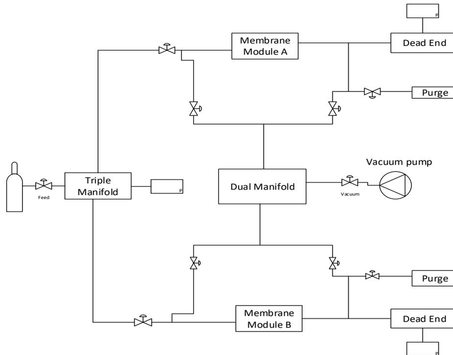
Figure 3.4 Single Gas Permeation Test System
