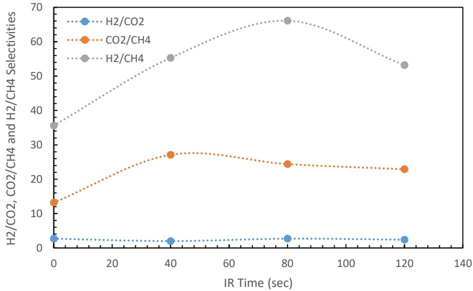
Figure 4.11 H<sub>2</sub>/CO<sub>2</sub>, CO<sub>2</sub>/CH<sub>4</sub> and H<sub>2</sub>/CH<sub>4</sub> selectivities vs IR time graph for PES/PI/ZIF-8/20/80/10 mixed matrix membrane
