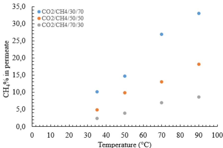
Figure 4.19 CH<sub>4</sub>% in the permeate vs. temperature graph of M3 membrane for different feed gas compositions
