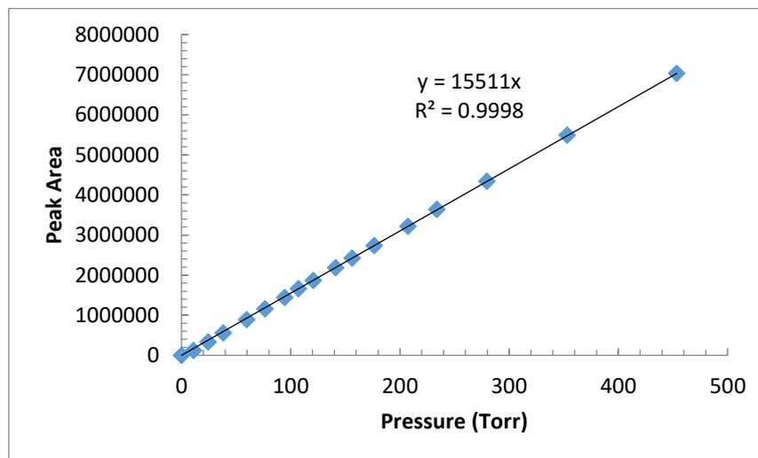
Figure E.2 Calibration curve of CH<sub>4</sub> gas
