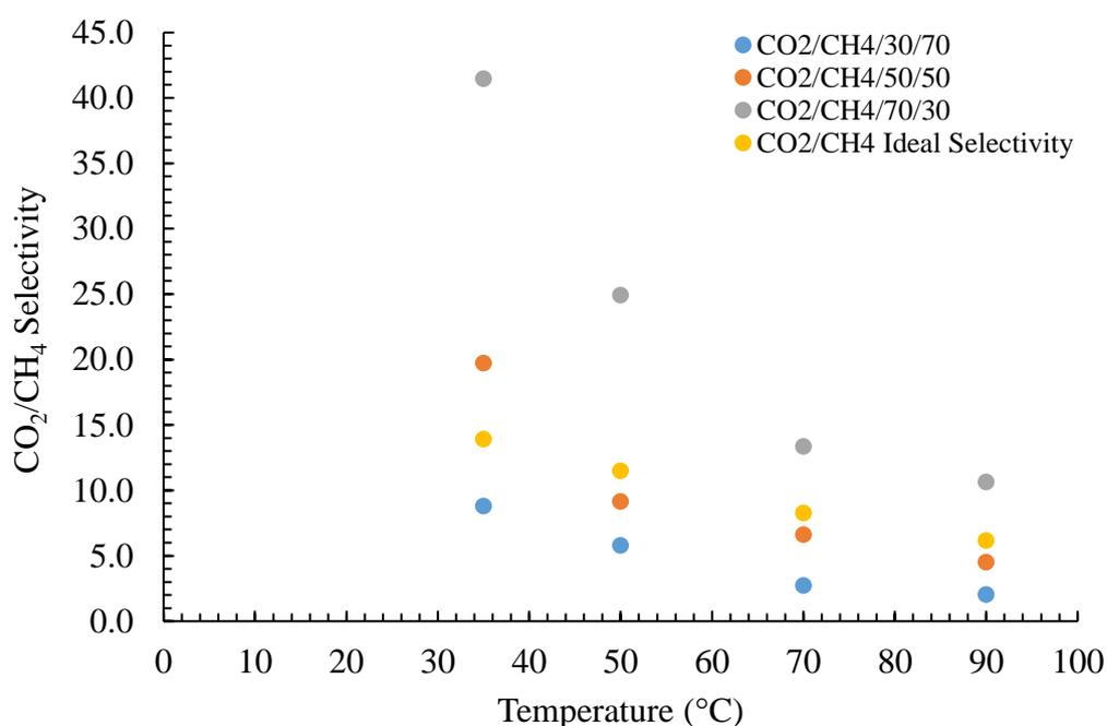
Figure 4.17 CO<sub>2</sub>/CH<sub>4</sub> selectivity versus temperature graph at different feed gas compositions
