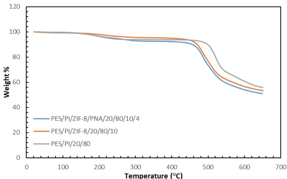
Figure 4.7 TGA curves of PES/PI/20/80, PES/PI/ZIF-8/20/80/10 and PES/PI/ZIF-8/PNA/20/80/10/4 membranes in N<sub>2</sub>
