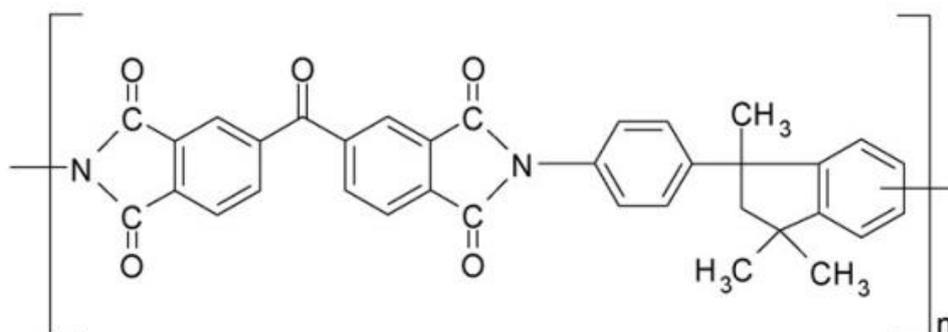
Figure 3.2 Molecular Structure of Matrimid ® 5218 polyimide [25]
