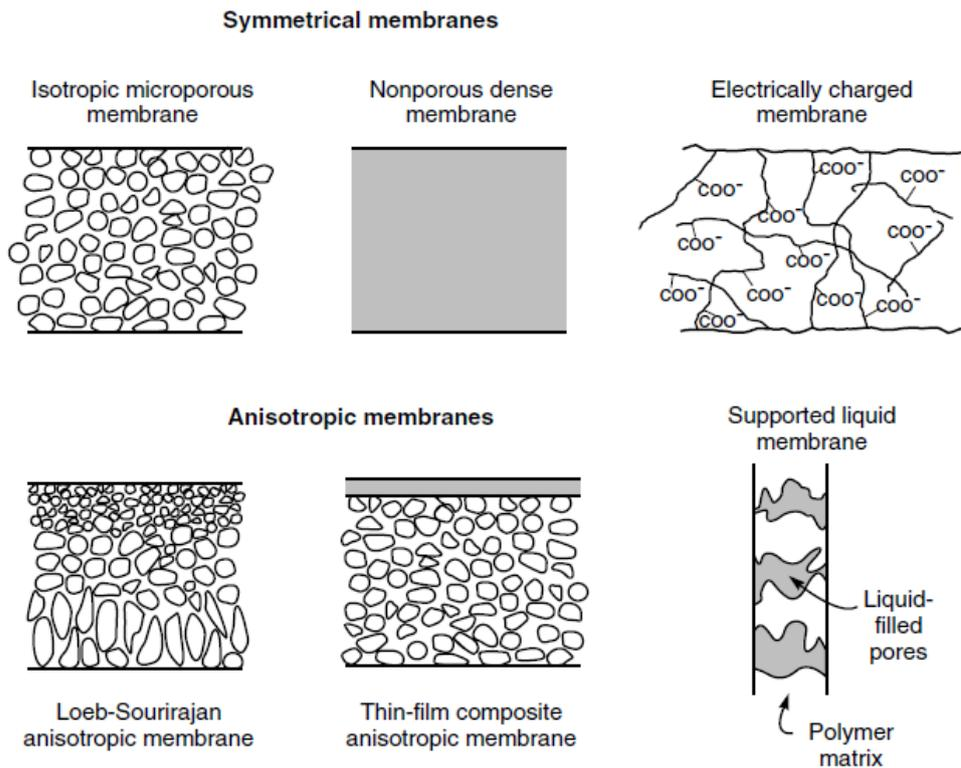
Figure 2.1 The schematic representation of the principal types of membranes [5]
