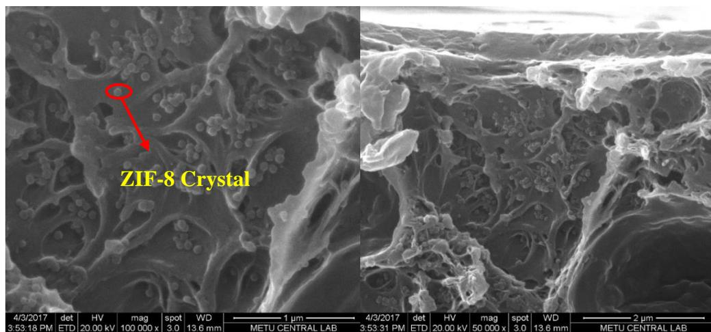
Figure 4.5 Good dispersion of ZIF-8 crystals throughout the membrane cross-section
