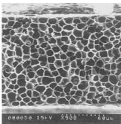
Figure 2.3 SEM image of PSf membrane for RH 80 % [11]
