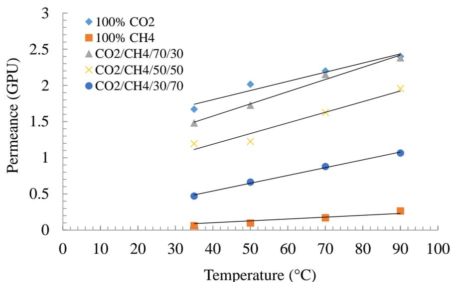
Figure 4.24 Permeance versus temperature graph of M7 membrane with different feed gas compositions
