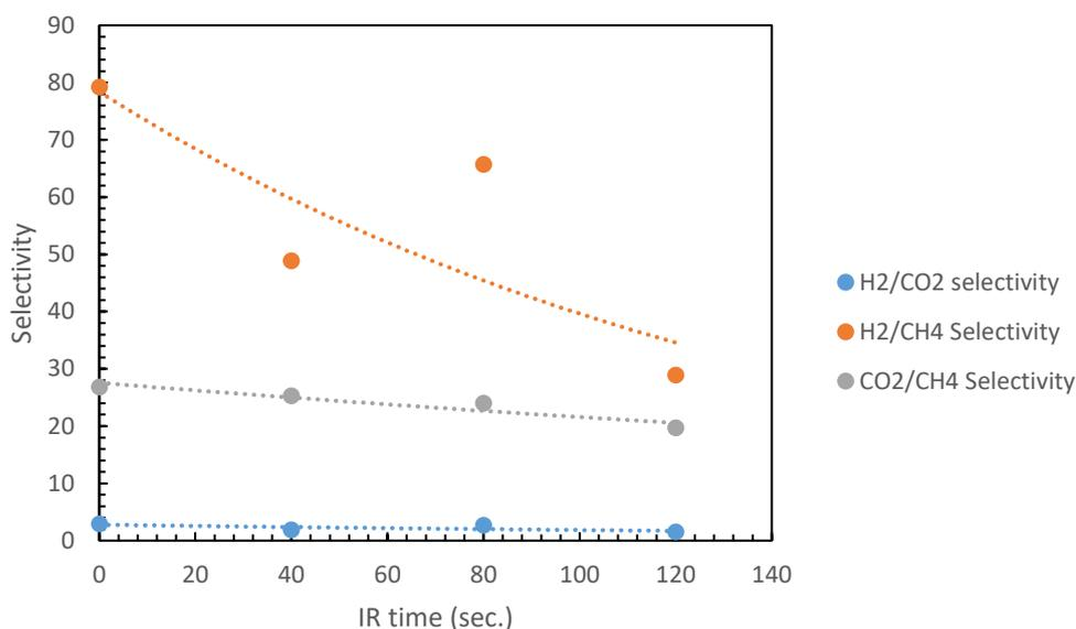
Figure 4.8 Selectivity vs IR time graph for PES/PI/20/80 membrane
