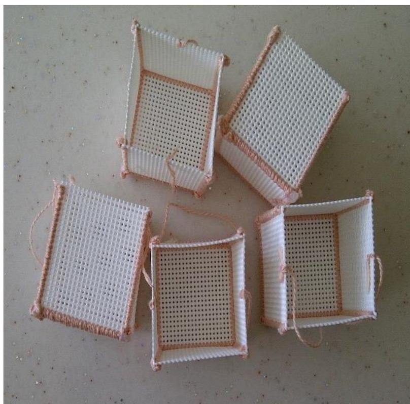
*Figure 2.2.* Plastic mesh baskets used during gelation.
