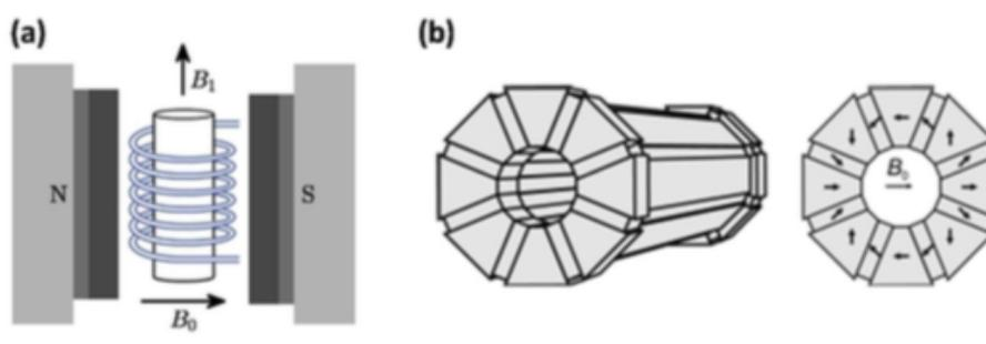
Figure 1.4. a) Parallel plate magnet design. The gap between the plates determines the magnetic field strength,  $B_0$ . The sample is placed in a solenoid radio frequency (RF)
