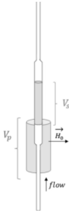
Figure 2.2. Scheme of the flow cell used in the NMR experiments.  $H_0$  represents the static magnetic field vector.  $V_s$  and  $V_p$  are the sensitive volume and pre-polarization volume, respectively.
