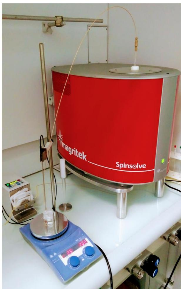
Figure 2.1. System setup for online reaction monitoring
