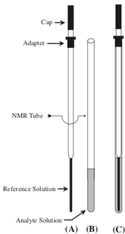
Figure 1.9. An extra capillary insert and NMR tube for external standard method, (A) capillary insert, (B) NMR tube, (C) assembled for the experiment.
