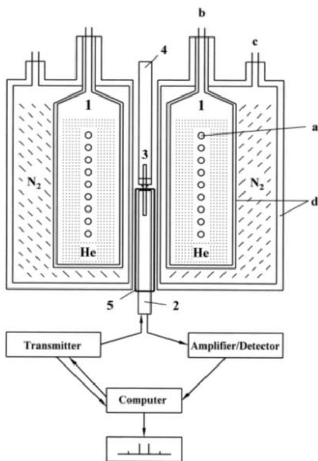
Figure 1.3. Components of an NMR high-field instruments with cryomagnet. 1, cryomagnet assembly; a, magnet coils; b and c, filling columns for liquid helium and liquid nitrogen respectively; d, vacuum jackets of the inner and outer Dewar vessels; 2, probe-head; 3, sample tube; 4, sample changer; 5, shim coils (Friebolin, 2005).
