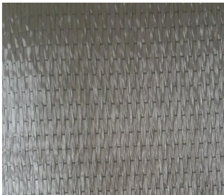
Figure 2.1 UD form of the carbon fibers used in this study
