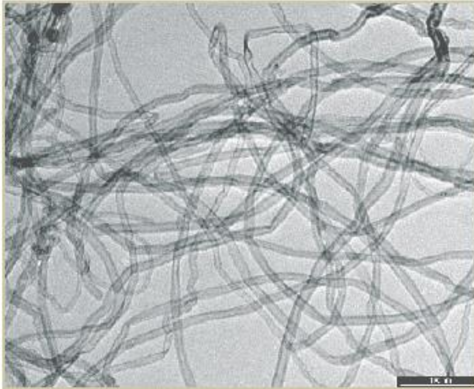
Figure 2.2 TEM image of the multi-walled CNTs used in this study (Nanocyl Inc., the bar in the image is 100 nm)
