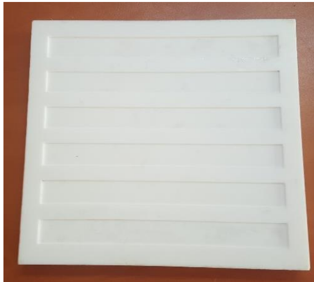
Figure 2.3 Bar-shaped mold cavities used for the production of Neat Epoxy and Epoxy with CNT composite specimens
