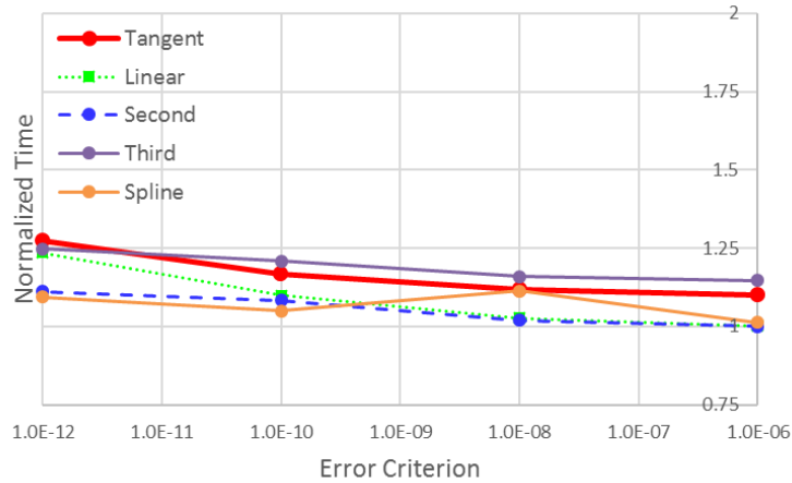
Figure 5.12. Performance comparison of different predictors for contact nonlinearity according to different error criteria and constant step
