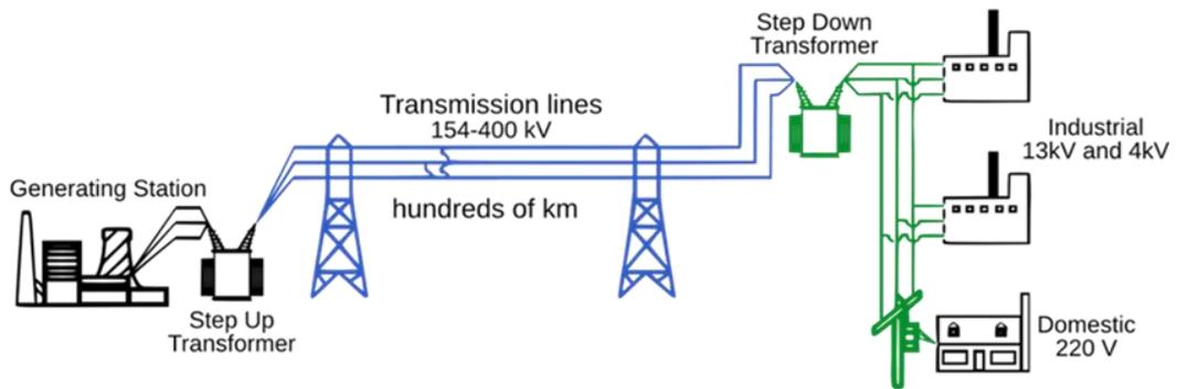
Figure 3.14. Basic transmission sample [60]
