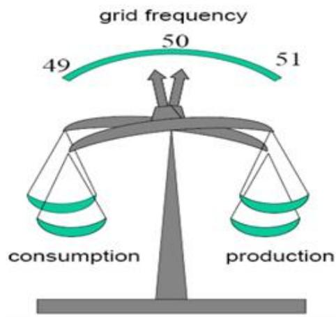
Figure 2.3. Relation between power generation and frequency [11]
