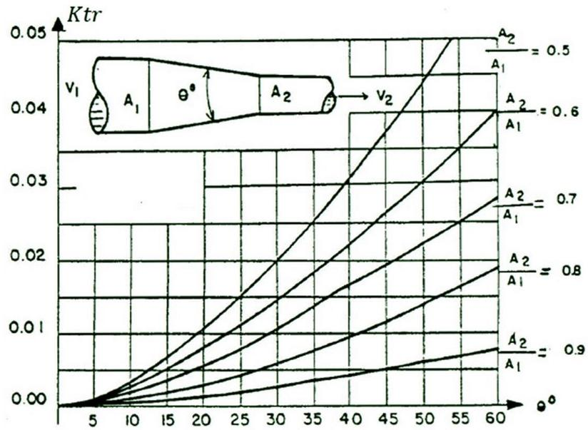
Figure 5.1. Transition loss coefficients for circular contracted conduits [77]
