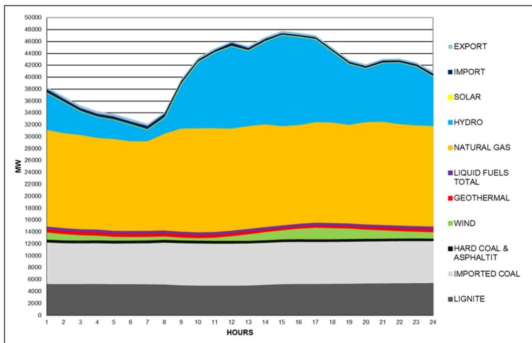
Figure 3.8. Operating status of power plants when meeting the instantaneous peak load of Turkey Interconnected System in 2017 [58]
