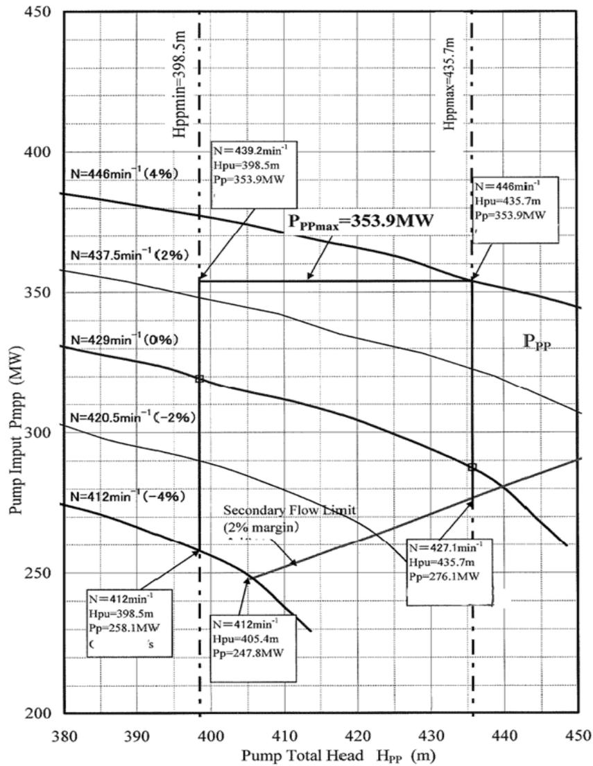
Figure 6.1. Pump Characteristics of Gökçekaya PSH [12]
