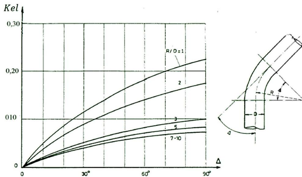
Figure 5.2. Bend loss coefficient [77]
