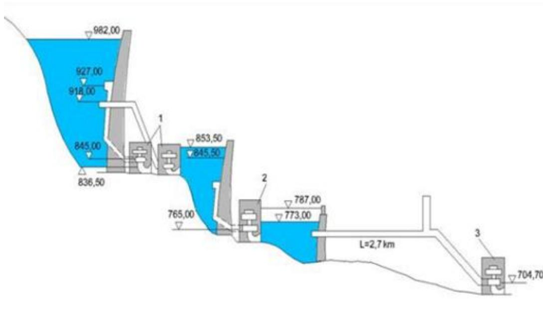
Figure 2.5. Azumi, Midano and Sinrusima PSHs located on the Azusa River [26]
