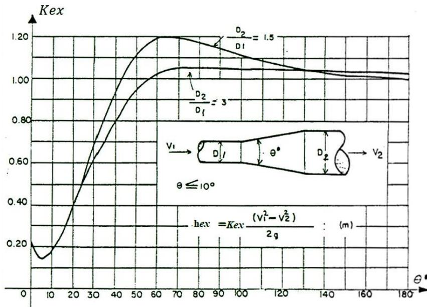
Figure 5.4. Expansion loss coefficient [77]
