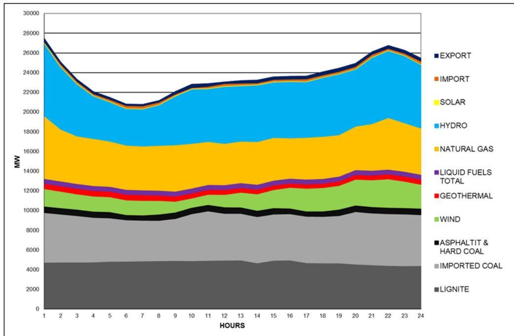
Figure 3.9. Operating status of power plants when the minimum consumption occurs in 2017 [58]
