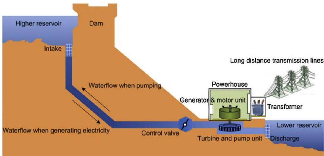
Figure 2.1. Operation cycle of PSH [6]
