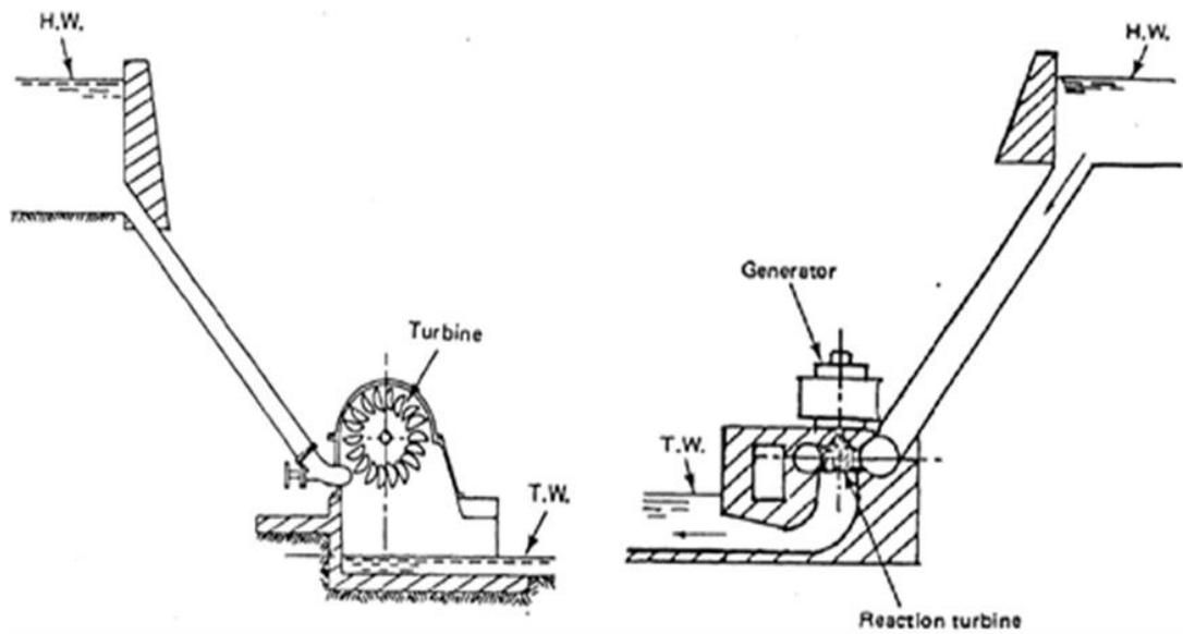
Figure 2.9. Schematic drawings of impulse & reaction turbines [7]
