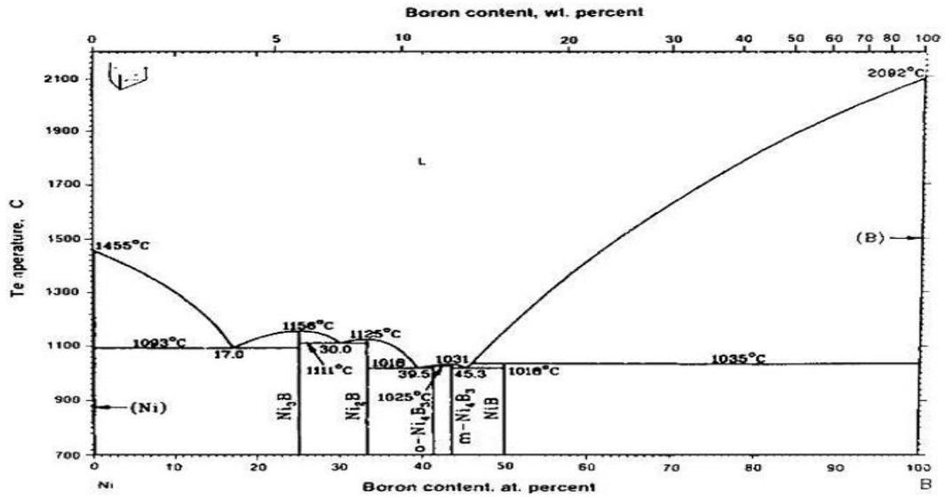
Figure 2.4 Ni-B Phase Diagram [35]
