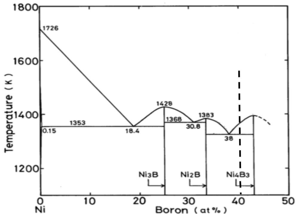
Figure 3.1 Partial phase diagram of Ni-B binary system [44]
