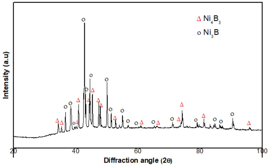
Figure 4.14 High temperature XRD pattern of the 60 h milled  $\text{Ni}_{60}\text{B}_{40}$  at 800 °C.
