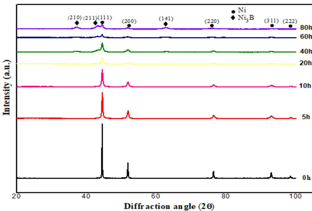
Figure 4.9 X-Ray diffraction patterns of  $\text{Ni}_{60}\text{B}_{40}$ , initial powders and powders ball milled for 5, 10, 20, 40, 60 and 80 h
