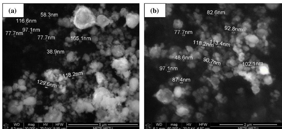
Figure 4.12 High Resolution SEM images for Ni<sub>60</sub>B<sub>40</sub> composition powder milled (a) 60 h (b) 80 h
