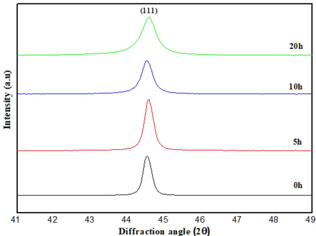
Figure 4.7 X-Ray diffraction peak of (111) for unmilled and milled pure Ni powders for different time periods
