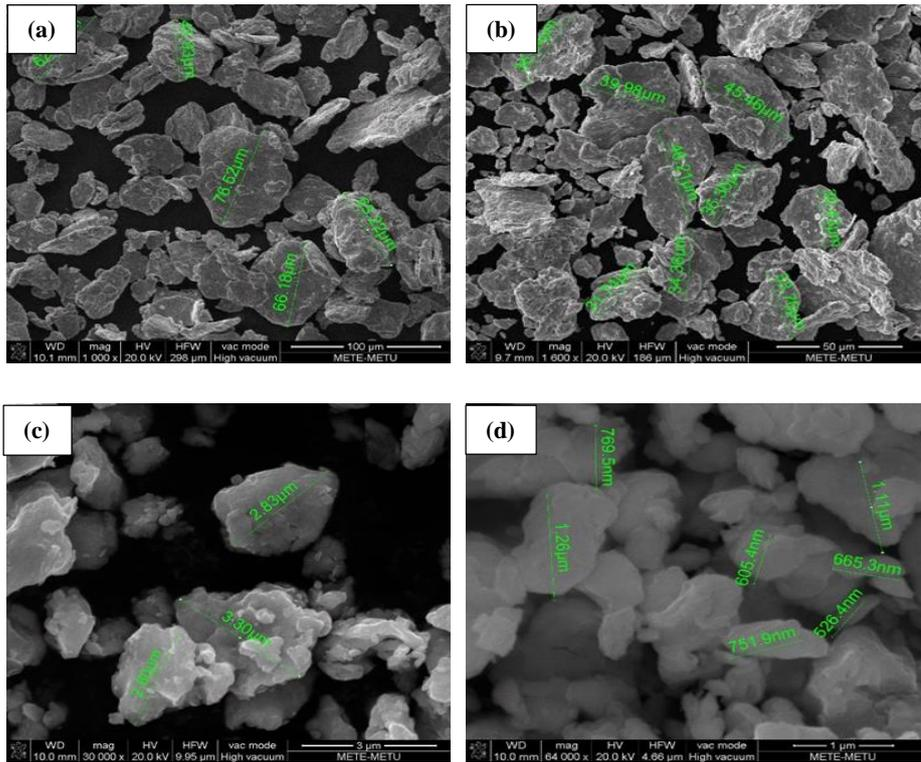
Figure 4.8 SEM images of (a) unmilled pure Ni powders and powders milled for (b) 5 h, (c) 10 h, (d) 20 h
