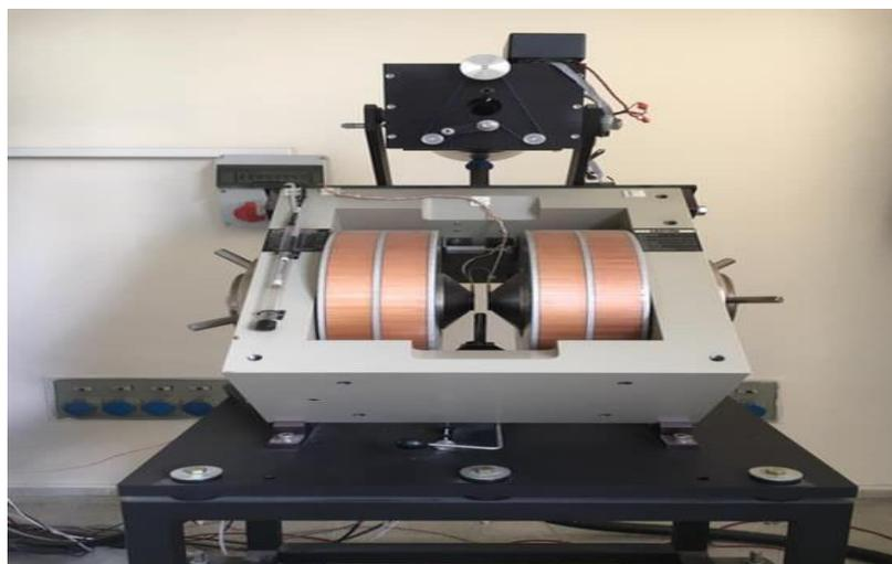
Figure 3.6 ADE Magnetics EV/9 Vibrating Sample Magnetometer (VSM) under a maximum applied field of 18000 Oe.
