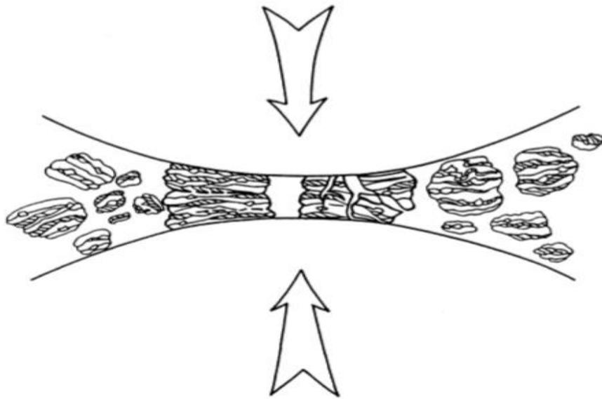
Figure 2.6 Ball-powder-ball collision of powder mixture during mechanical alloying [81]
