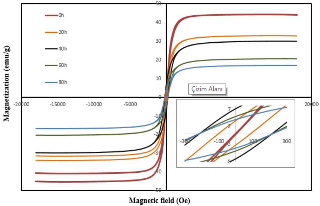
Figure 4.15 Hysteresis curves for initial  $\text{Ni}_{60}\text{B}_{40}$  powder and powders milled for different time periods
