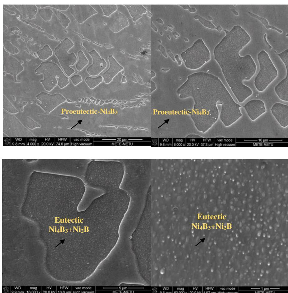
Figure 4.2 SEM images of Ni<sub>60</sub>B<sub>40</sub> bulk alloys showing pro-eutectic and eutectic intermetallic phases
