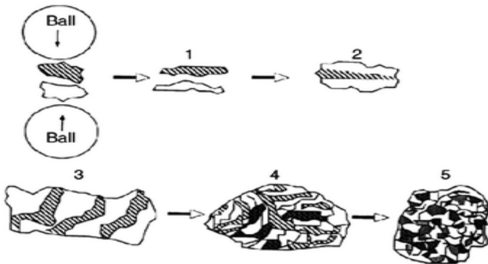
Figure 2.7 Evolution of different stages of mechanical alloying [81]
