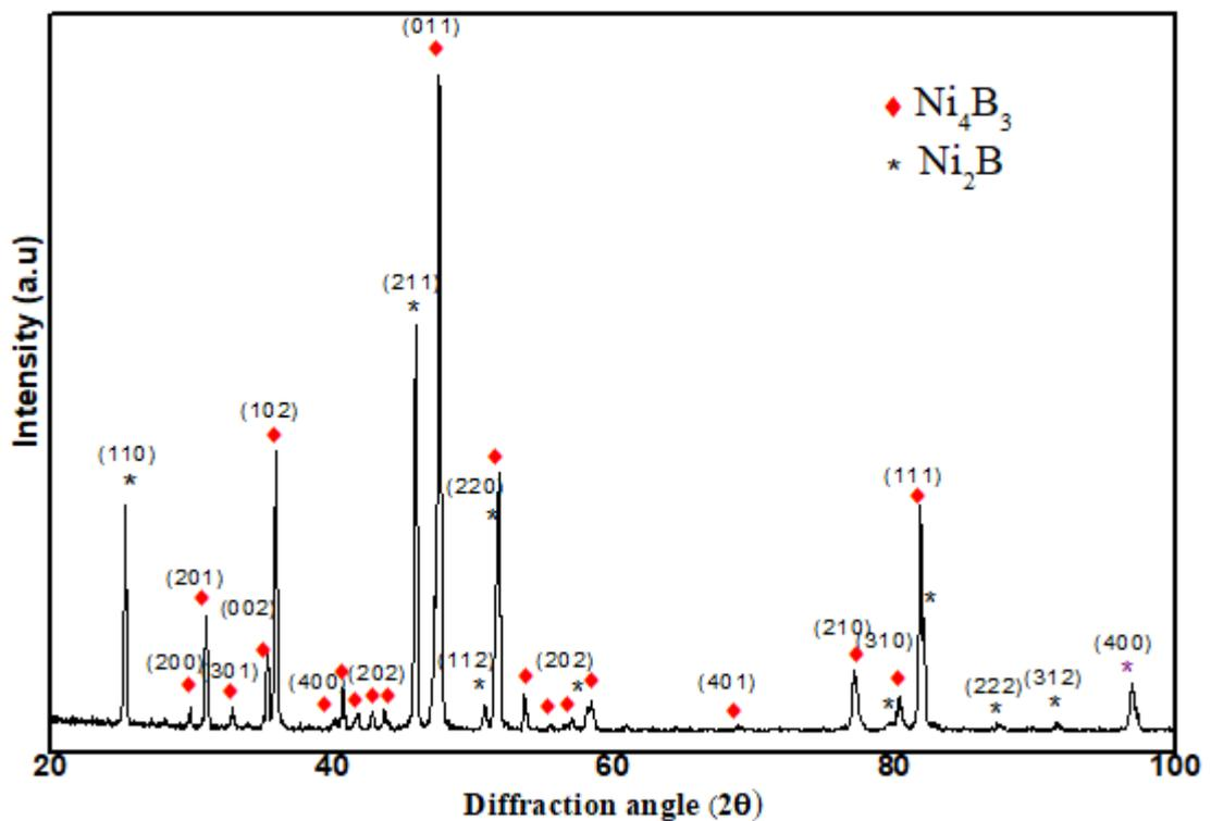
Figure 4.1 X-Ray diffraction patterns of Ni<sub>60</sub>B<sub>40</sub> bulk alloy rod
