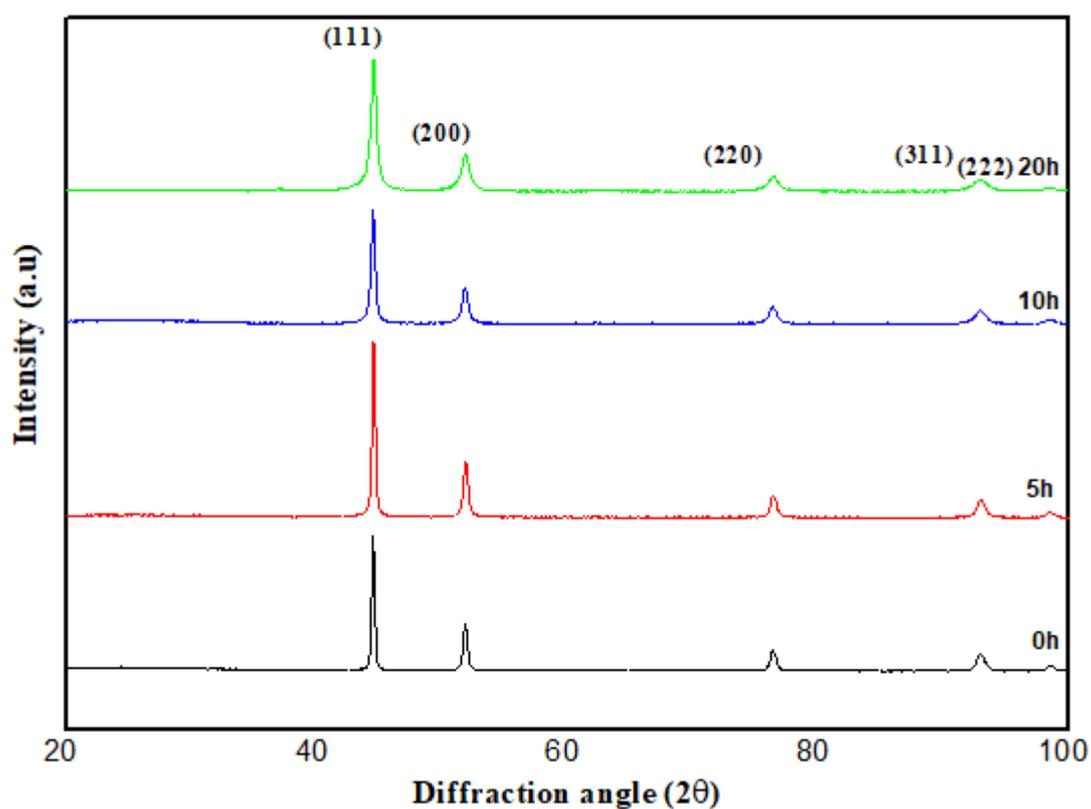
Figure 4.6 X-Ray diffraction patterns for unmilled and milled pure Ni powders for different time periods.
