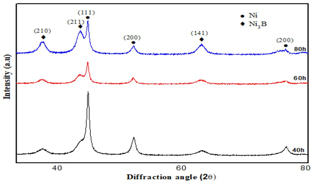
Figure 4.10 X-Ray diffraction patterns of  $\text{Ni}_{60}\text{B}_{40}$  nanoalloys in detail for 40, 60 and 80 h milling times
