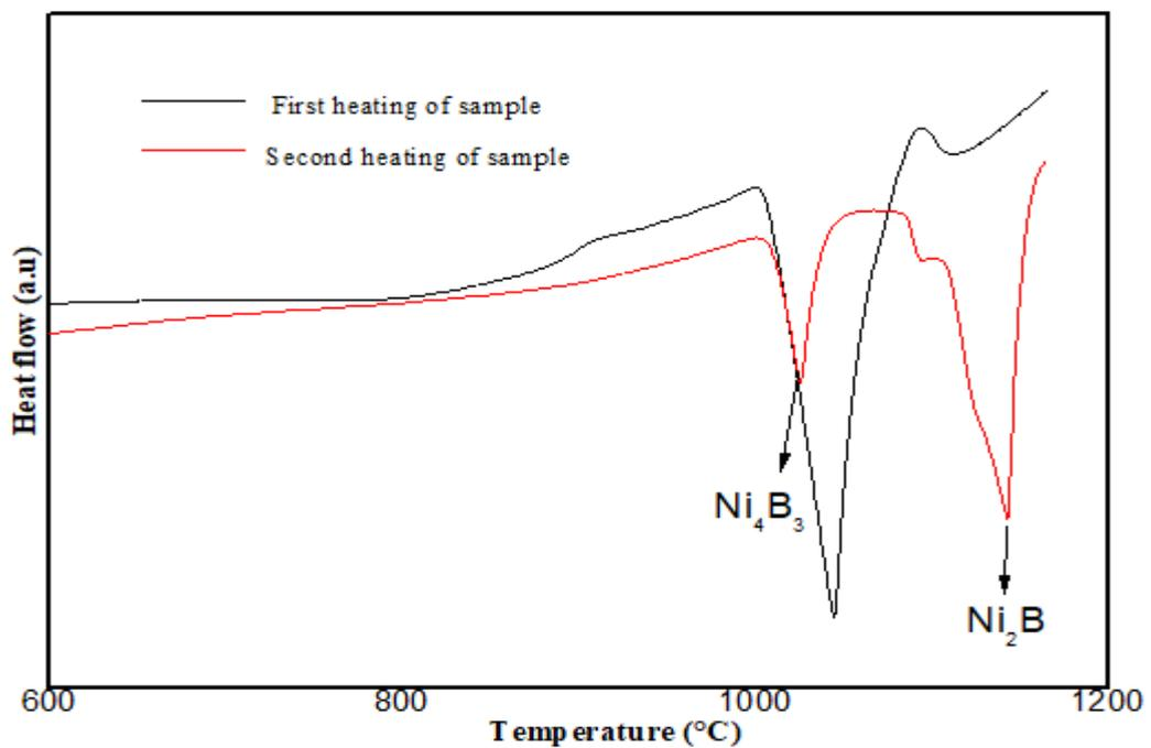
Figure 4.4 DSC analysis of the  $\text{Ni}_{60}\text{B}_{40}$  bulk alloys
