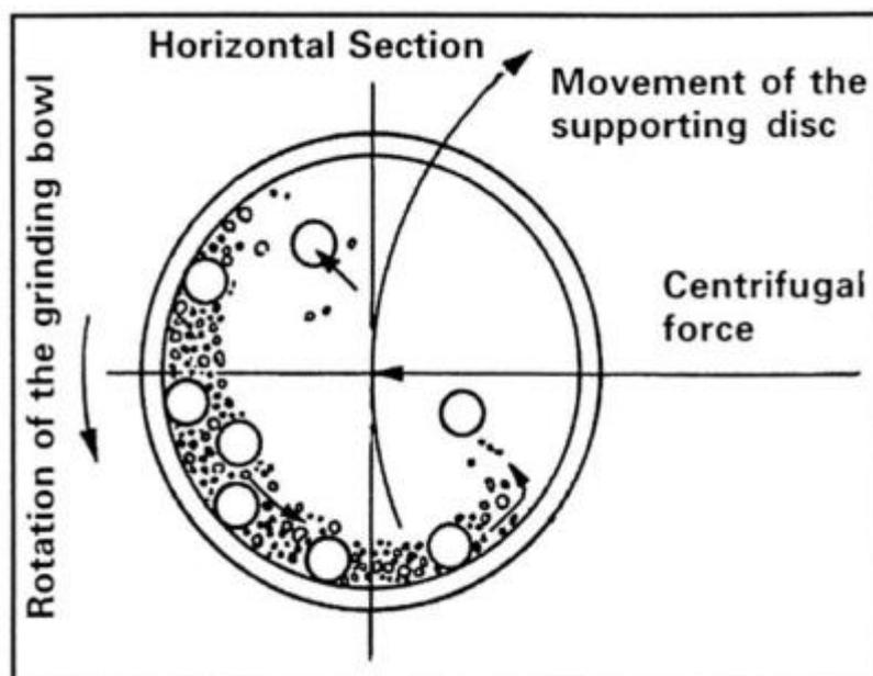
Figure 2.5 Schematic view of ball and powder mixture [81]
