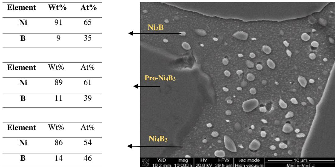
Figure 4.3 EDS results of  $\text{Ni}_{60}\text{B}_{40}$  bulk alloys
