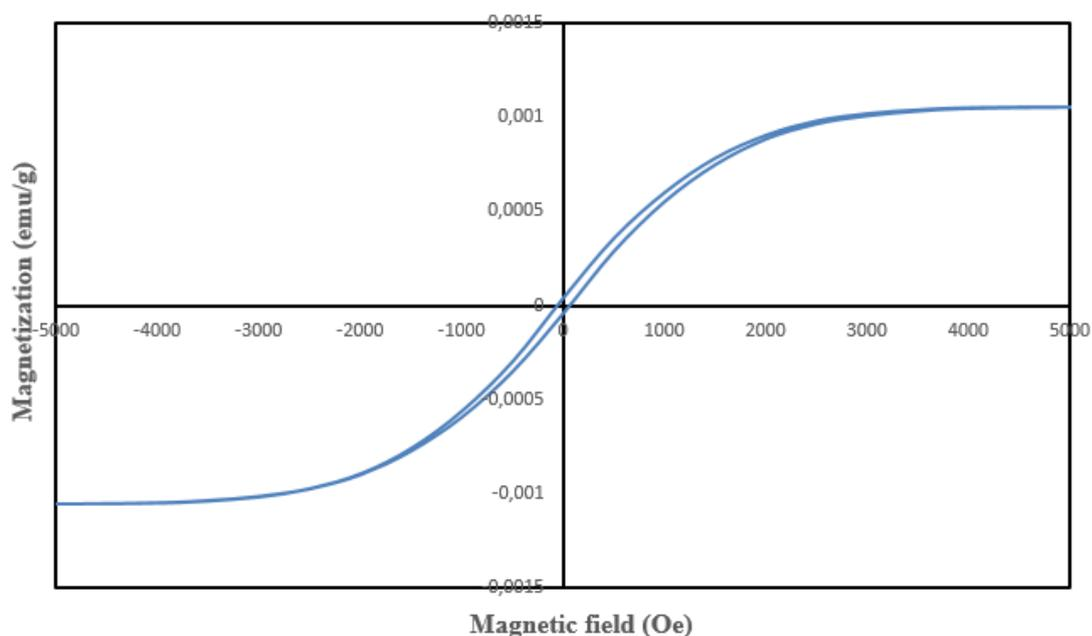
Figure 4.5 Hysteresis curves for Ni<sub>60</sub>B<sub>40</sub> bulk alloys
