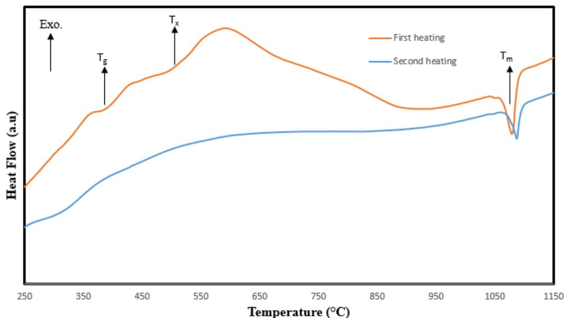
Figure 4.13 DSC analyses of the milled Ni<sub>60</sub>B<sub>40</sub> powder for 80 h
