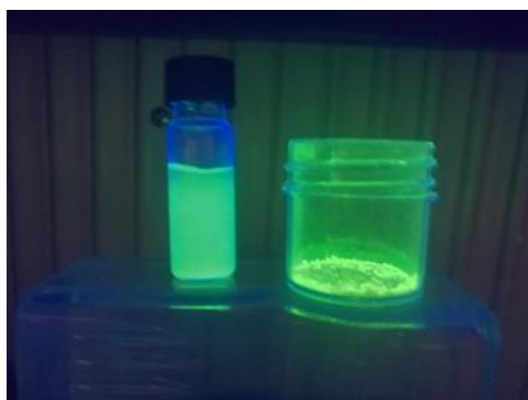
Figure 32. Image of \text{Gd}_{0.90}\text{Ce}_{0.05}\text{Tb}_{0.05}\text{BO}_3 samples both in water-dispersed and solid forms under UV lamp, 366 nm.
