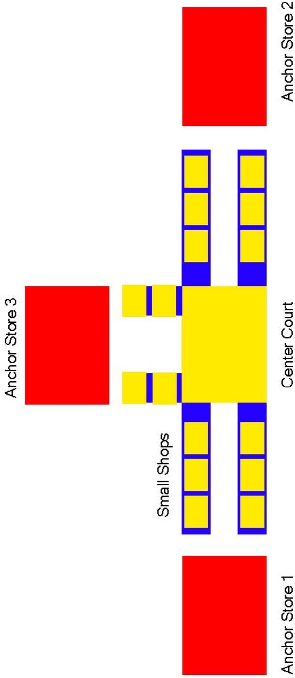
Figure 3.16: Arrangement of stores according to the Dumb-bell plan.
