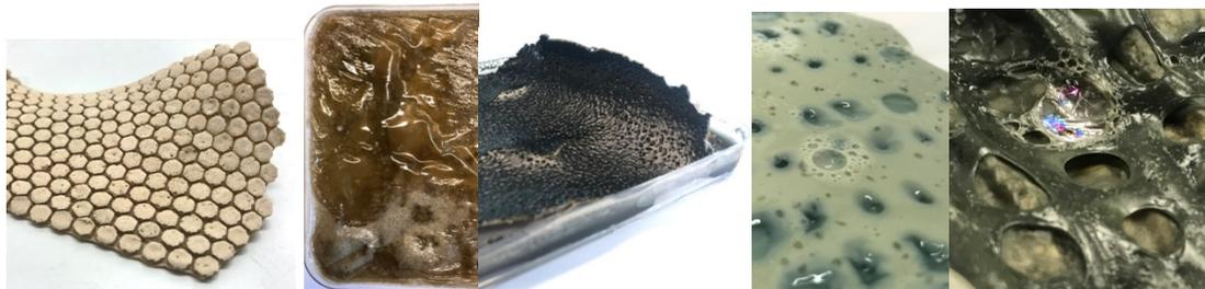
*Figure 5.12.* (From left to right) The pattern achieved by mold, color and texture change owing to drying treatment in different temperatures (50C, 60 C), perforated surface provided by cabbage water drops.
