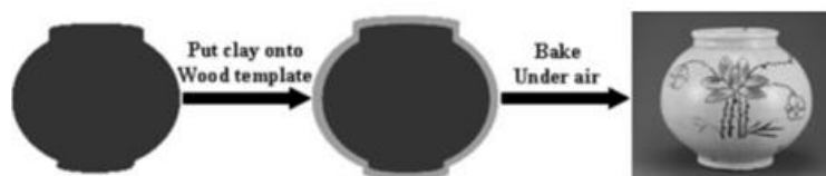
Figure 4.7. Schematic representation of nanocasting concept, reprinted from [53].
