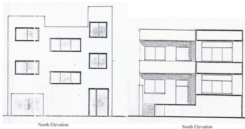
Figure 132. The comparison of openings in two facades of a house: left (street-face façade) right (the façade looks to the yard). source: (Tabriz Municipality's Archive)
