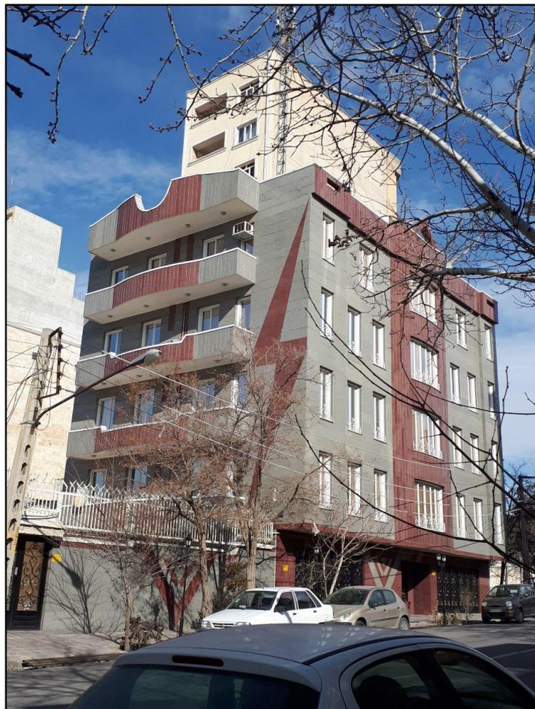
Figure 139. Stone cladding in different colors was used in arbitrary shapes and sometimes accidentally. source: (Author, 2017)
