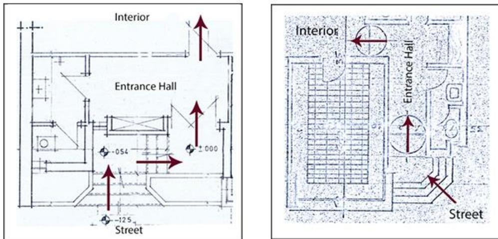
Figure 121. Entrance spaces of houses built in the early 1980s; Creating a change of view or deviation prohibit a person standing on the door step of the open door to see the interior of the house. source: (Tabriz Municipality's Archive)
