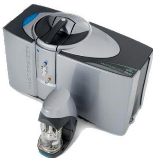
**Figure 12** Particle size analyzer (Malvern Instruments, Mastersizer 3000 hydro, Worcestershire, UK).
