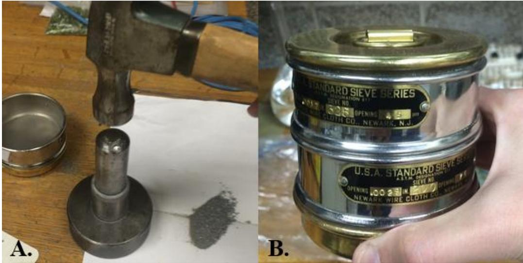
**Figure 7.2.** A. Samples are crushed and powdered by using hammer B. Samples ground to pass 325 to 200 mesh sieves
