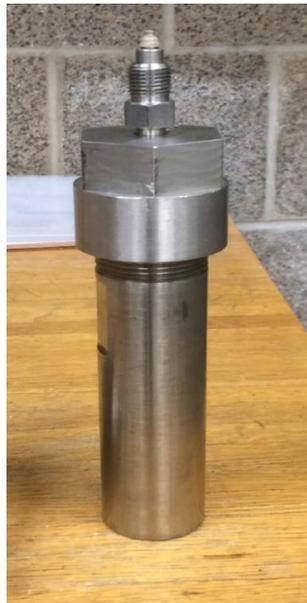
**Figure 7.4.** Titanium made vessel used in the experiments
