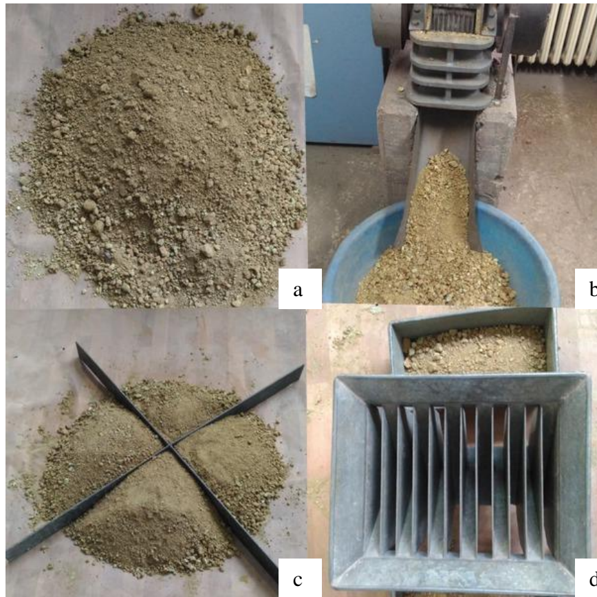
Figure 4.4 Preparation of Eskişehir-Mihalıççık ore for pre-concentration studies: a) Run-of-mine after drying, b) Coarse crushing of the run-of-mine, c) Dividing the ore pile into representative fractions by cone and quartering, d) Representative sampling of the sample by using Jones Riffle separator for obtaining smaller representative fractions
