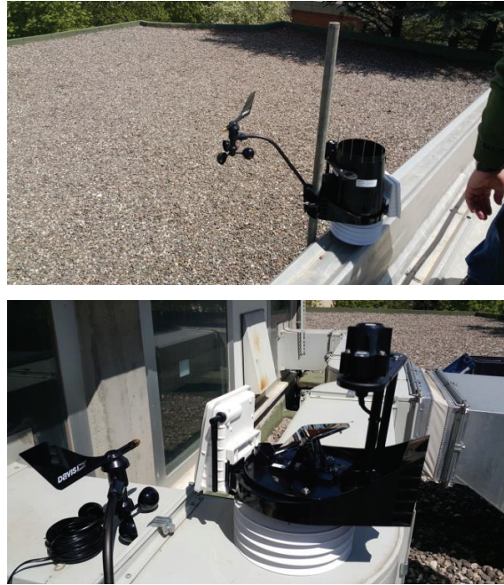
Figure 63. Davis Instruments Vantage Pro2 Weather Station installed at roof of Environmental Engineering Department
