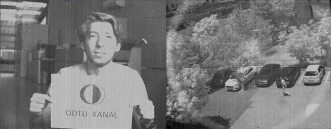
**Figure 3.19:** Not optimized snapshots taken by 25  $\mu\text{m}$  pitch 640x512 NIR/SWIR InGaAs camera.
