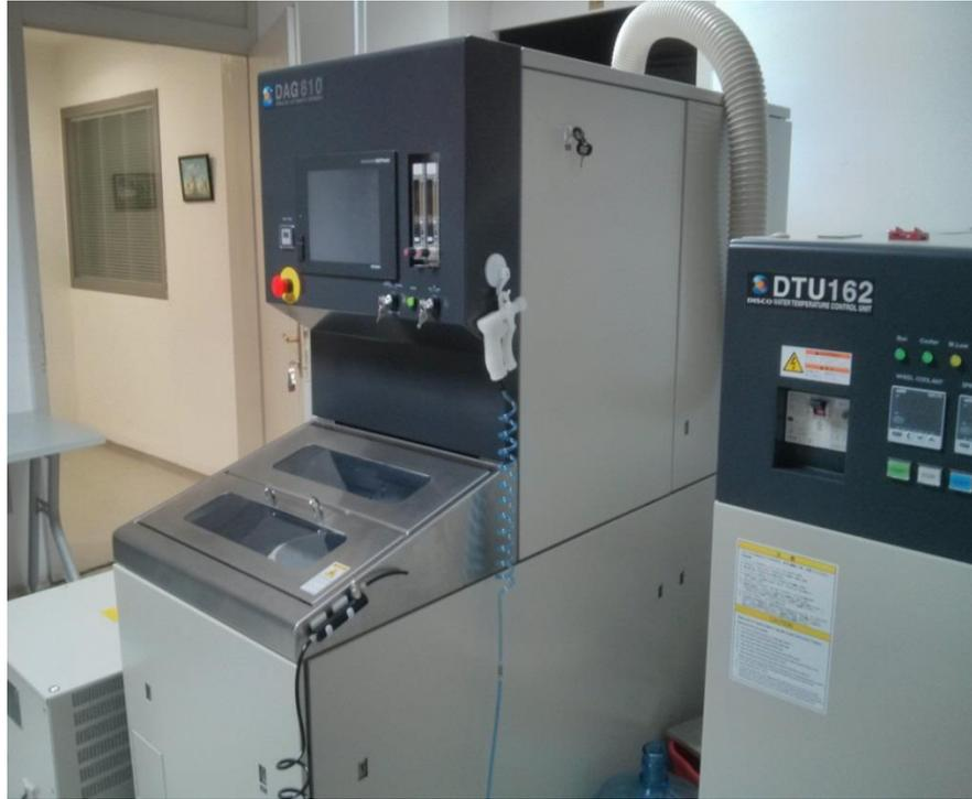
**Figure 3.7:** “DAG810” substrate grinding machine utilized for substrate removal.
