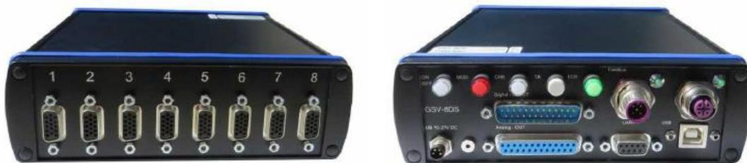
**Figure B-3.** Front and back sides of the amplifier
