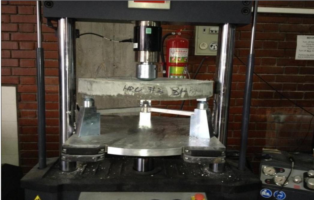
Figure 3.9 Set-up for round panel tests
