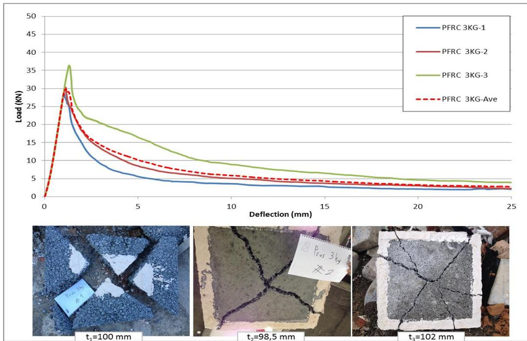
Figure 4.9 Load deflection curves and crack formations of PFRC 3kg samples with square panel test for 28 days.
