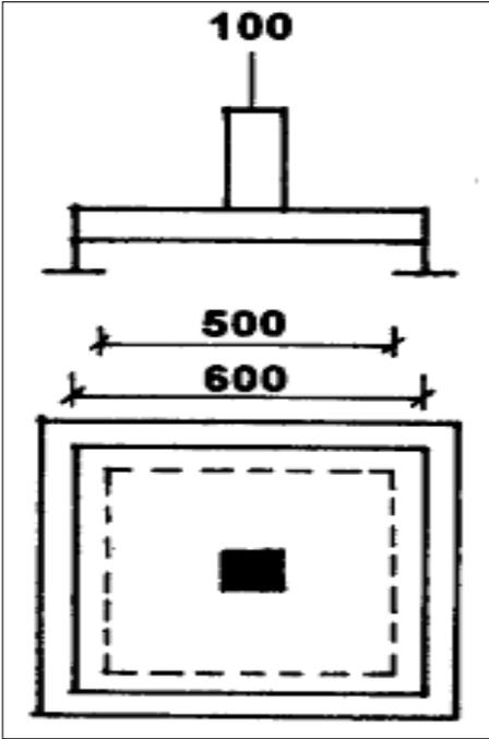
Figure 2.16 Set up for square panel test (EFNARC, 1996).
