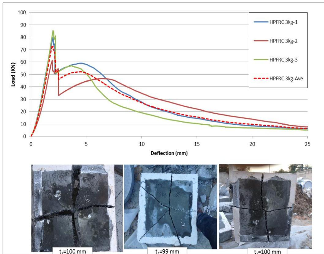
Figure 4.3 Load deflection curves and crack formations of HPFRC 3 kg samples with square panel test for 28 days.
