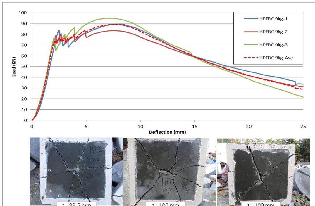
Figure 4.5 Load deflection curves and crack formations of HPFRC 9 kg samples with square panel test for 28 days.
