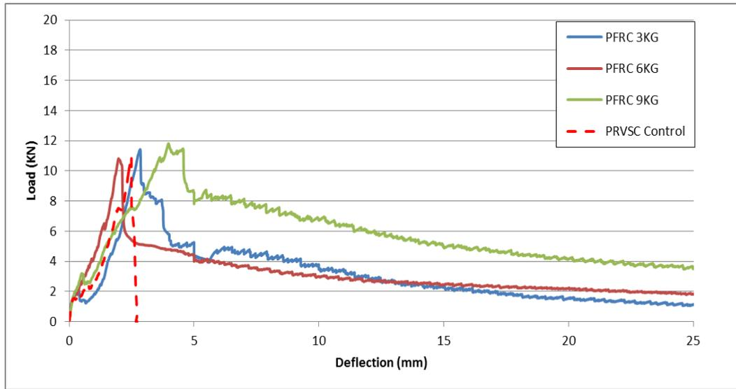
Figure 4.24 Comparison of load deflection curves of PFRC mixes with round panel test for 28 days.
