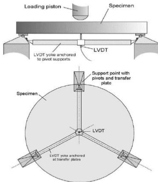
Figure 2.15 Plan and profile view of ASTM 1550 (ASTM C 1550, 2012)
