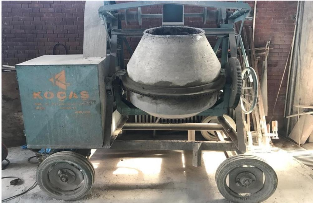
Figure 3.3 Rotary drum mixers
