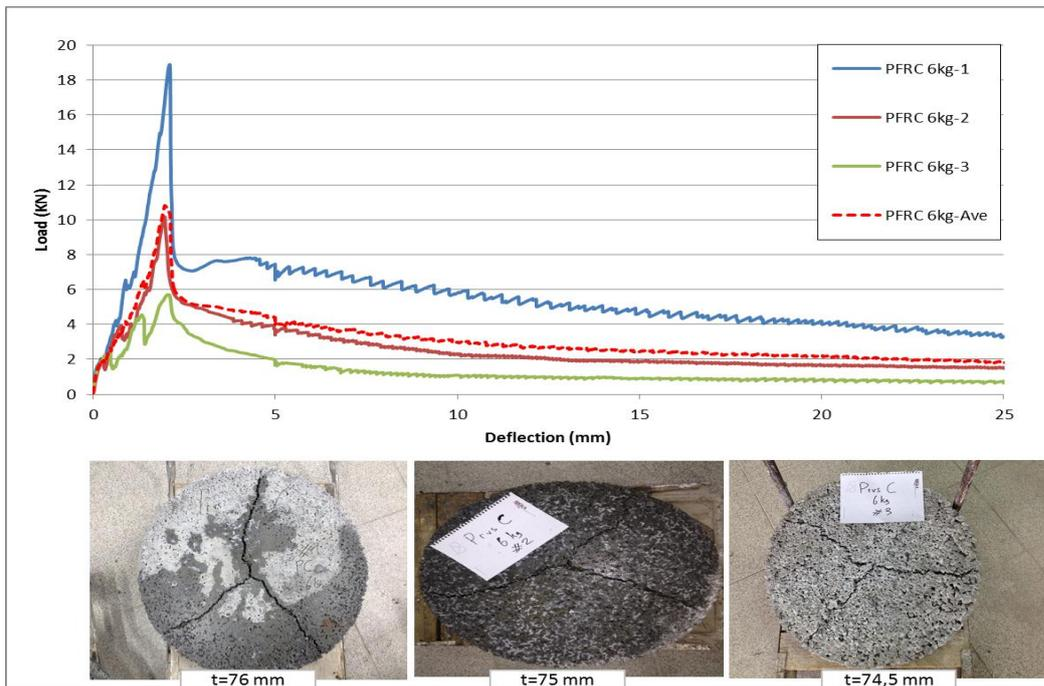
Figure 4.22 Load deflection curves and crack formations of PFRC 6kg samples with round panel test for 28 days.
