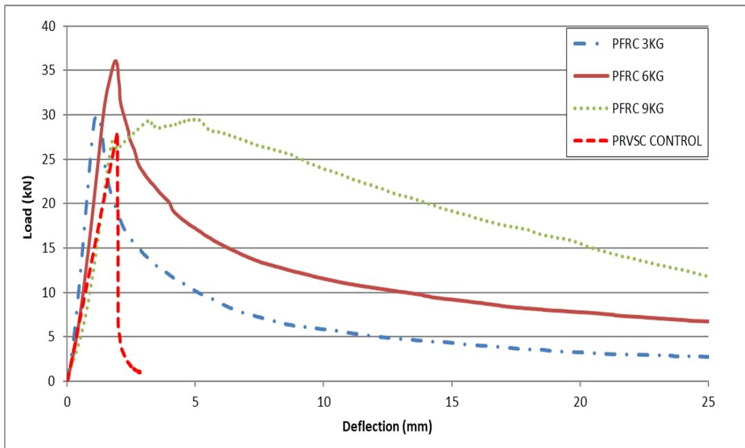
Figure 4.12 Comparison of load deflection curves of PFRC mixes with square panel test for 28 days.
