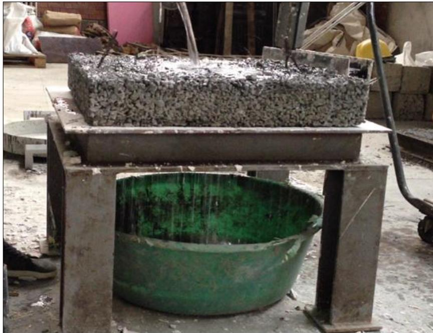
Figure 3.6 Test for infiltration rate of pervious concrete
