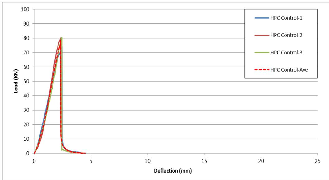
Figure 4.2 Load deflection curves of HPC Control samples with square panel test for 28 days.
