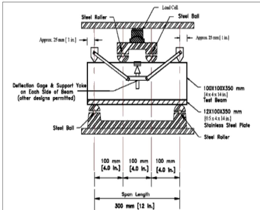
Figure 2.13 Schematic of apparatus ASTM C1399 (2010).
