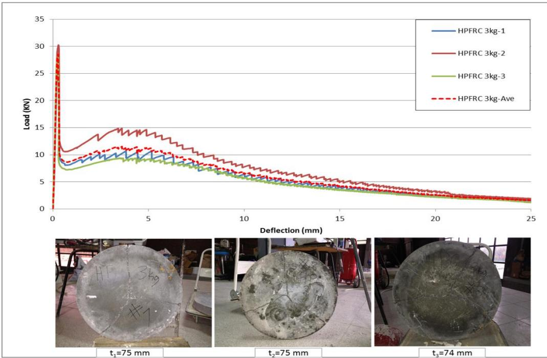
Figure 4.15 Load deflection curves and crack formations of HPFRC 3 kg samples with round panel test for 28 days.
