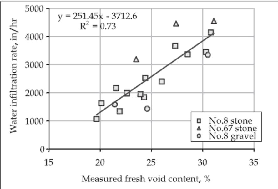
Figure 2.11 Relationship of water infiltration rate and void content in pervious concrete (Obla, 2010).
