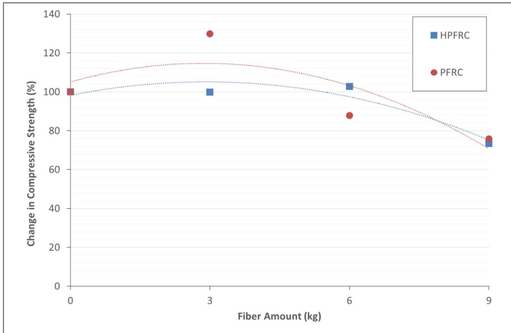
Figure 4.1 Change in compressive strength of all mixes
