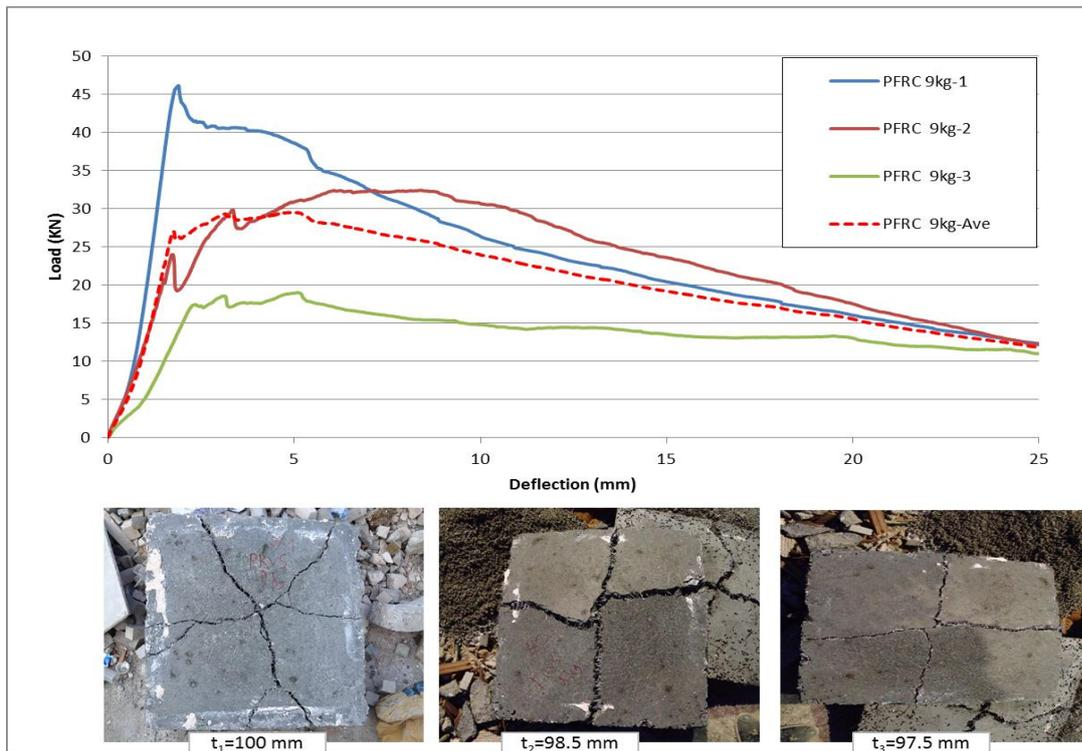
Figure 4.11 Load deflection curves and crack formations of PFRC 9kg samples with square panel test for 28 days.
