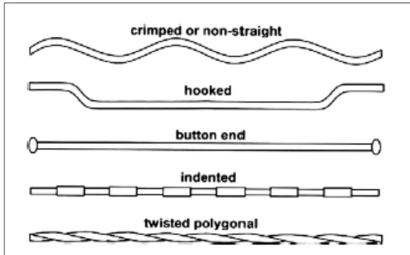
Figure 2.1 Some steel fiber types (Brant, 2008).
