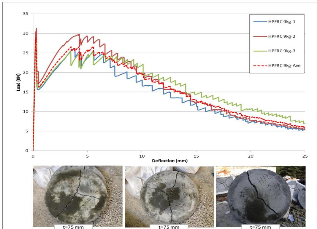
Figure 4.17 Load deflection curves and crack formations of HPFRC 9 kg samples with round panel test for 28 days.
