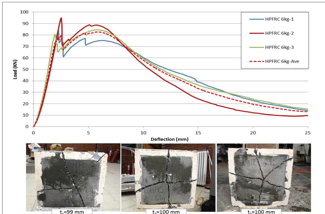
Figure 4.4 Load deflection curves and crack formations of HPFRC 6 kg samples with square panel test for 28 days.
