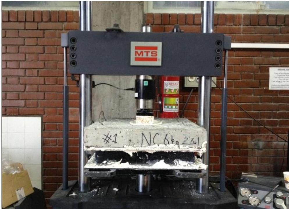
Figure 3.7 Set-up for square panel tests
