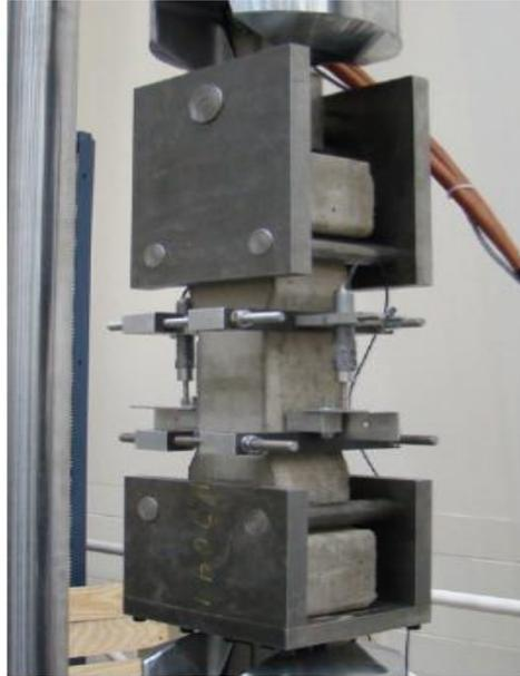
Figure 2.14 Uniaxial direct tensile testing settings (Chao et al., 2011).
