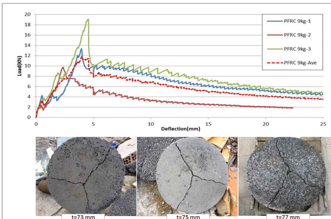
Figure 4.23 Load deflection curves and crack formations of PFRC 9kg samples with round panel test for 28 days.
