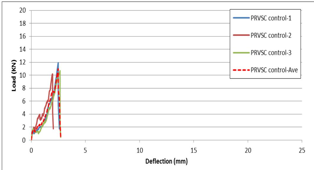
Figure 4.20 Load deflection curves of PRVSC Control samples with round panel test for 28 days.
