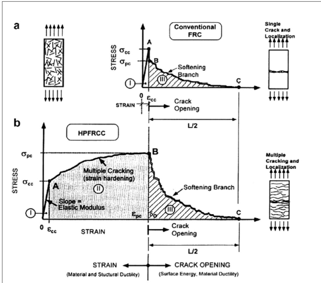
Figure 2.7 Strain hardening and strain softening behavior of HPFRCC and FRC (Brandt, 2008)
