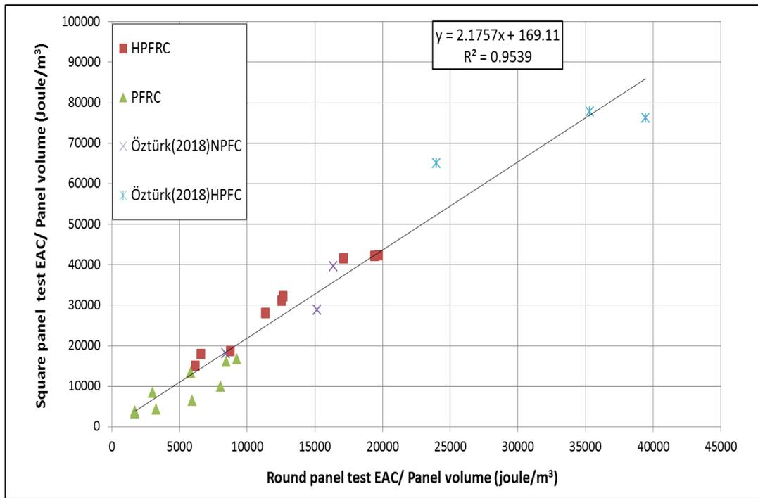
Figure 4.30 Correlation between round panel test and square panel test
