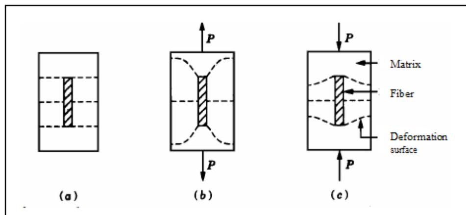
Figure 2.3 Interaction between non-cracked matrix and fiber a) unloaded b) tension forces c) compression forces (Shah and Balaguru, 1992).
