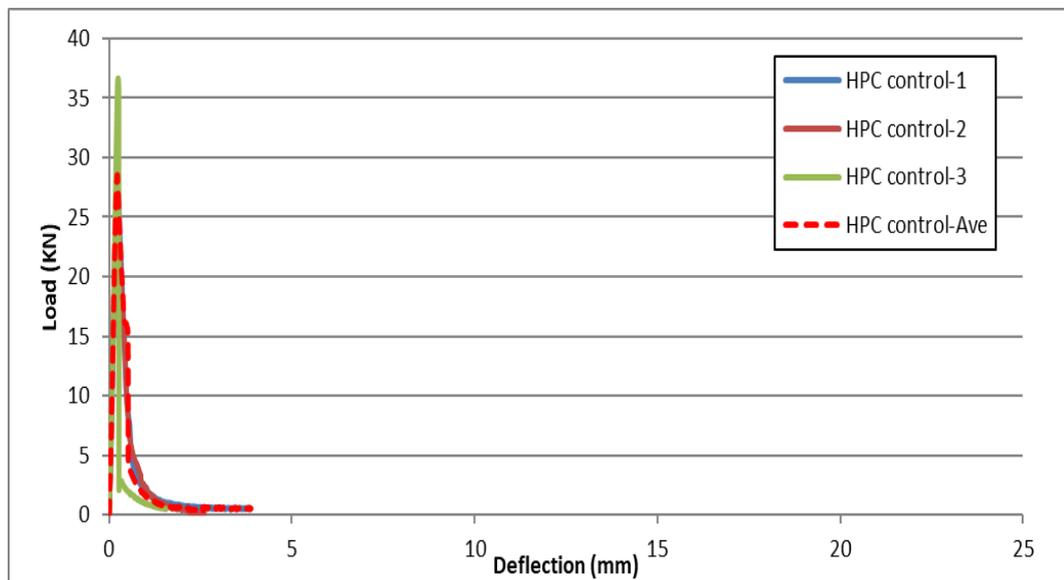
Figure 4.14 Load deflection curves of HPC control samples with round panel test for 28 days.
