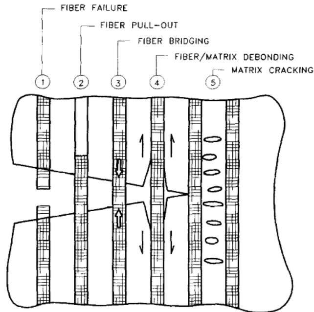
Figure 2.5 Fiber and matrix mechanism (Zollo, 1997).
