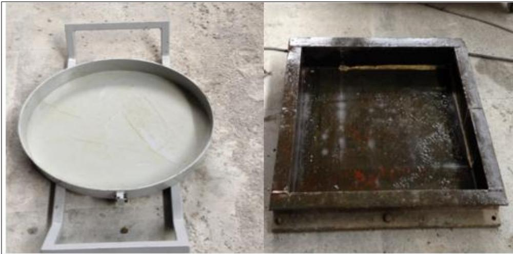
Figure 3.4 Round and square panel molds
