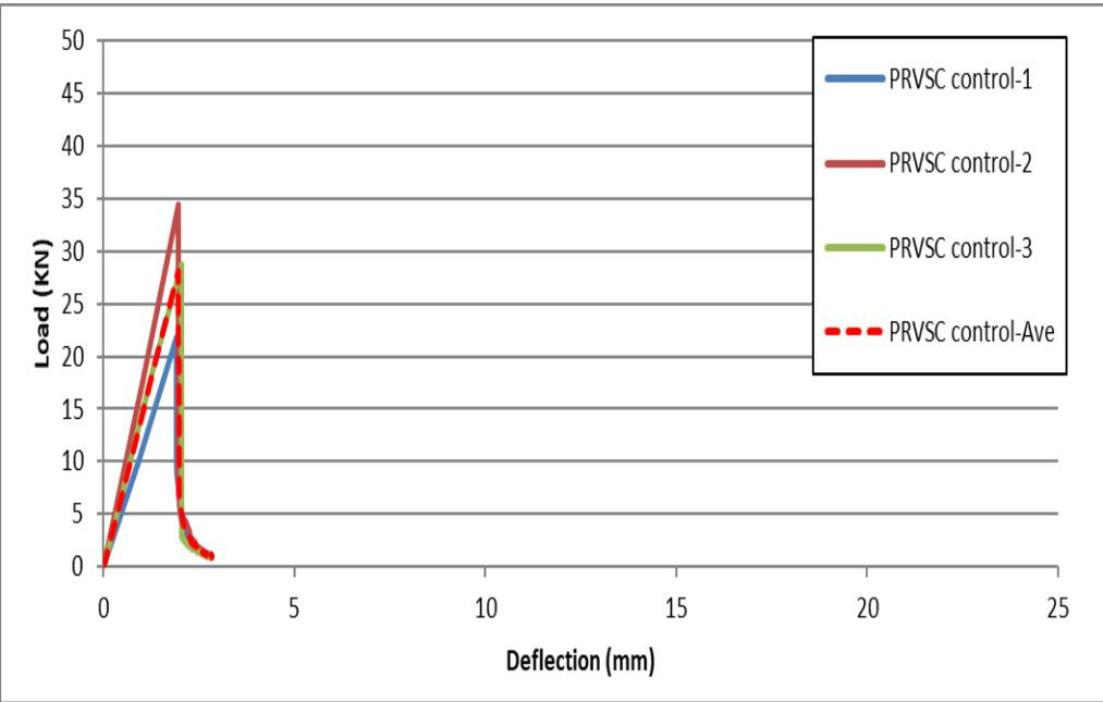
Figure 4.8 Load deflection curves of PRVSC Control samples with square panel test for 28 days.
