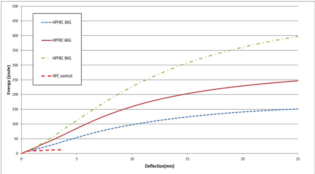
Figure 4.19 Comparison of energy deflection curves of HPFRC mixes with round panel test for 28 days.
