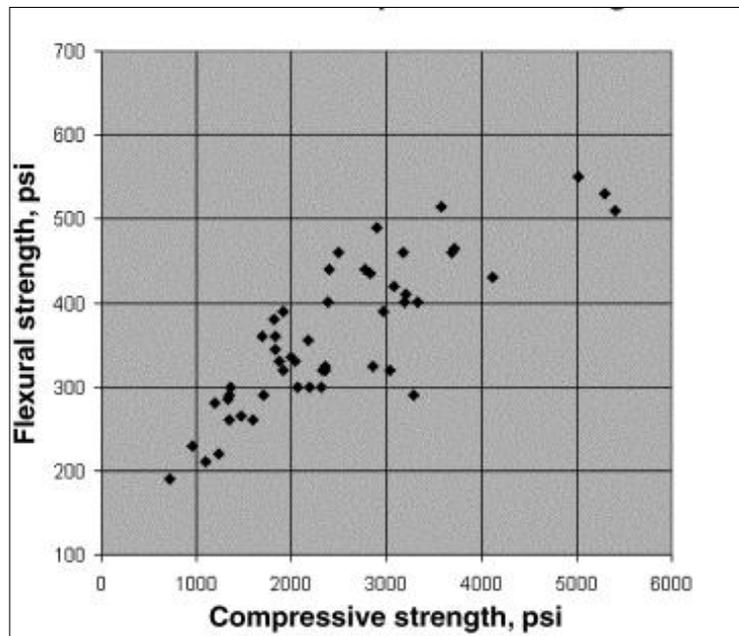
Figure 2.10 Relationship of compressive strength and flexural strength in pervious concrete (ACI Committee 522, 2006).
