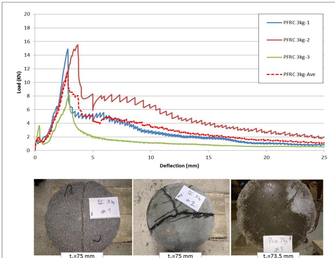
Figure 4.21 Load deflection curves and crack formations of PFRC 3kg samples with round panel test for 28 days.
