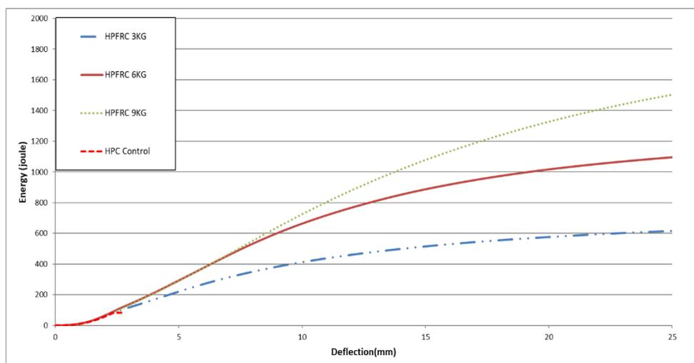
Figure 4.7 Comparison of energy deflection curves of HPFRC mixes with square panel test for 28 days.
