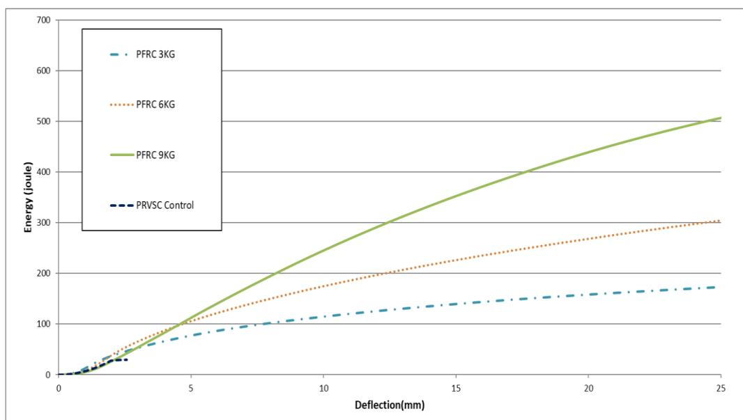
Figure 4.13 Comparison of energy deflection curves of PFRC mixes with square panel test for 28 days.
