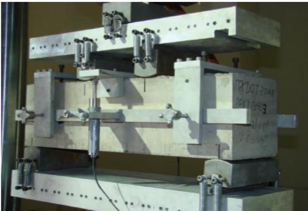
Figure 2.12 Setup for ASTM C1609 test (Chao et al., 2011).
