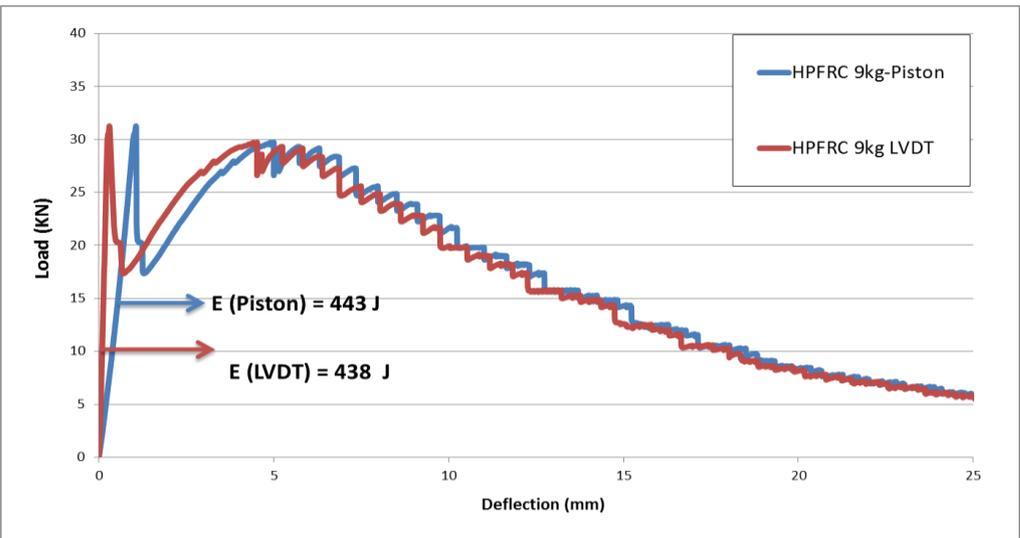
Figure 4.28 Load-deflection curves obtained from piston and LVDT
