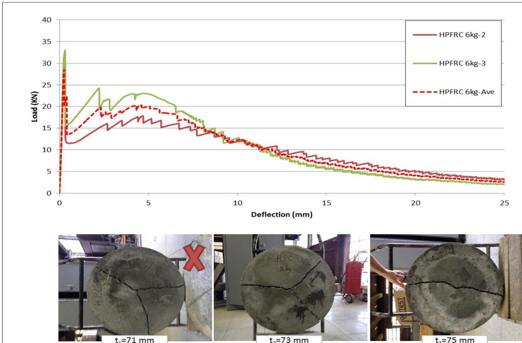
Figure 4.16 Load deflection curves and crack formations of HPFRC 6 kg samples with round panel test for 28 days.
