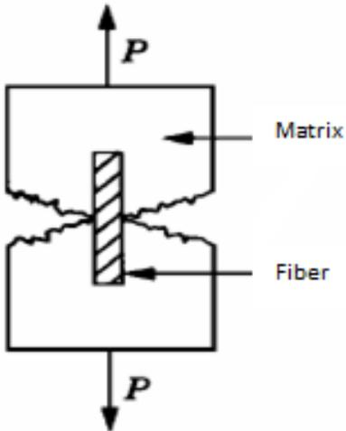
Figure 2.4 Cracked matrix-fiber relations (Shah and Balaguru, 1992).
