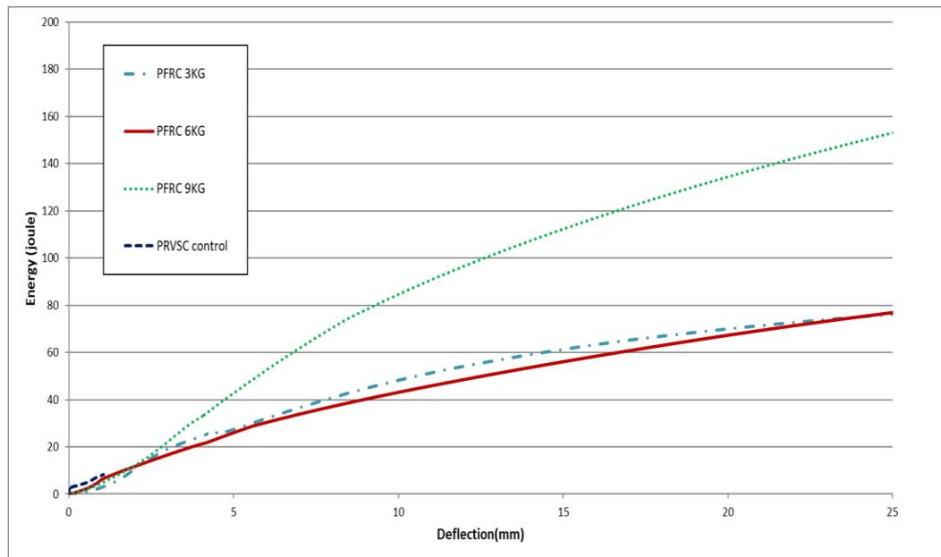
Figure 4.25 Comparison of energy deflection curves of PFRC mixes with round panel test for 28 days.
