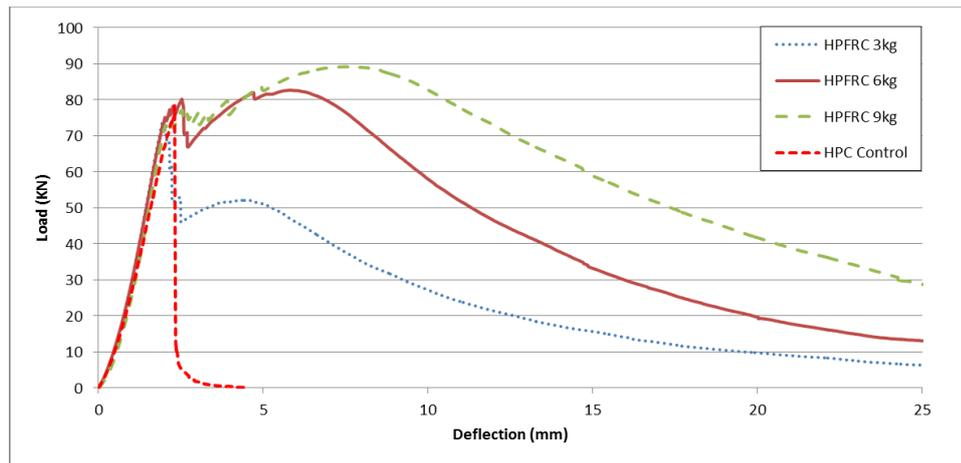
Figure 4.6 Comparison of load deflection curves of HPFRC mixes with square panel test for 28 days.
