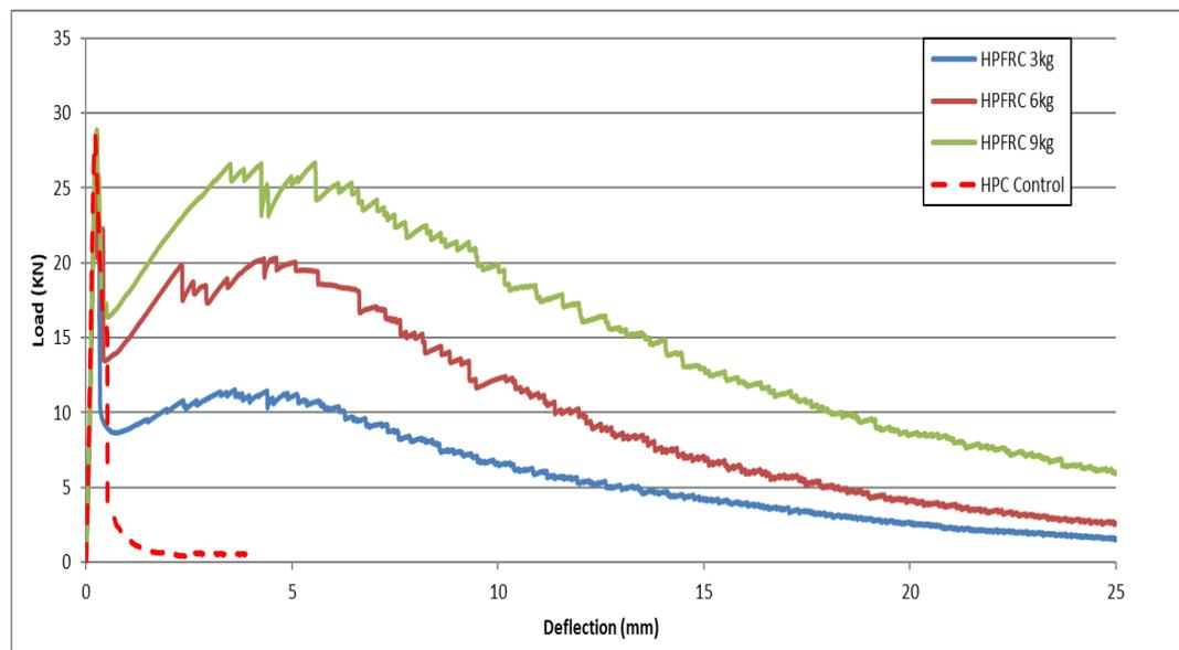
Figure 4.18 Comparison of load deflection curves of HPFRC mixes with round panel test for 28 days.
