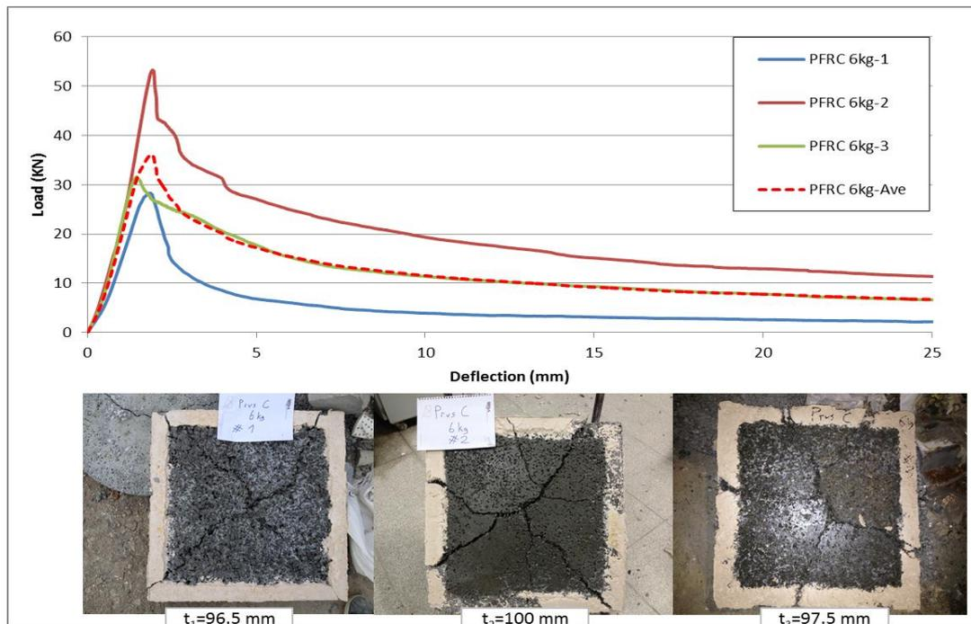
Figure 4.10 Load deflection curves and crack formations of PFRC 6kg samples with square panel test for 28 days.
