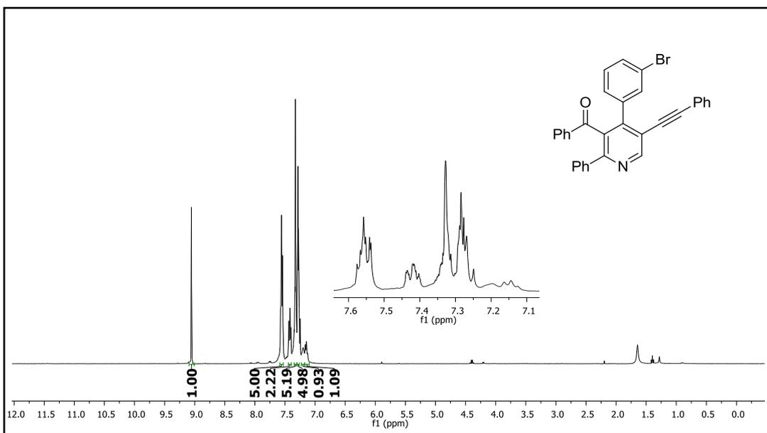
Figure 268.  $^1\text{H}$  NMR spectrum of compound **57aba**.
