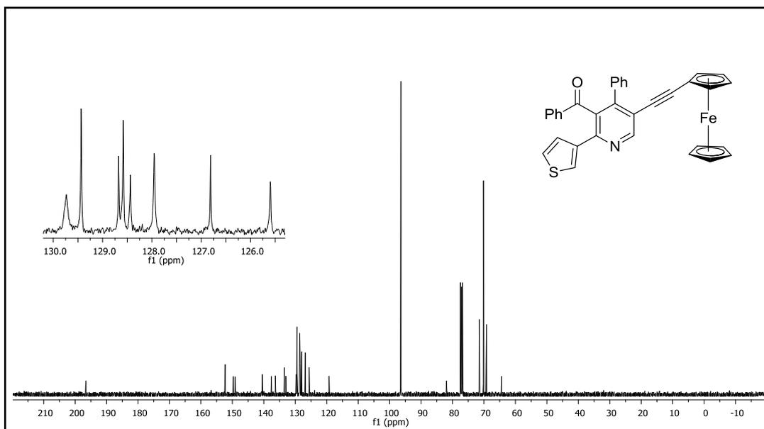
**Figure 265.**  $^{13}\text{C}$  NMR spectrum of compound **57mr**.
