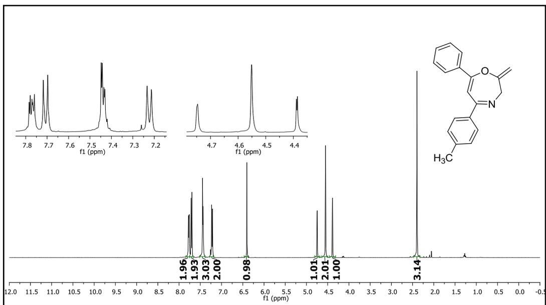
Figure 278.  $^1\text{H}$  NMR spectrum of compound 33d.
