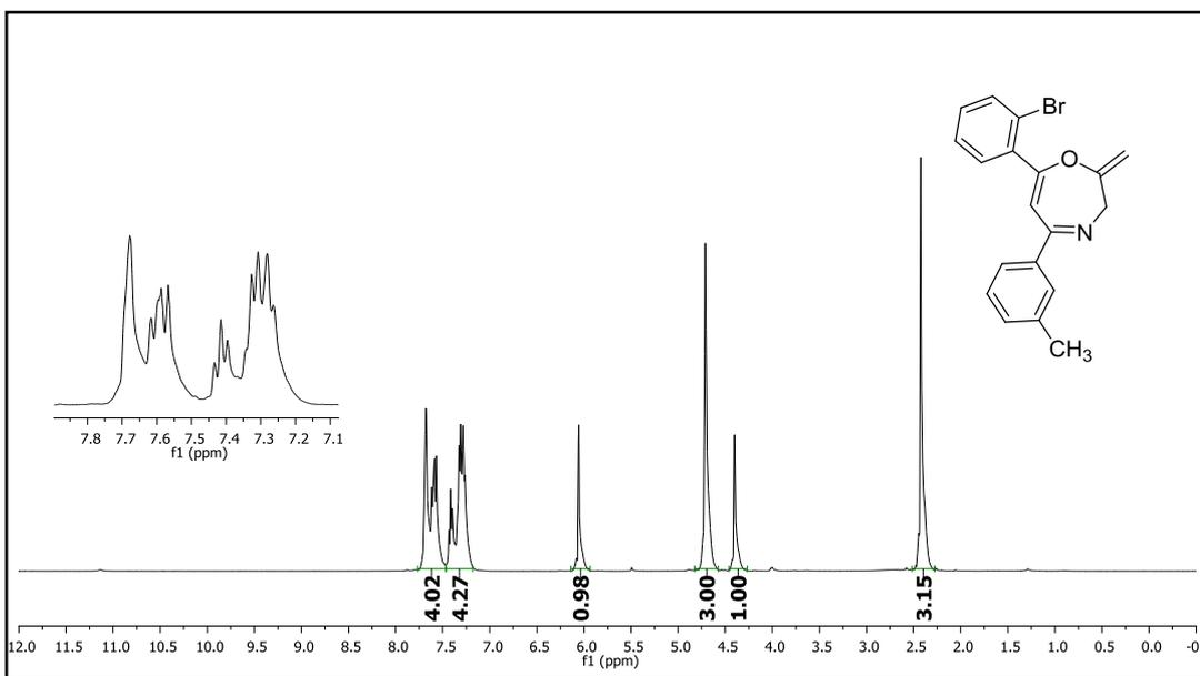
**Figure 304.**  $^1\text{H}$  NMR spectrum of compound 33r.
