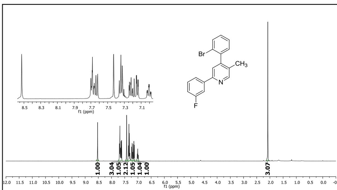
**Figure 398.**  $^1\text{H}$  NMR spectrum of compound **61t**.
