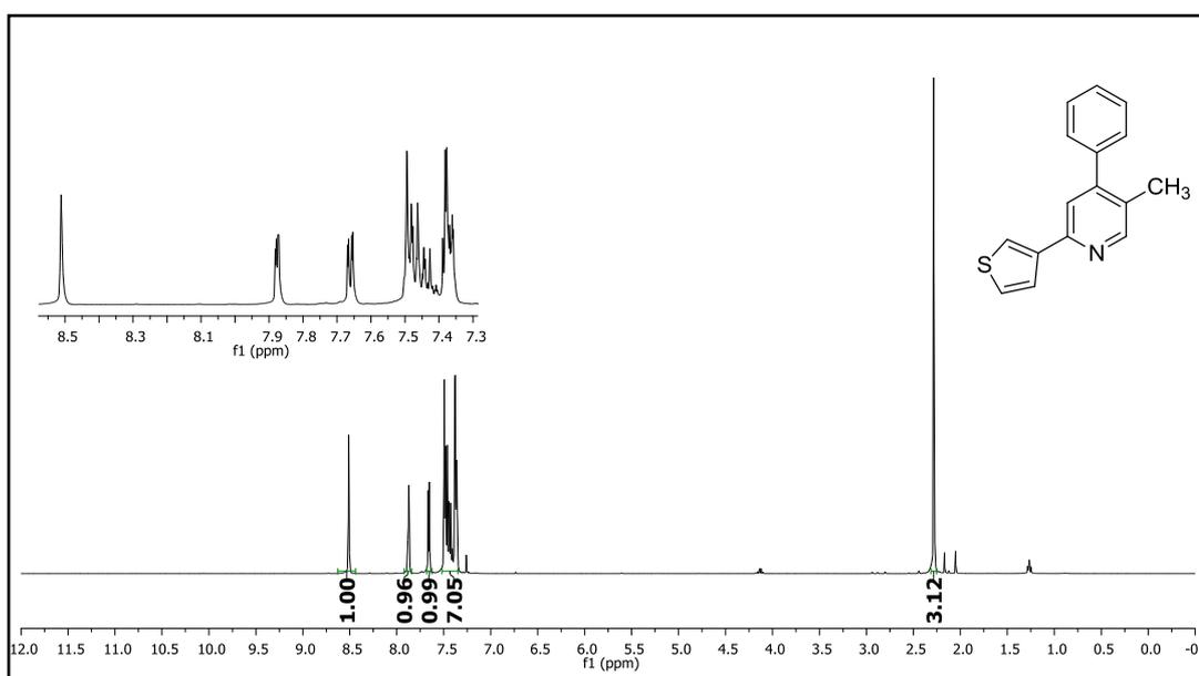
Figure 390.  $^1\text{H}$  NMR spectrum of compound 61m.
