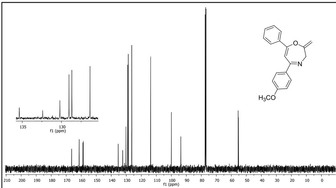
Figure 275.  $^{13}\text{C}$  NMR spectrum of compound 33b.
