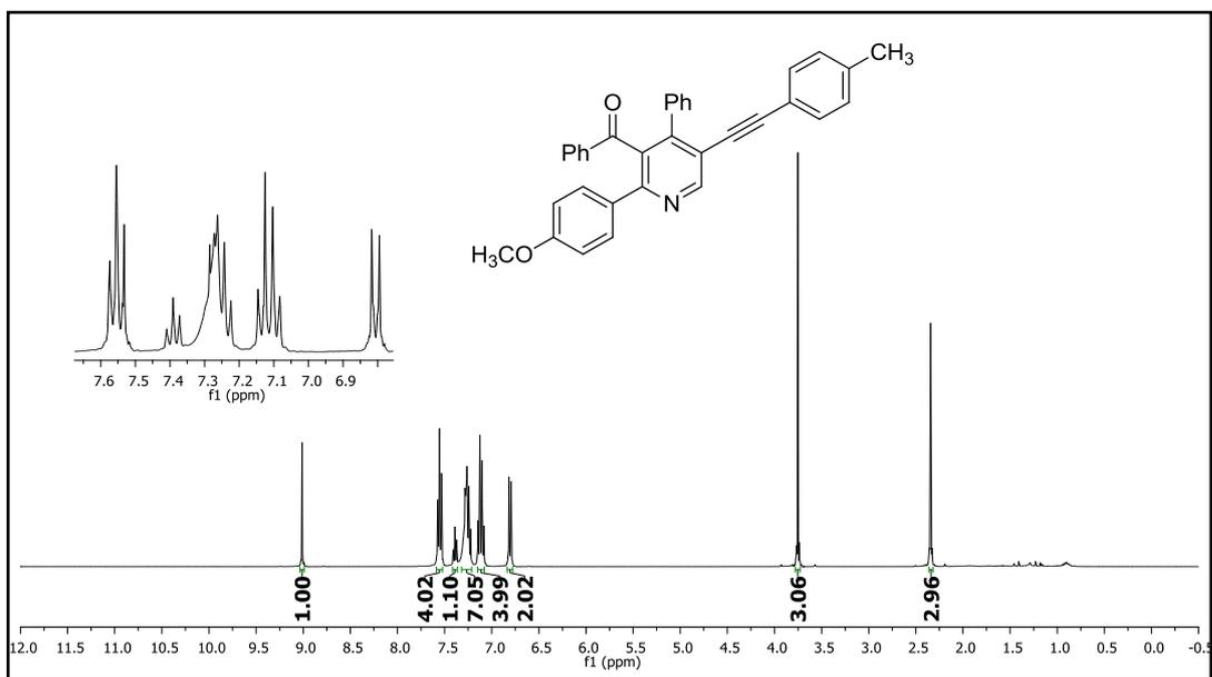
**Figure 250.**  $^1\text{H}$  NMR spectrum of compound **57bd**.
