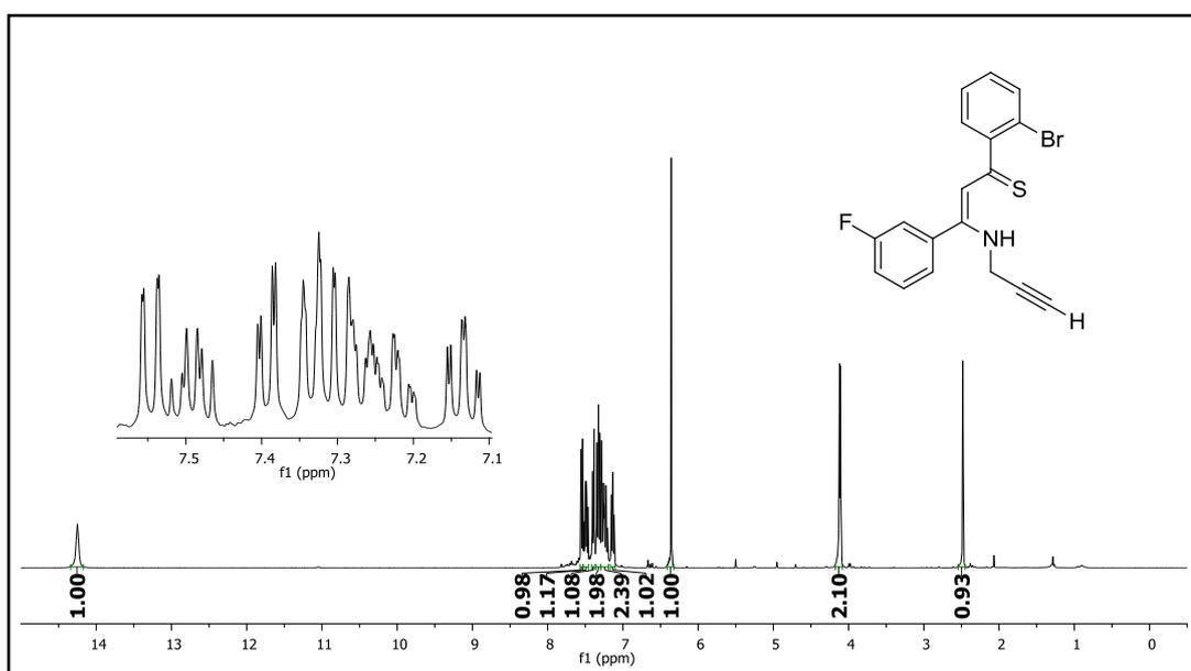
**Figure 200.**  $^1\text{H}$  NMR spectrum of compound 58t.
