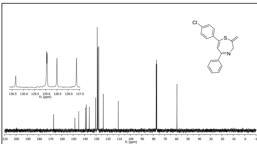
**Figure 358.**  $^{13}\text{C}$  NMR spectrum of compound **59y**.
