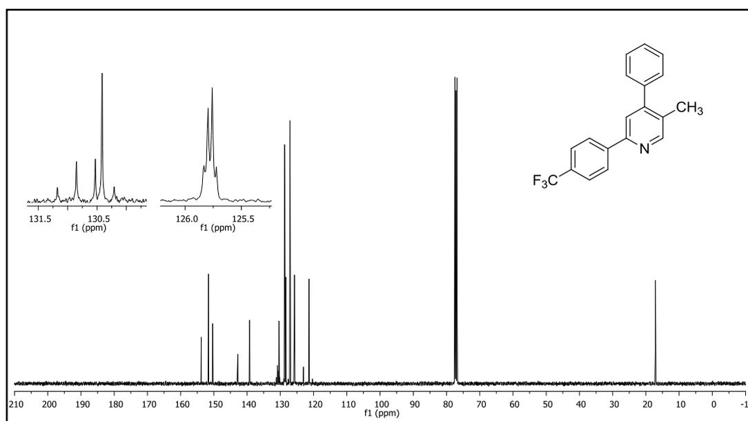
**Figure 382.**  $^{13}\text{C}$  NMR spectrum of compound **61f**.
