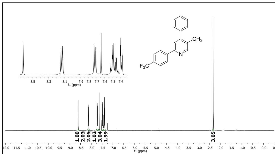
**Figure 381.**  $^1\text{H}$  NMR spectrum of compound **61f**.
