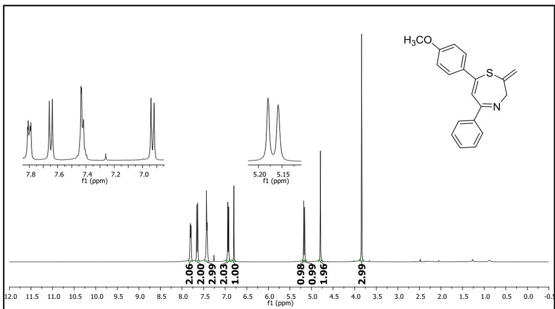
**Figure 351.**  $^1\text{H}$  NMR spectrum of compound **59v**.
