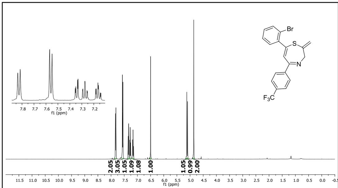
Figure 347.  $^1\text{H}$  NMR spectrum of compound **59s**.
