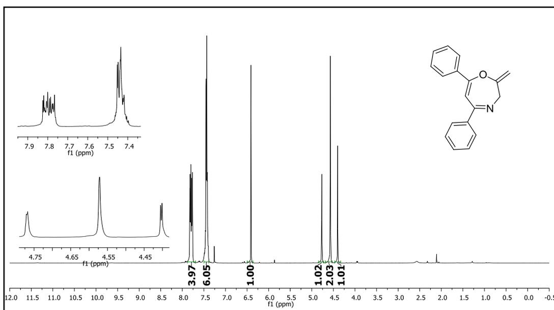
**Figure 272.**  $^1\text{H}$  NMR spectrum of compound **33a**.
