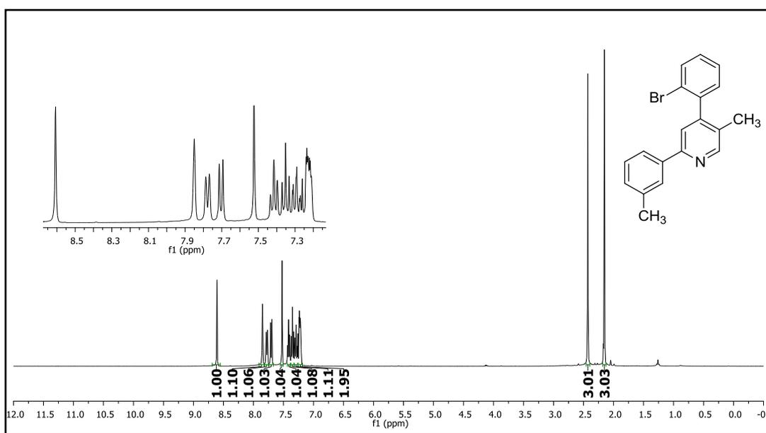
Figure 394.  $^1\text{H}$  NMR spectrum of compound 61r.
