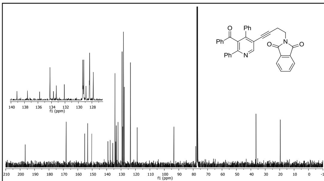
**Figure 231.**  $^{13}\text{C}$  NMR spectrum of compound **57k**.
