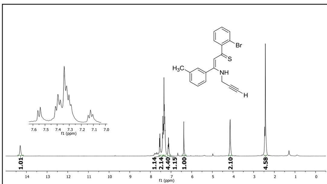
**Figure 196.**  $^1\text{H}$  NMR spectrum of compound **58r**.
