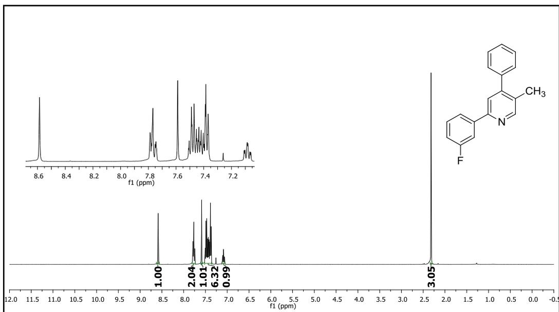
Figure 383. <sup>1</sup>H NMR spectrum of compound 61h.
