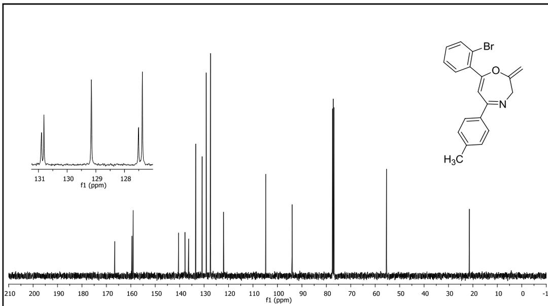
**Figure 303.**  $^{13}\text{C}$  NMR spectrum of compound 33q.
