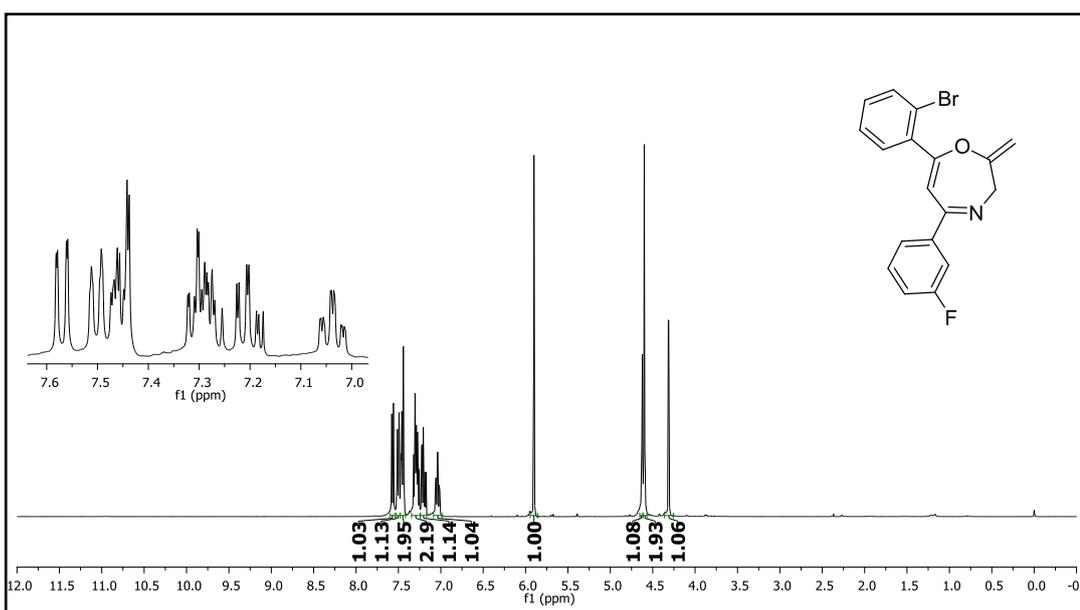
**Figure 308.**  $^1\text{H}$  NMR spectrum of compound **33t**.
