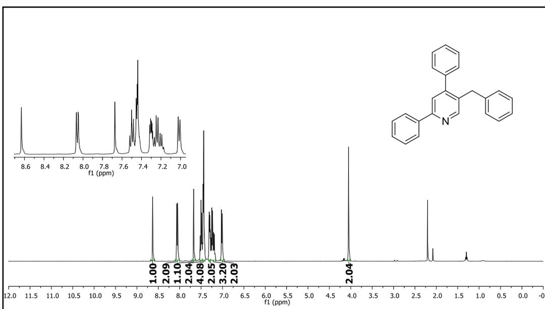
Figure 410.  $^1\text{H}$  NMR spectrum of compound **89**.
