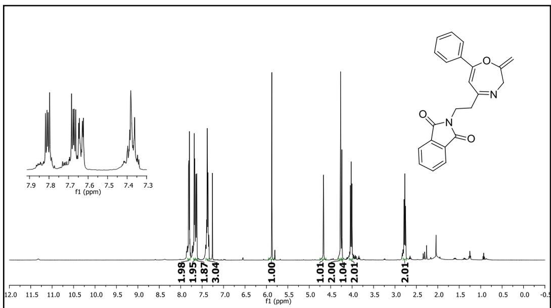
Figure 290.  $^1\text{H}$  NMR spectrum of compound 33k.
