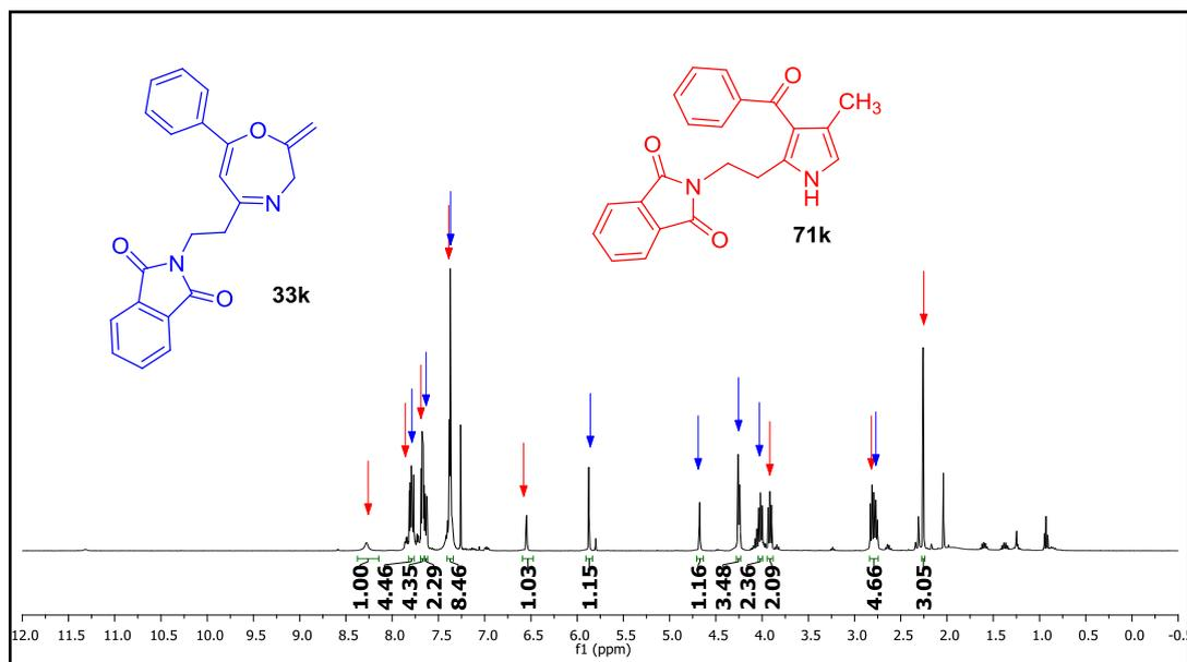
**Figure 316.**  $^1\text{H}$  NMR spectrum of a mixture of compounds **33k** and **71k** with a ratio of 1.15:1.00, respectively.
