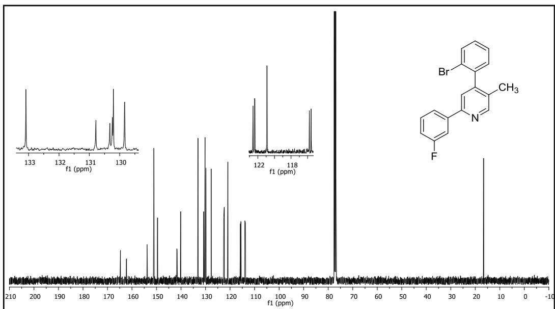
Figure 399.  $^{13}\text{C}$  NMR spectrum of compound **61t**.
