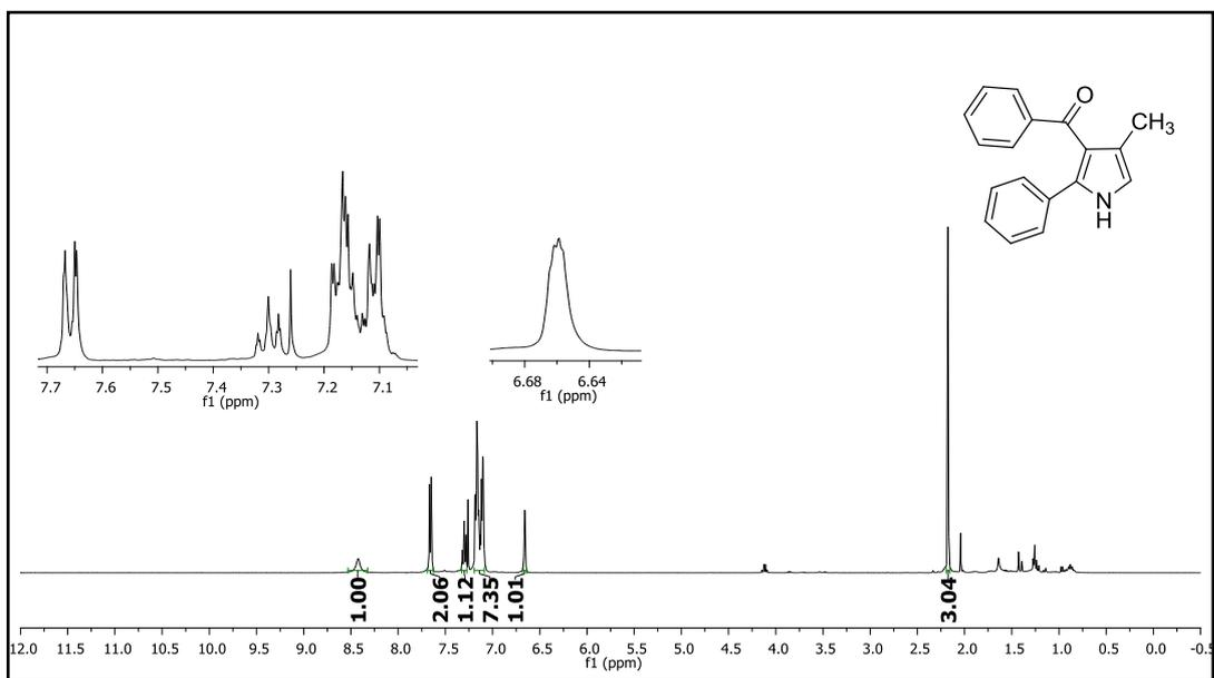
**Figure 314.**  $^1\text{H}$  NMR spectrum of compound **71a**.
