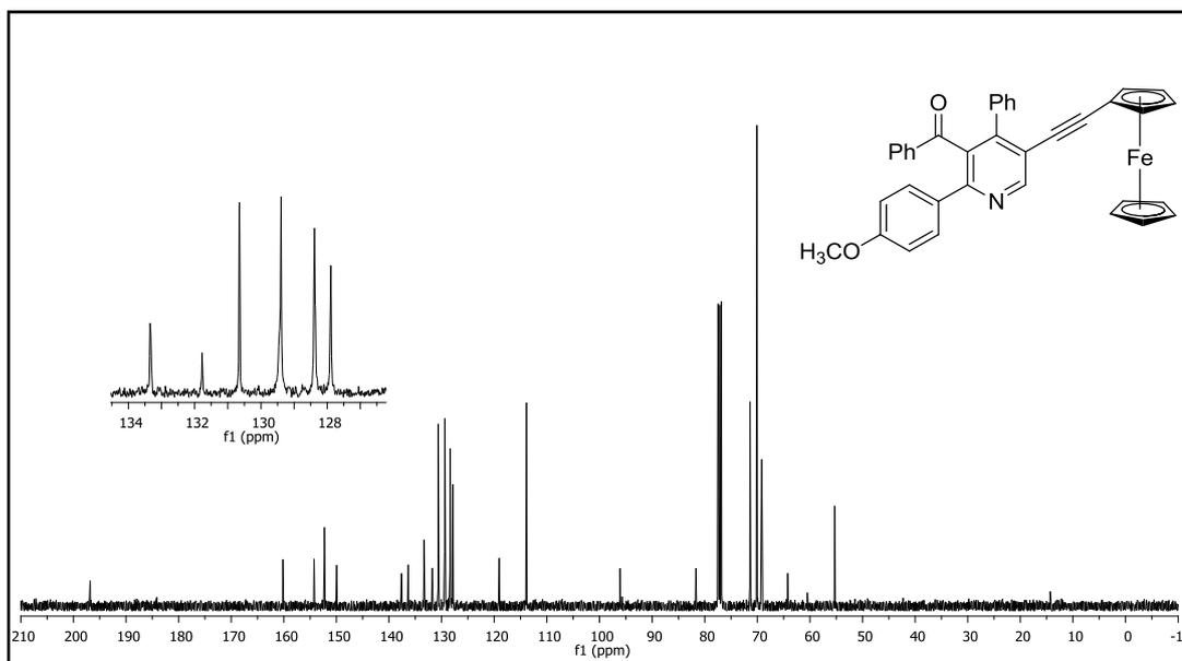
**Figure 255.**  $^{13}\text{C}$  NMR spectrum of compound **57br**.
