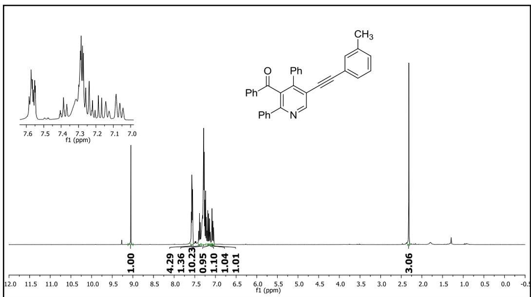
Figure 222.  $^1\text{H}$  NMR spectrum of compound 57e.
