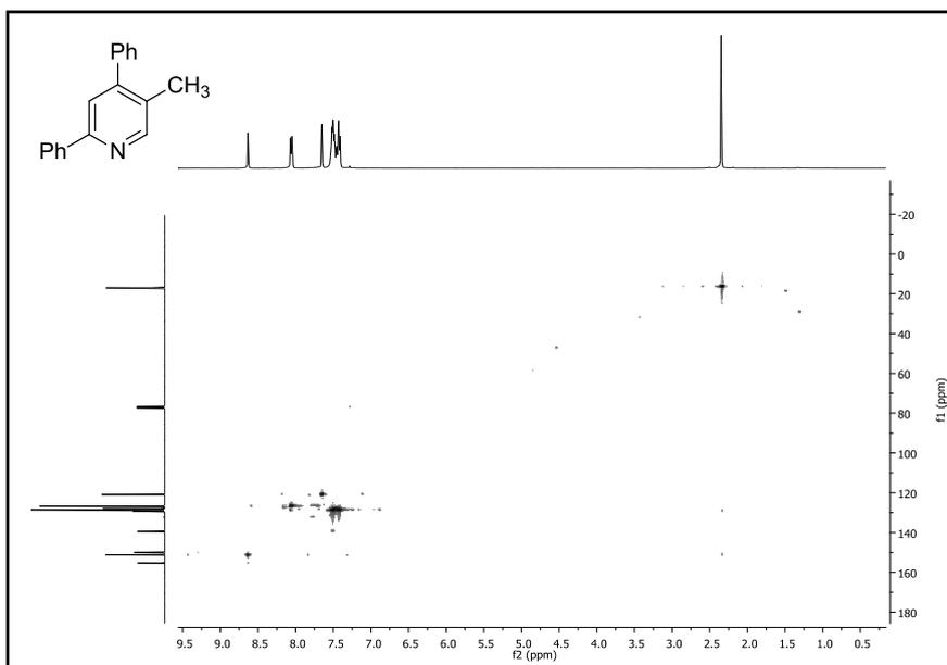
**Figure 371.** HSQC NMR spectrum of compound **61a**.
