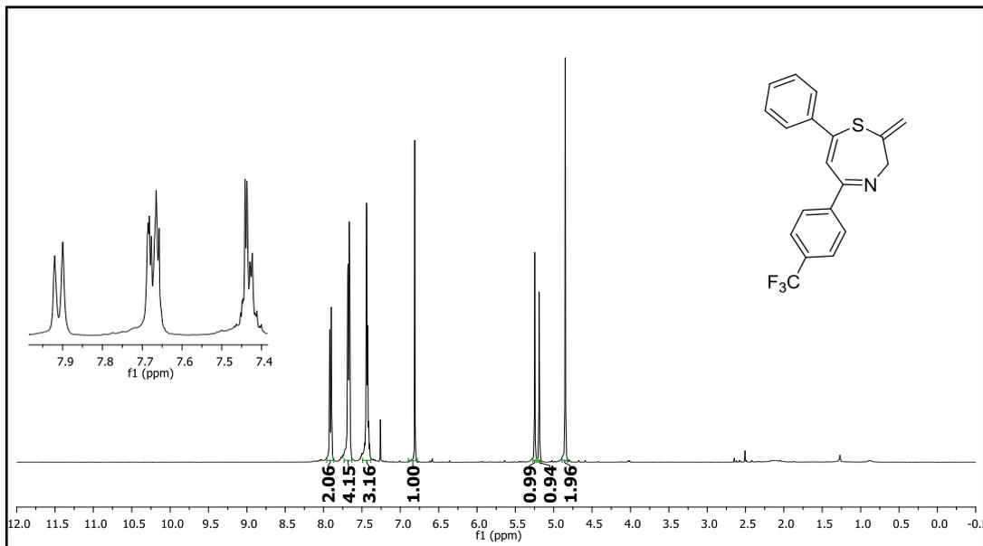
Figure 331.  $^1\text{H}$  NMR spectrum of compound **59f**.
