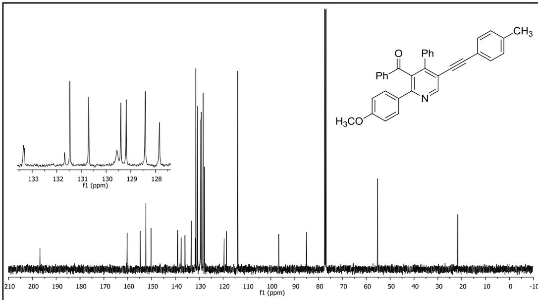
**Figure 251.**  $^{13}\text{C}$  NMR spectrum of compound **57bd**.
