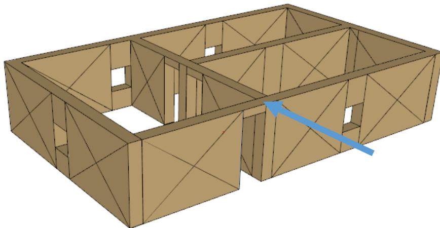
Figure A - 6 Earthquake force perpendicular to house
