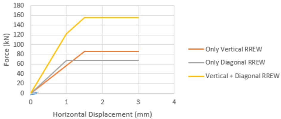
Figure A - 3 Wall failure predictions according to reinforcements
