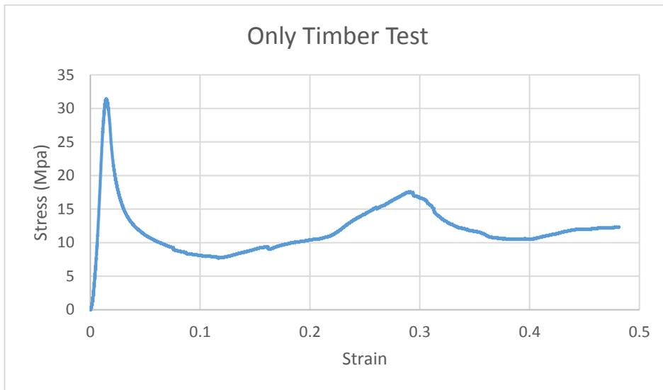
Figure 3.17 Wooden confinement element test results
