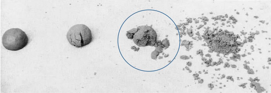
Figure 2.17 Drop test [16]
