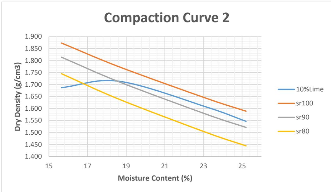
Figure 3.4 Compaction curve of 2nd mixture
