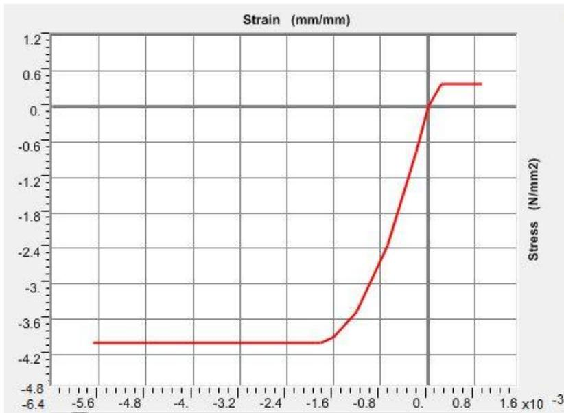
Figure 4.10 Earthen material properties
