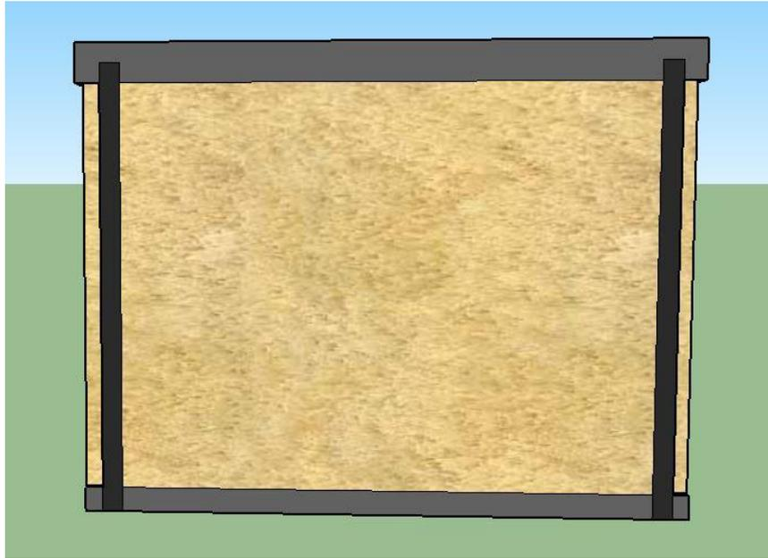
Figure 2.35 REW with vertical reinforcement
