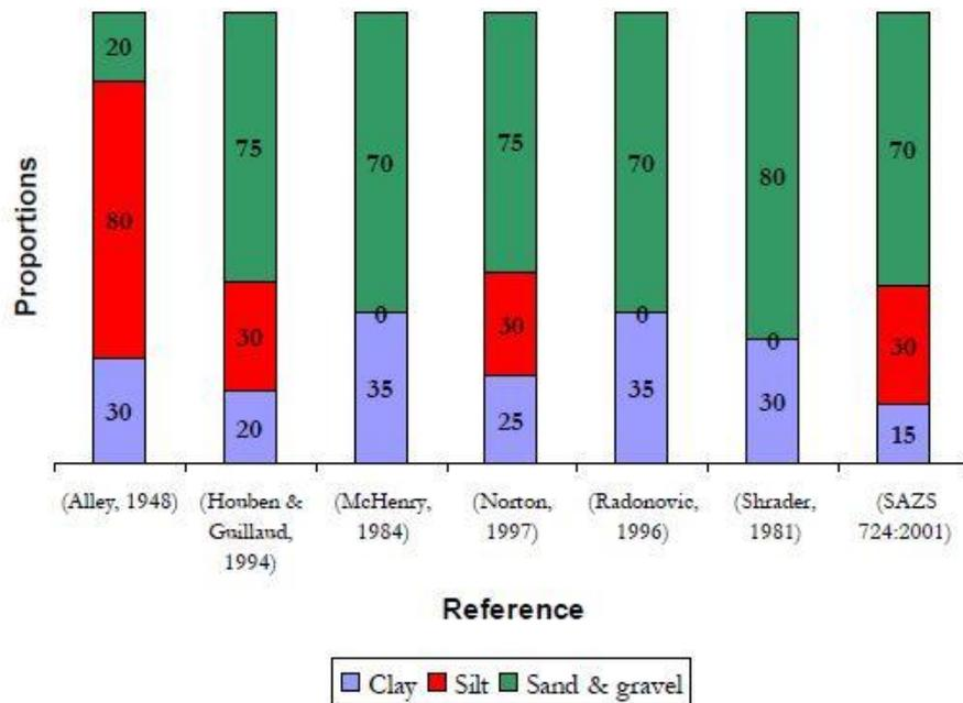
Figure 2.3 Upper limits of the mixing composition [12]
