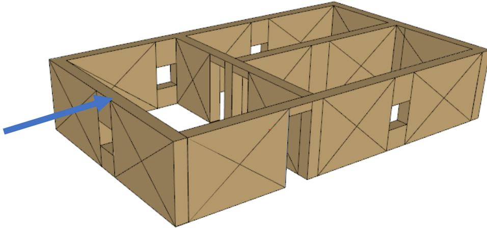
Figure A - 5 Earthquake force parallel to house
