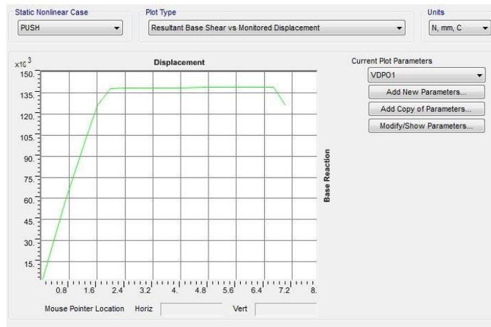
Figure 4.16 Pushover curve of the third wall's final test
