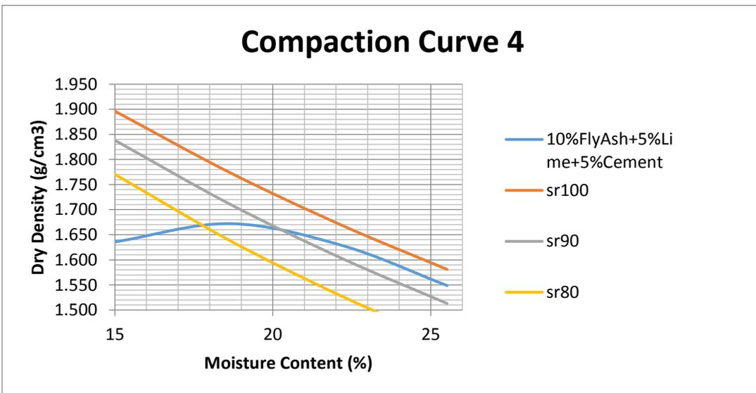
Figure 3.6 Compaction curve of 4th mixture
