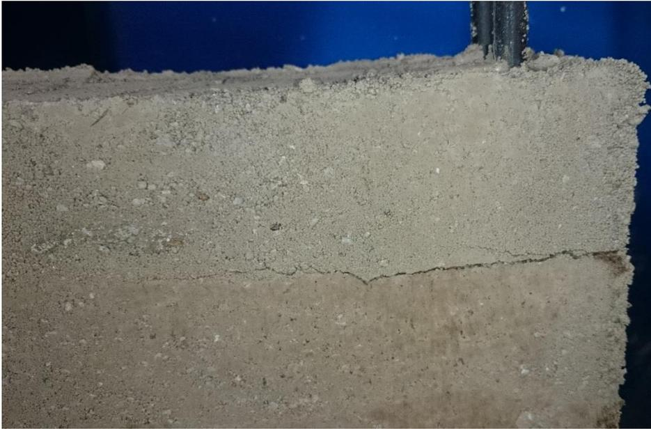
Figure 3.34 Shrinkage cracks
