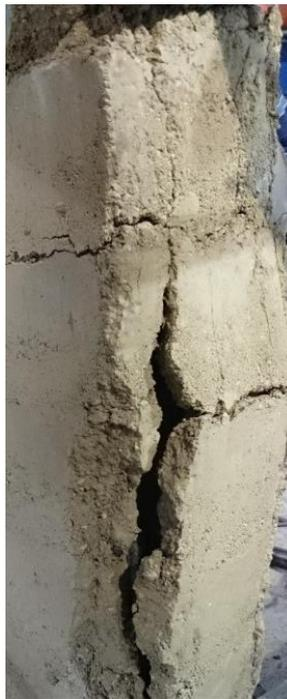
Figure 3.36 Expansion of the cracks at side
