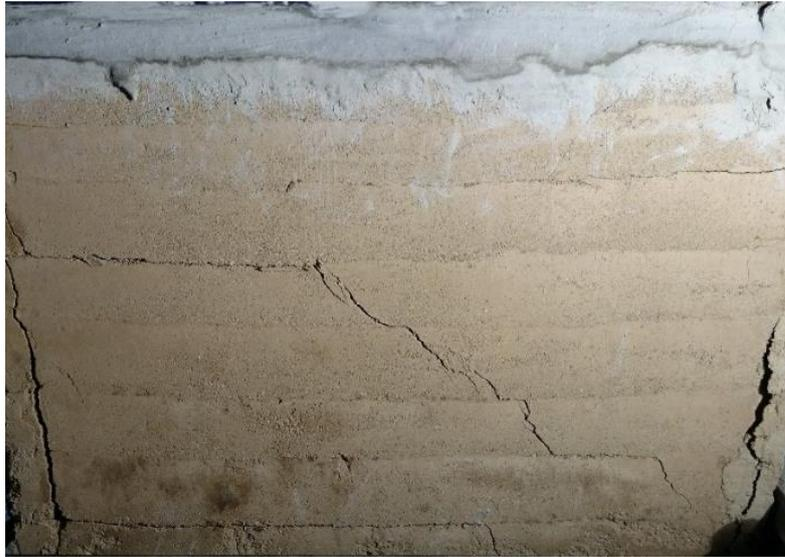
Figure 3.35 1st failure of RREW
