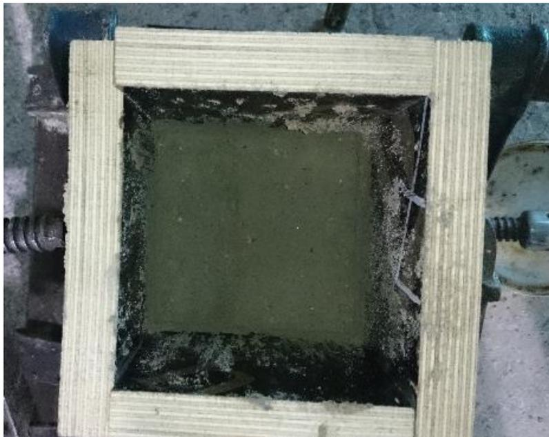
Figure 2.12 Ramming process (top of the specimen and formwork)
