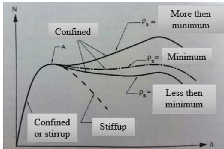
Figure 3.20 Reinforced and confined column behavior graph [29]
