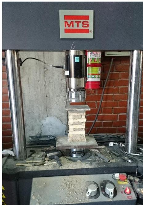
Figure 3.11 Wooden confinement column test
