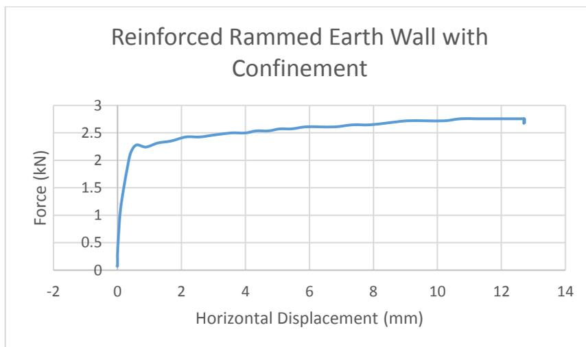
Figure 3.44 Test 3.1 - results of confinement reinforced REW
