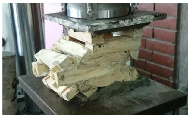
Figure 3.16 Wooden confinement element's deformation
