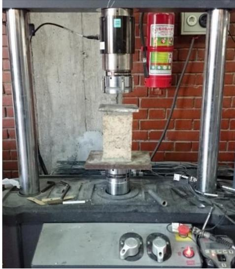
Figure 3.21 Steel hoop confinement column test
