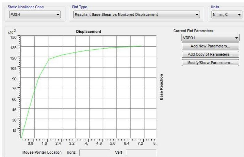
Figure 4.15 Pushover curve of the second wall's final test
