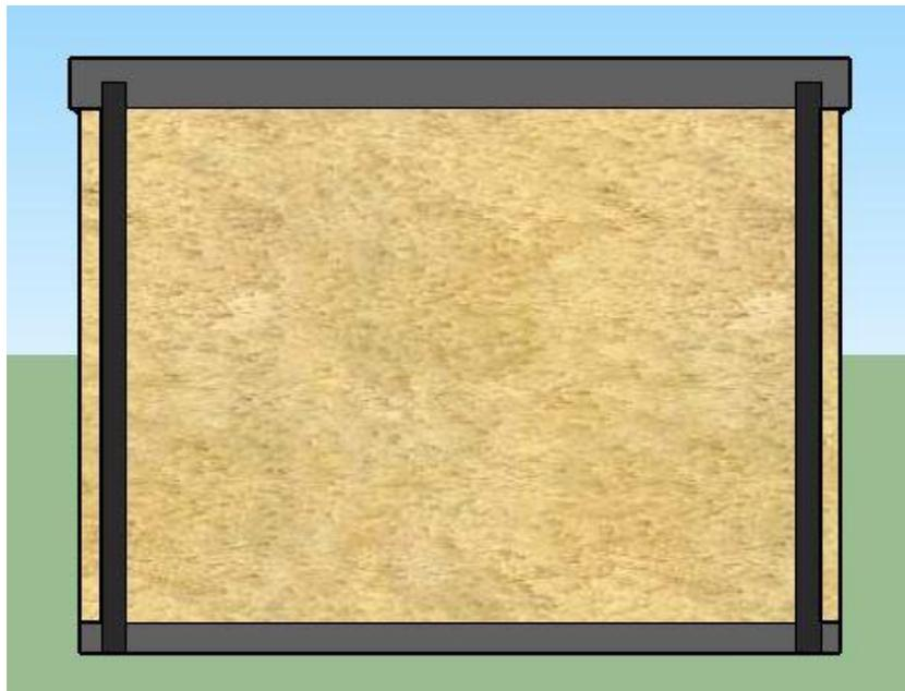
Figure 2.7 REW with vertical reinforcement
