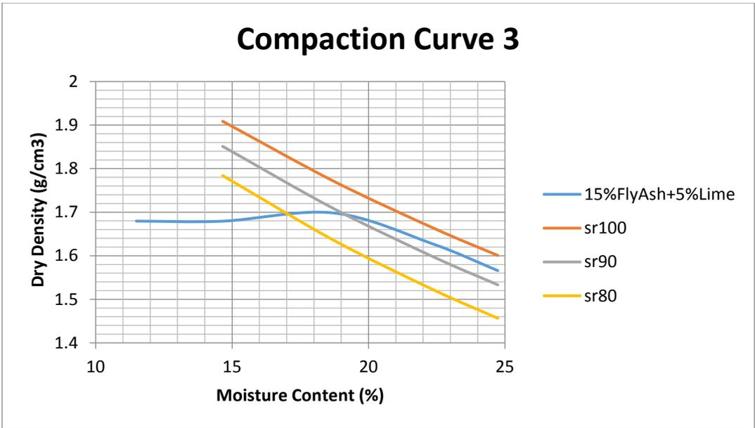
Figure 3.5 Compaction curve of 3rd mixture
