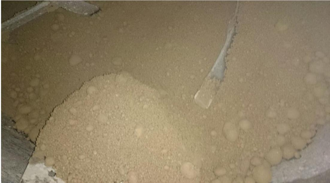
Figure 2.16 Floc balls in the mixture
