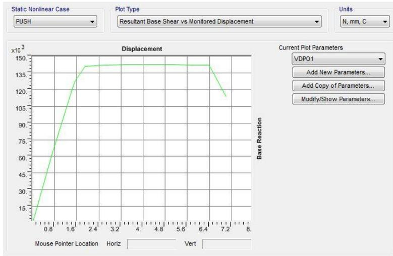
Figure 4.14 Pushover curve of the first wall's final test
