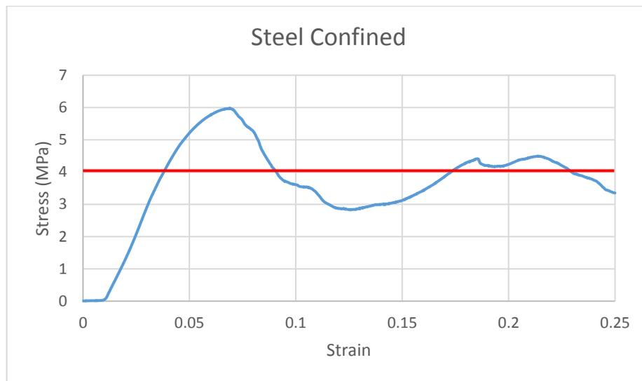
Figure 3.24 Steel hoop confined column test results
