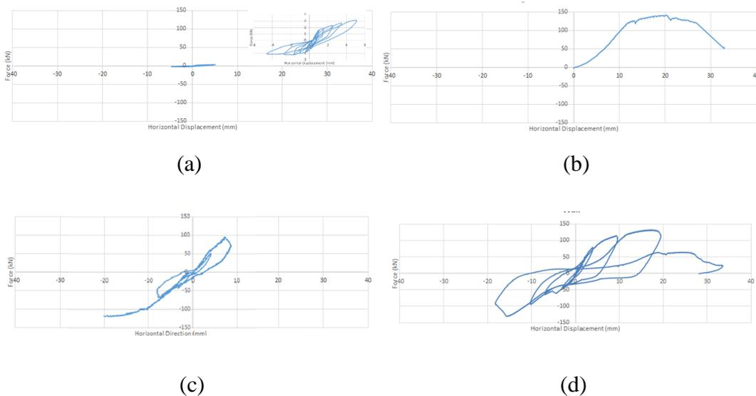
Figure 5.1 Same scale test results a) UrREW, b) 1<sup>st</sup> RREW, c) 2<sup>nd</sup> RREW, d) 3<sup>rd</sup> RREW
