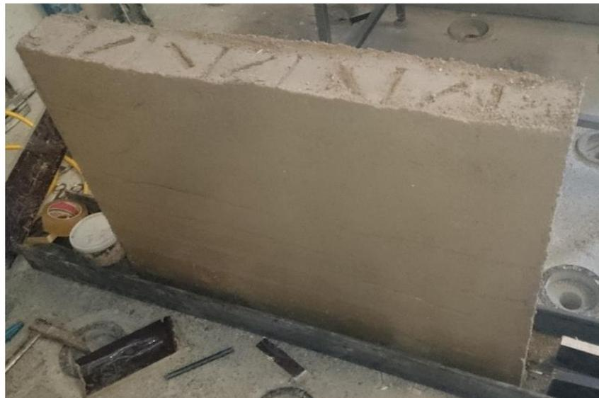
Figure 2.32 REW after formworks were removed
