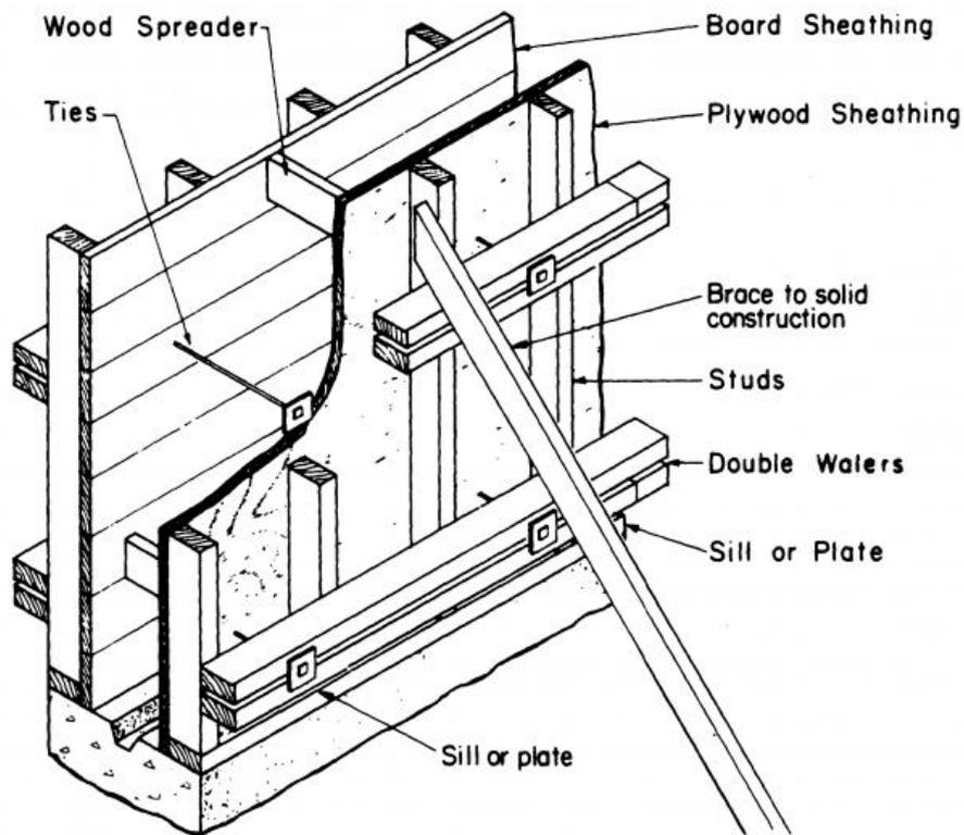
Figure 2.22 Example of sheathing and stiffening elements (URL – 10)
