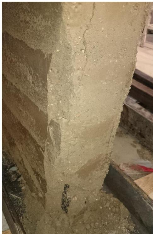
Figure 3.33 Cracks at the sides
