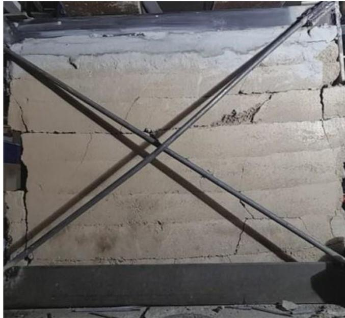
Figure 3.39 Expansion of the cracks at side
