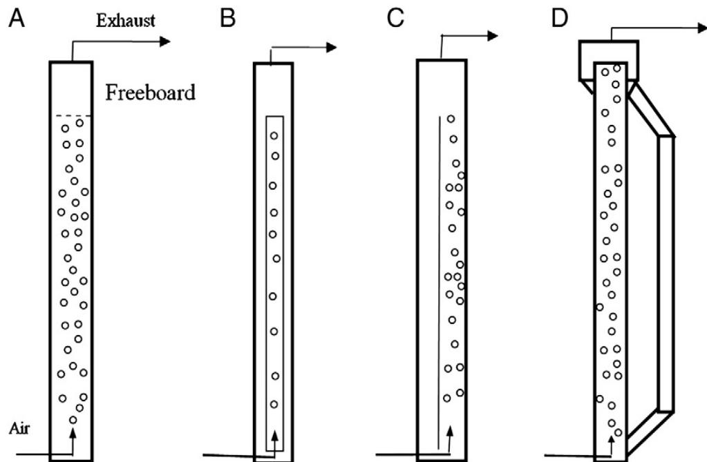
Figure 2-5 Schematic representation of different kinds of vertical column reactors:
