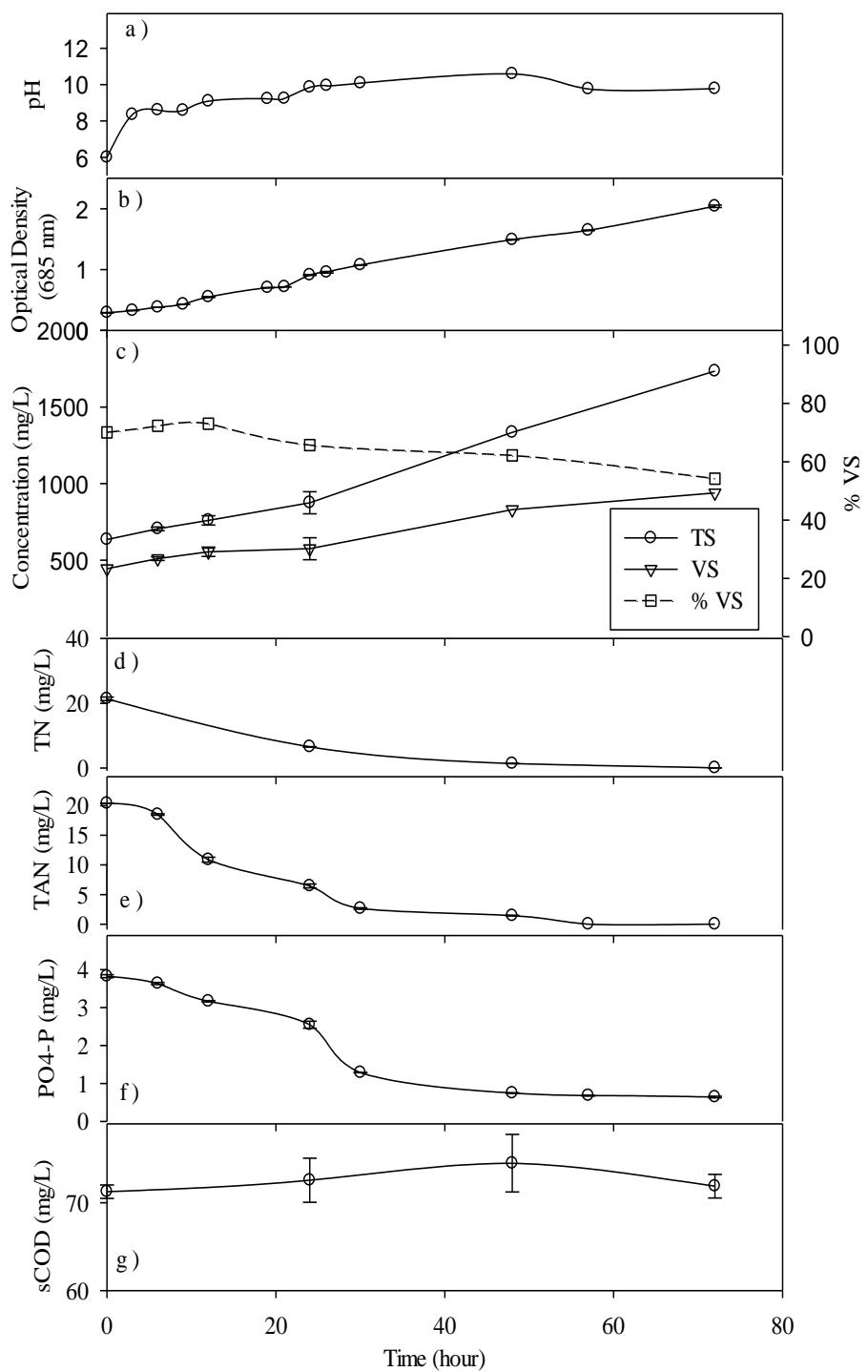
Figure 4-9 The change in parameters a) pH, b) Optical density, c) TS concentration, VS concentration, % VS, d) TN, e) TAN, f) PO<sub>4</sub>-P and g) sCOD in XB-1 reactor with respect to time
