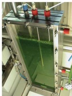
Figure 2-7 An example picture of flat plate PBR (Iersel et al., 2009)
