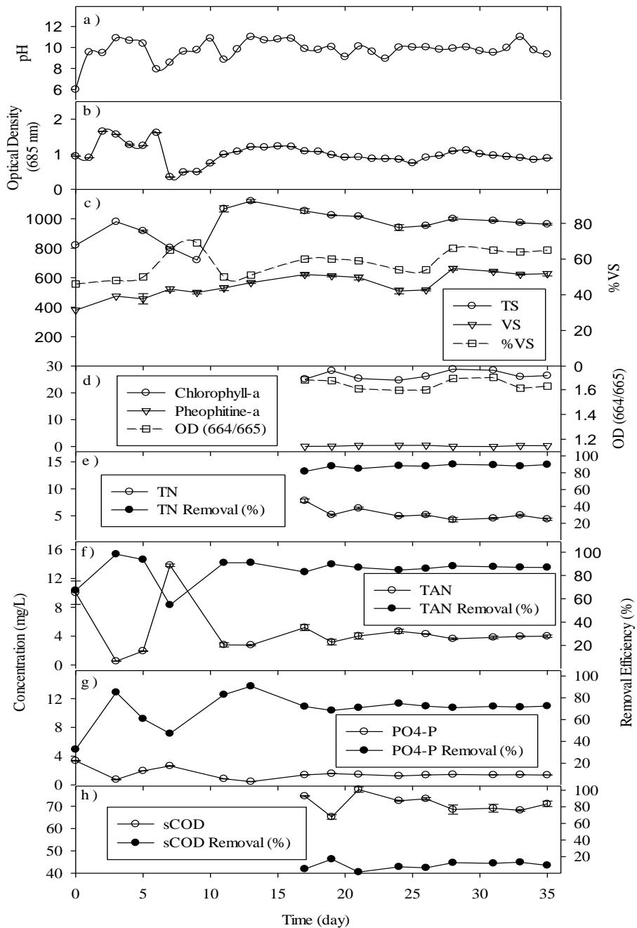
Figure 4-6 The change in parameters of X1 Reactor with respect to time; a) pH, b) Optical density, c) TS concentration, VS concentration, % VS, d) Chlorophyll-a, Pheophytin-a, OD (664<sub>b</sub>/665<sub>a</sub>), e) TN effluent concentration, TN removal efficiency, f) TAN effluent concentration, TAN removal efficiency, g) PO<sub>4</sub>-P effluent concentration, PO<sub>4</sub>-P removal efficiency, h) sCOD effluent concentration, sCOD removal efficiency.
