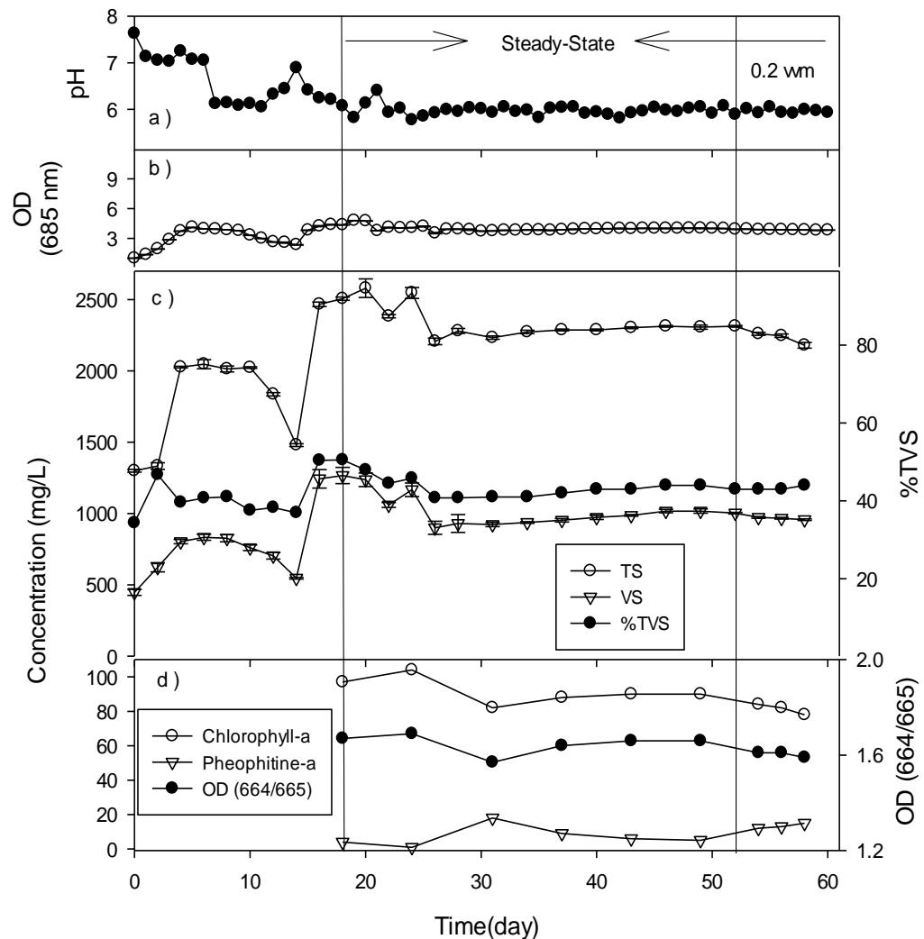
Figure 4-17 Change in parameters of C12 reactor with respect to time; a) pH, b) optical density at 685 nm, c) total solid concentration, volatile solid concentration, %TVS, d) Chlorophyll-a, Pheophytin-a, OD (664<sub>b</sub>/665<sub>a</sub>).
