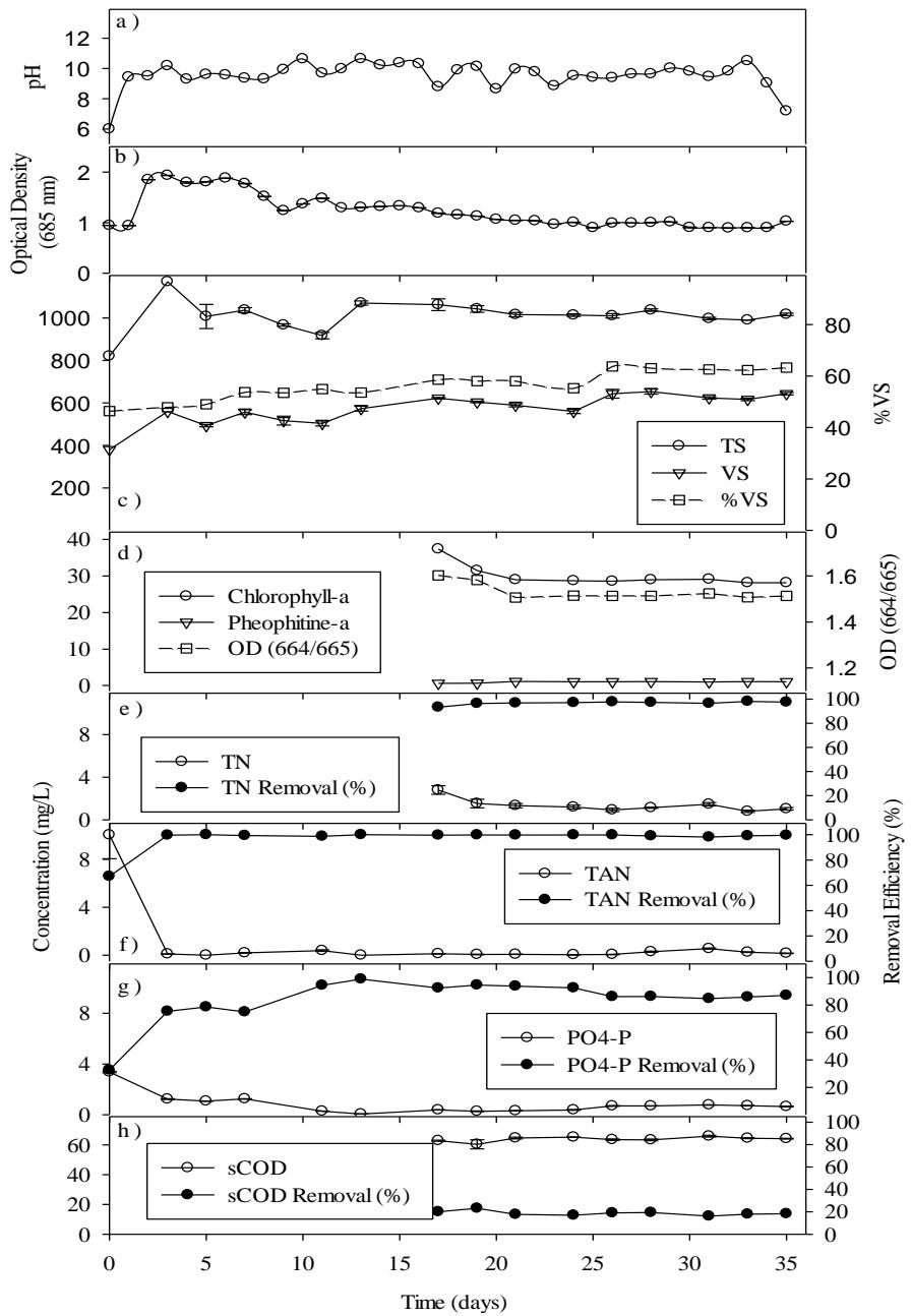
Figure 4-7 The change in parameters of X2 Reactor with respect to time; a) pH, b) Optical density, c) TS concentration, VS concentration, % VS, d) Chlorophyll-a, Pheophytine-a, OD (664<sub>b</sub>/665<sub>a</sub>), e) Total Nitrogen effluent concentration, Total Nitrogen removal efficiency, f)TAN effluent concentration, TAN removal efficiency, g) PO<sub>4</sub>-P effluent concentration, PO<sub>4</sub>-P removal efficiency, h) sCOD effluent concentration, sCOD removal efficiency
