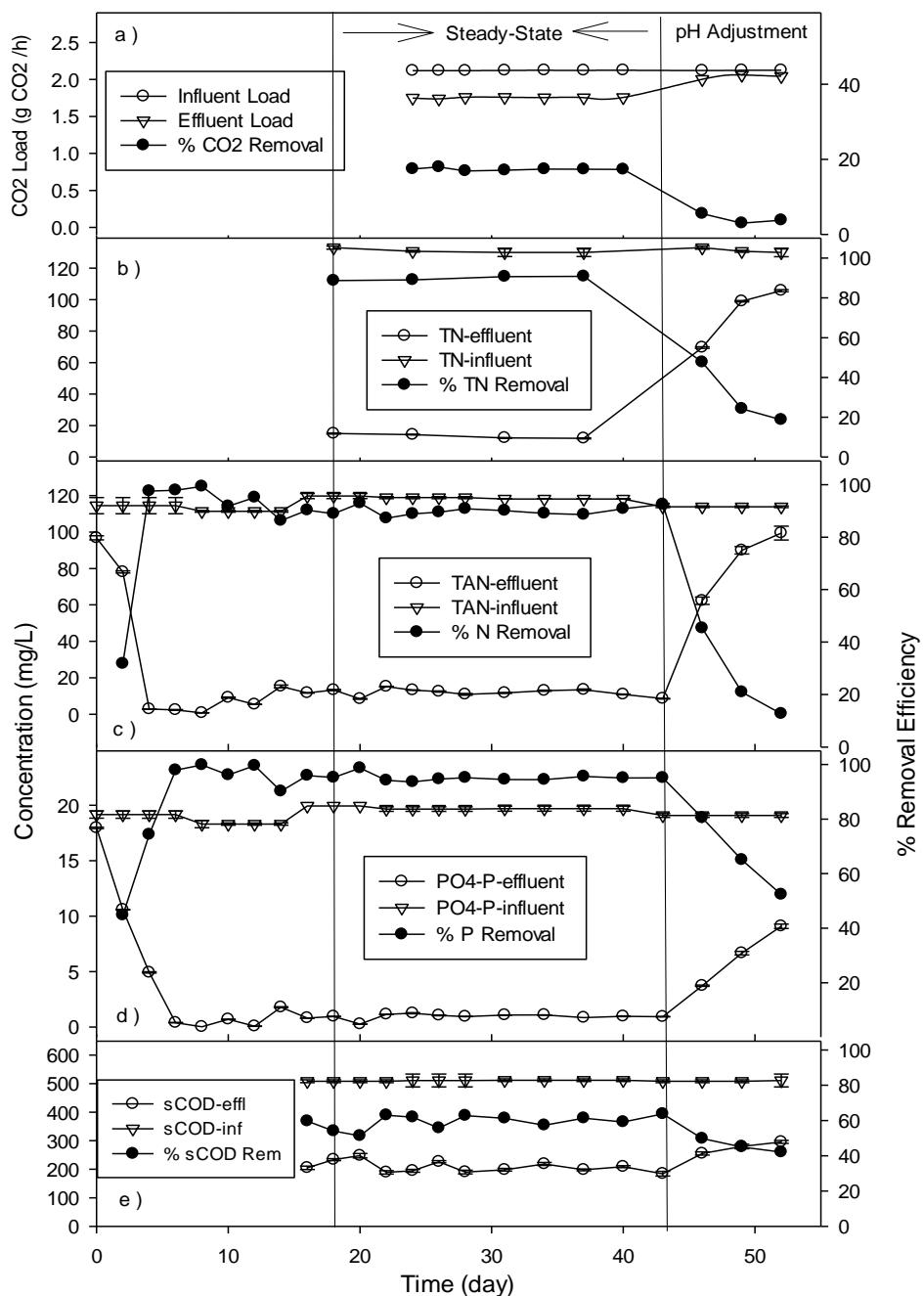
Figure 4-16 Change in parameters of C8 reactor with respect to time; a) CO<sub>2</sub> influent and effluent load, removal, b)TAN influent and effluent concentration, TAN removal c) TN influent and effluent concentration, TN removal, d) PO<sub>4</sub>-P influent and effluent concentration, PO<sub>4</sub>-P removal, e.) sCOD influent and effluent concentration and sCOD removal.
