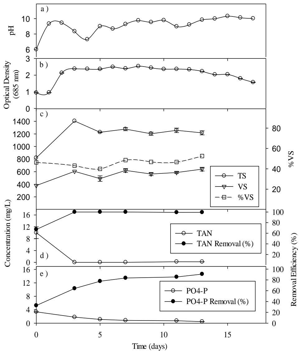
Figure 4-8 Change in parameters of X3 reactor with respect to time; a) pH, b) Optical density, c) TS concentration, VS concentration, %TVS, d) TAN effluent concentration, TAN removal efficiency, e) PO<sub>4</sub>-P effluent concentration, PO<sub>4</sub>-P removal efficiency.
