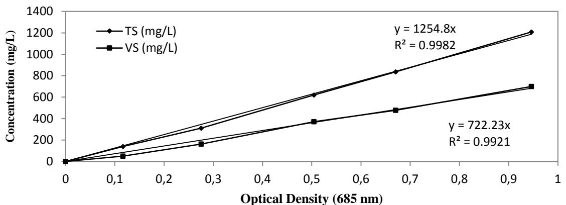
Figure D-1 Calibration curve and equation of optical density at 685 nm to TS and VS concentration of *Chlorella vulgaris* culture
