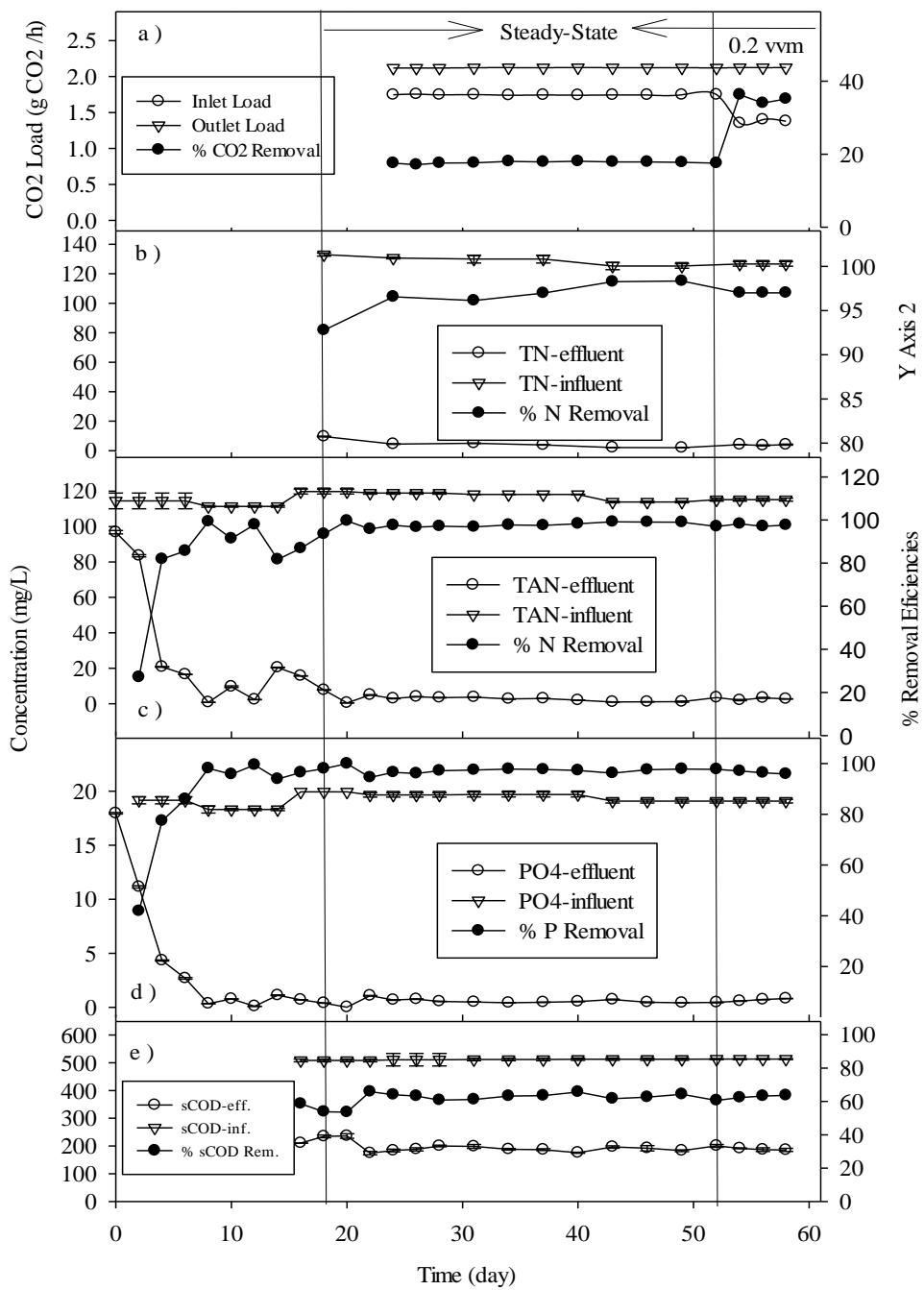
Figure 4-18 Change in parameters of reactor C12 with respect to time; a) CO<sub>2</sub> influent and effluent load, removal, b) TAN influent and effluent concentration, TAN removal c) TN influent and effluent concentration, TN removal, d) PO<sub>4</sub>-P influent and effluent concentration, PO<sub>4</sub>-P removal, e.) sCOD influent and effluent concentrations, sCOD removal.
