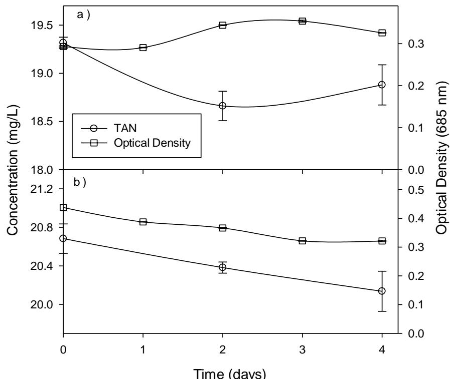
Figure 4-5 The change in TAN and optical density values in reactors a) B2-50 b)B2-100 with respect to time
