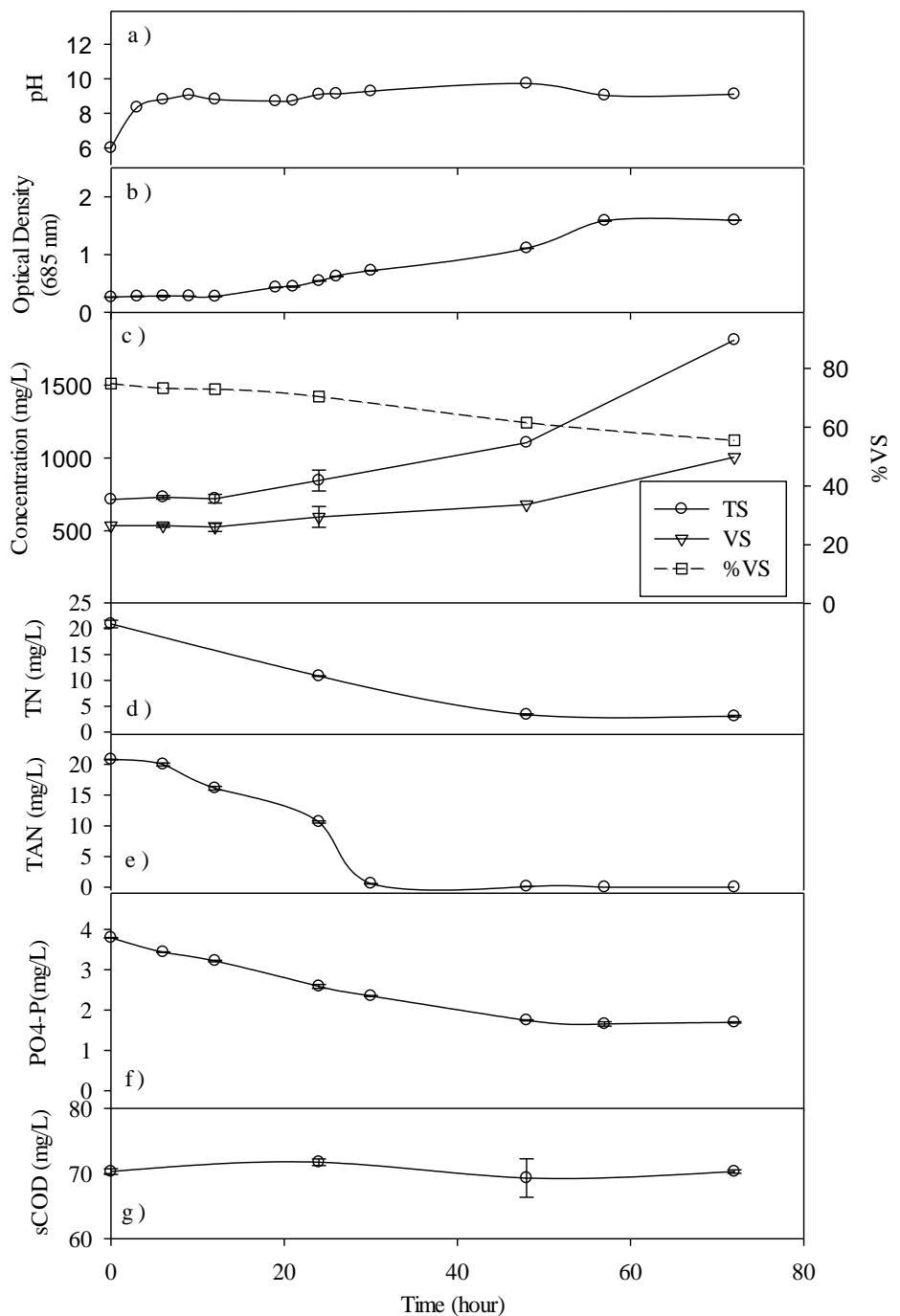
Figure 4-10 The change in parameters a) pH, b) Optical density, c) TS concentration, VS concentration, % VS, d) TN, e) TAN, f) PO<sub>4</sub>-P and g) sCOD in XB-2 reactor with respect to time
