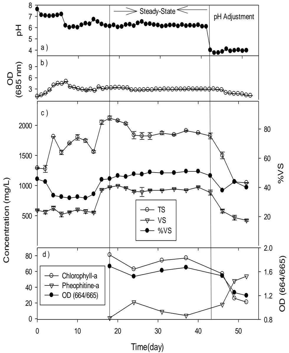
Figure 4-15 Change in parameters of C8 reactor with respect to time; a) pH, b) optical density at 685 nm, c) TS concentration, VS concentration, %VS, d) Chlorophyll-a, Pheophytine-a, OD (664<sub>b</sub>/665<sub>a</sub>).
