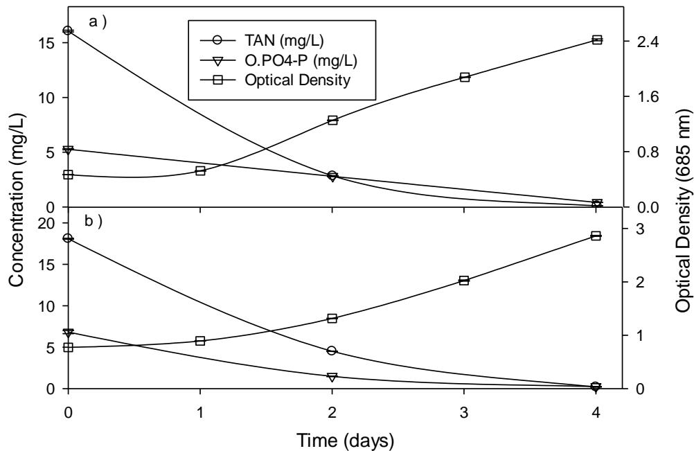
Figure 4-4 The change in TAN, PO<sub>4</sub>-P and optical density values in reactors a) B1-50, b) B1-100 with respect to time
