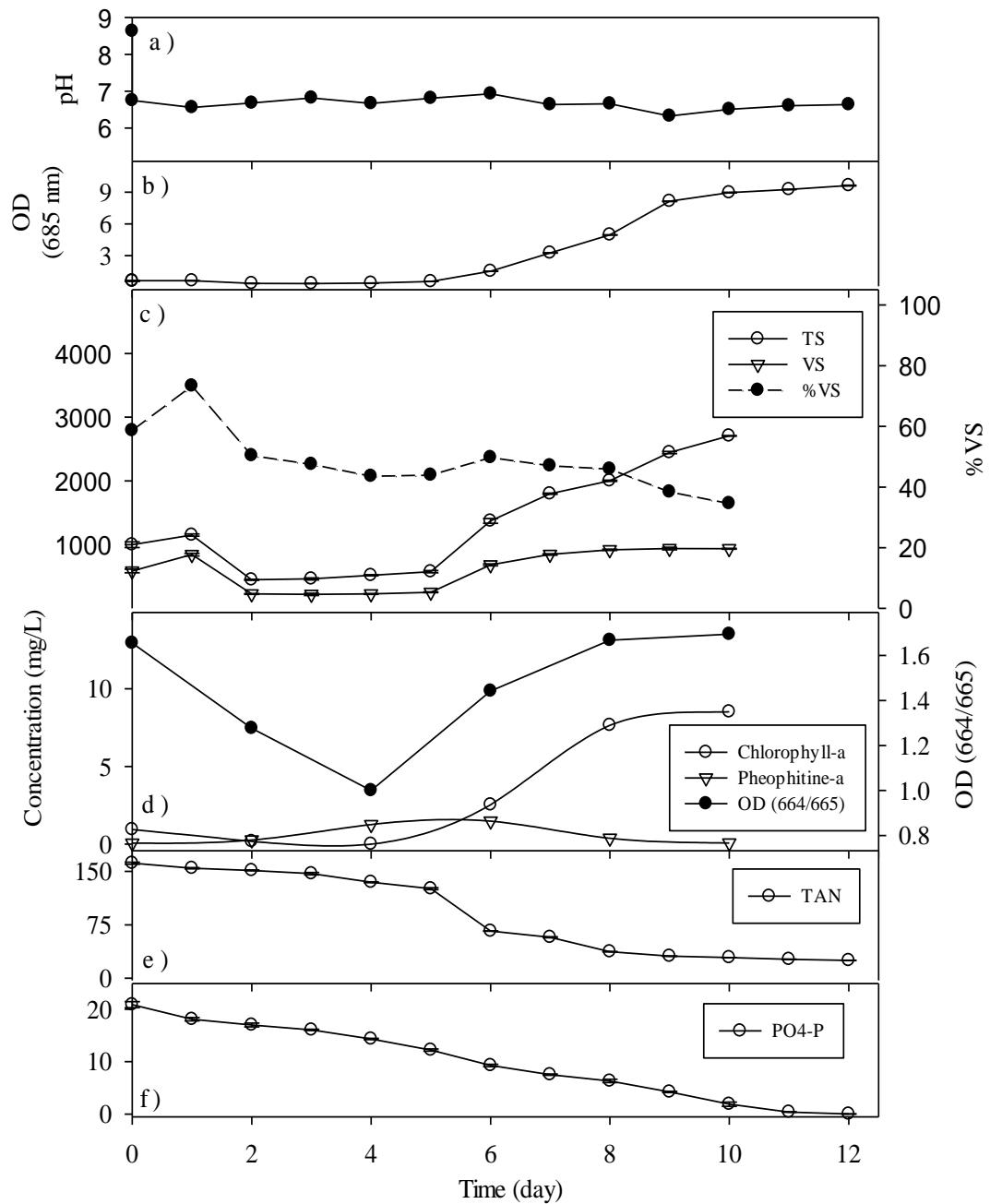
Figure 4-12 Change in a) pH, b) Optical Density (685 nm ), c) TS concentration, VS concentration, %VS, d) Chlorophyll-a, Pheophytine-a, OD (664<sub>b</sub>/665<sub>a</sub>), e) TAN, f) PO<sub>4</sub>-P Parameters of CB8 Reactor with respect to time
