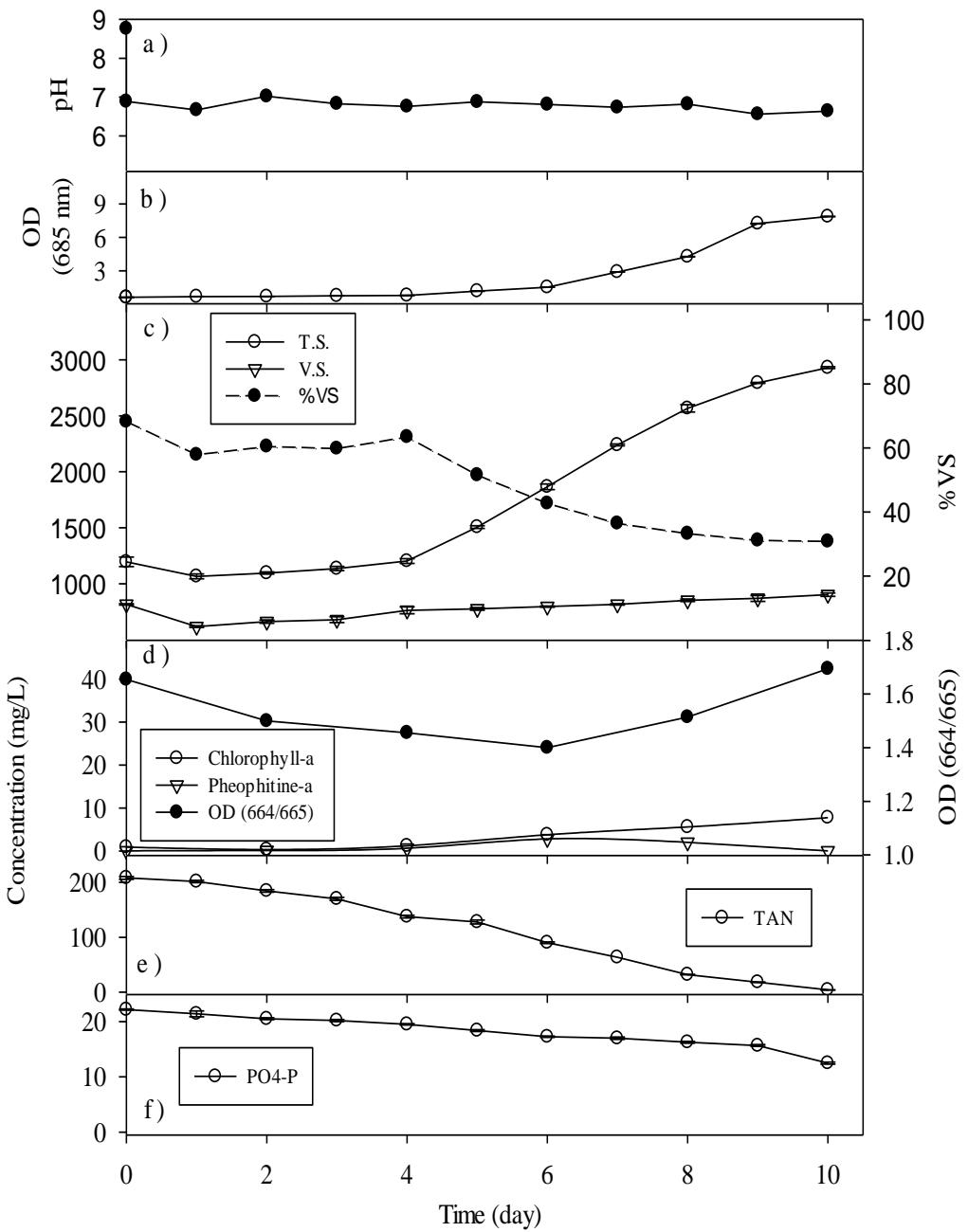
Figure 4-13 Change in a) pH, b) Optical Density ( 685 nm ), c.) TS concentration, VS concentration, %TVS, d) Chlorophyll-a, Pheophytine-a, OD (664<sub>b</sub>/665<sub>a</sub>), e) TAN, f) PO<sub>4</sub>-P parameters of CB10 Reactors with respect to time
