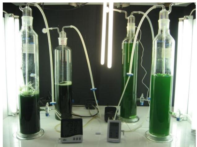
Figure 3-2 PBRs for cultivation of microalgal biomass
