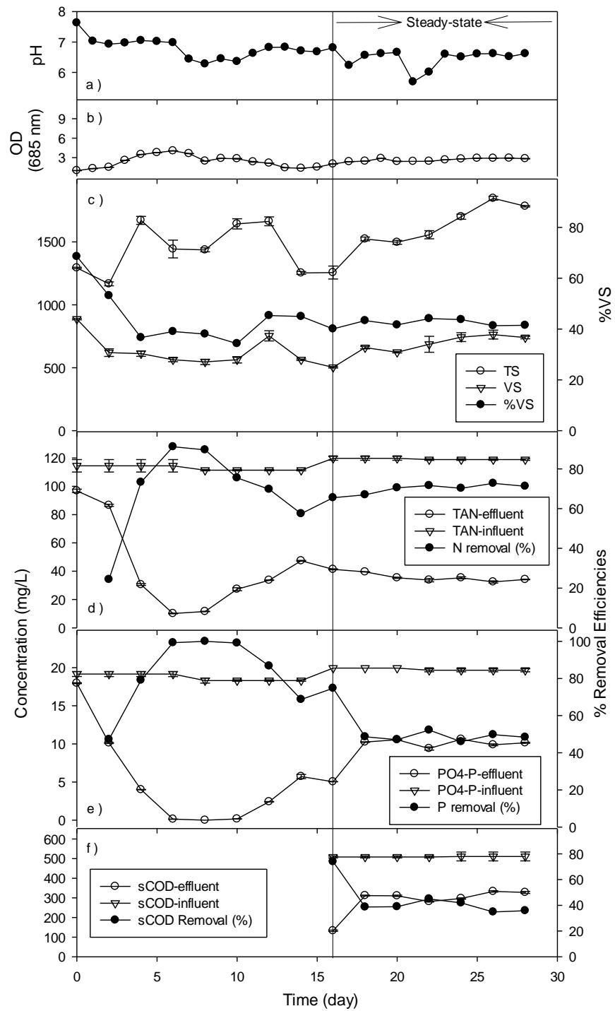
Figure 4-14 Change in parameters of C5 reactor with respect to time; a) pH, b) optical density at 685 nm, c) TS concentration, VS concentration, % VS, d)TAN, e) PO<sub>4</sub>-P, f) sCOD.
