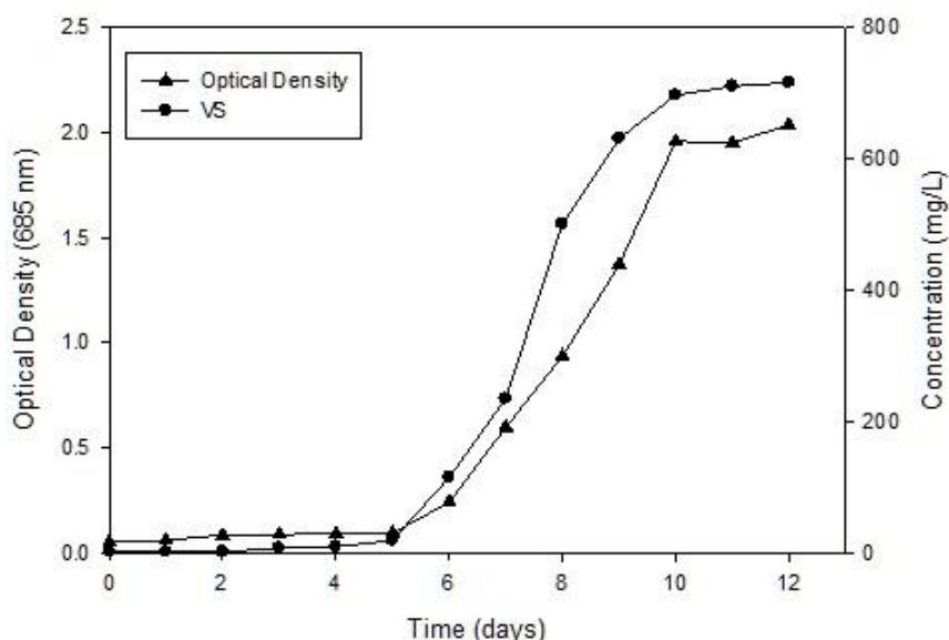
Figure 4-1 The change in optical density and VS concentration in batch cultivation reactor of *Chlorella vulgaris*
