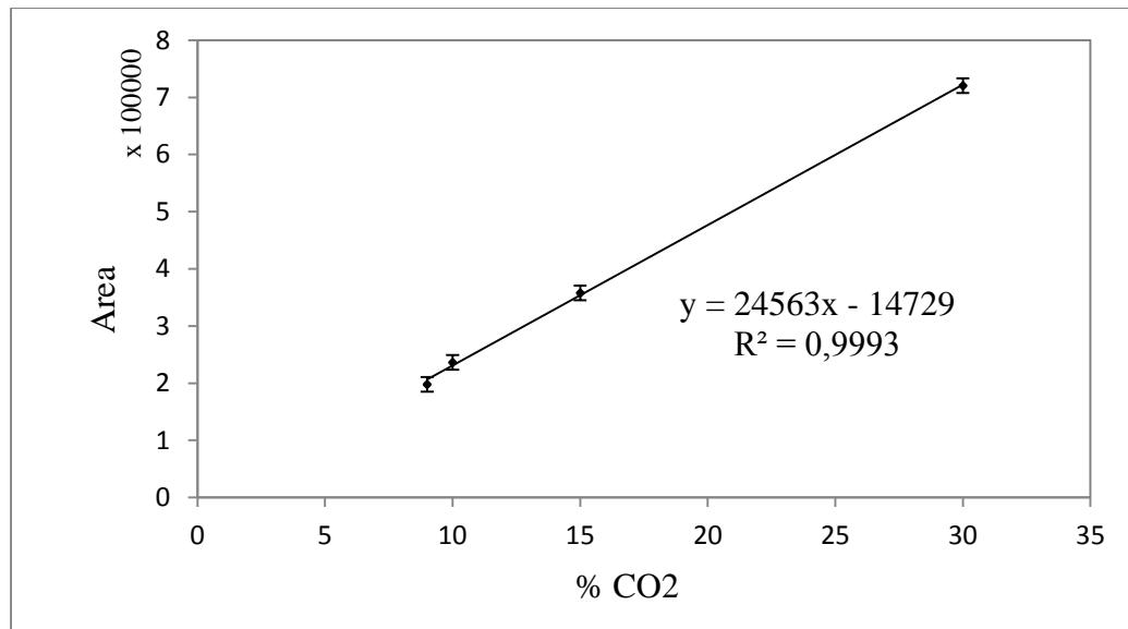
Figure B-1 Calibration curve and equation for CO<sub>2</sub>
