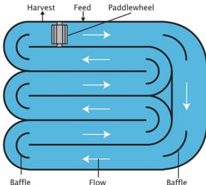
Figure 2-3 A representative raceway open pond (Johnson et al., 2009)
