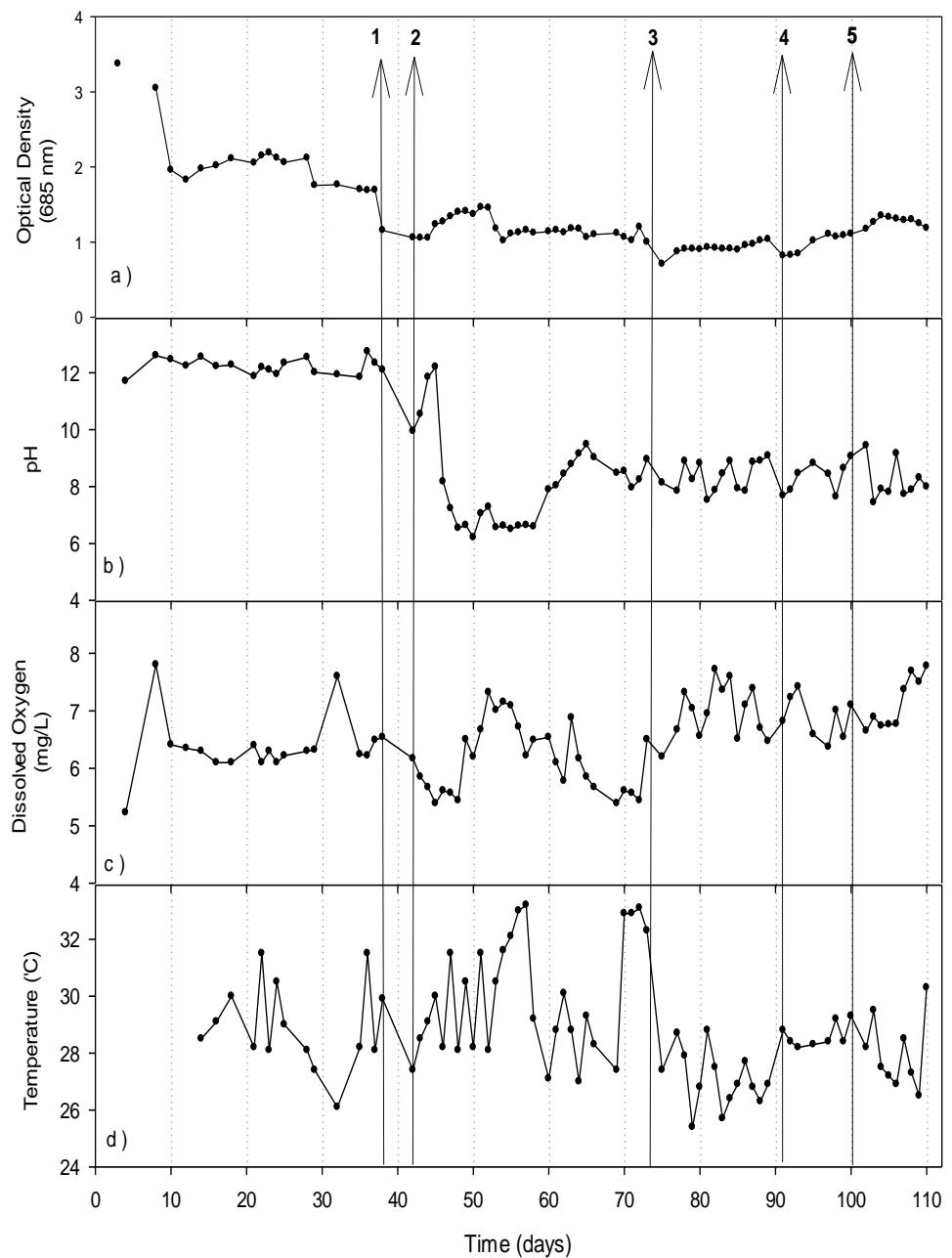
Figure 4-3 The change in physical parameters; a) Optical Density, b) pH, c) Dissolved Oxygen, d) Temperature, in R2 cultivation reactor with respect to time.
