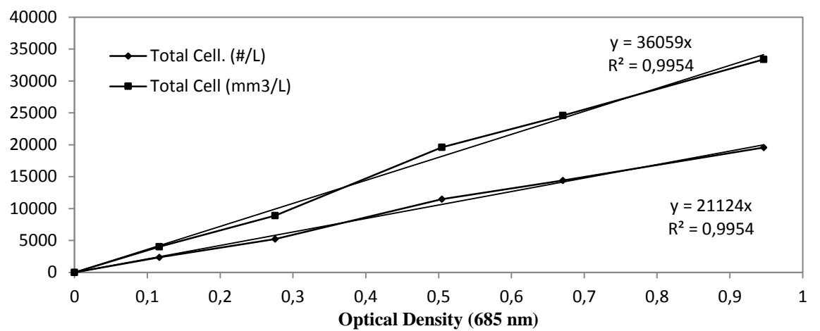
Figure D-3 Calibration curve and equation of optical density at 685 nm to total cell number and volume of *Chlorella vulgaris* culture
