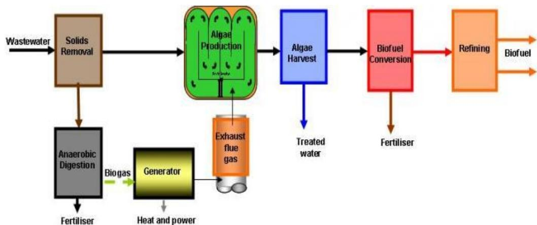
Figure 1-1 Scheme of algal system (Craggs, 2009)
