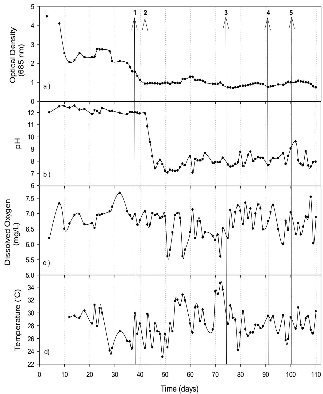
Figure 4-2 The change in physical parameters; a ) Optical Density, b ) pH, c ) Dissolved Oxygen, d ) Temperature, in R1 cultivation reactor with respect to time.
