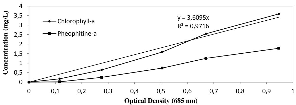
Figure D-2 Calibration curve and equation of optical density at 685 nm to chlorophyll-a concentration of *Chlorella vulgaris* culture
