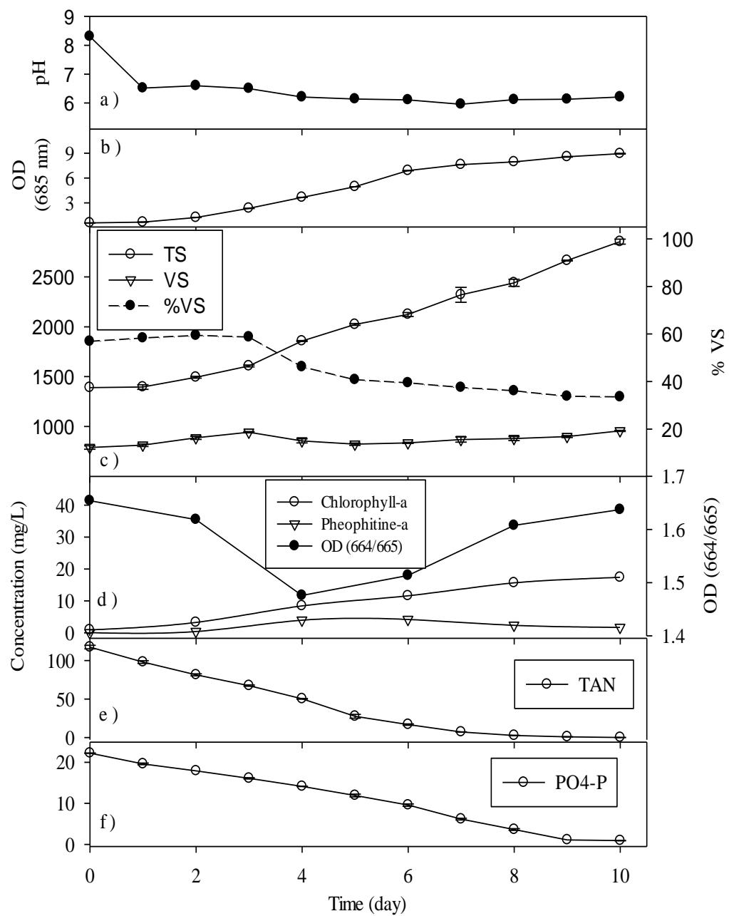
Figure 4-11 Change in a) pH, b) Optical Density (685 nm ), c) TS concentration, VS concentration, %VS, d) Chlorophyll-a, Pheophytine-a, OD (664<sub>b</sub>/665<sub>a</sub>), e) TAN, f) PO<sub>4</sub>-P parameters of CB6 reactor with respect to time.
