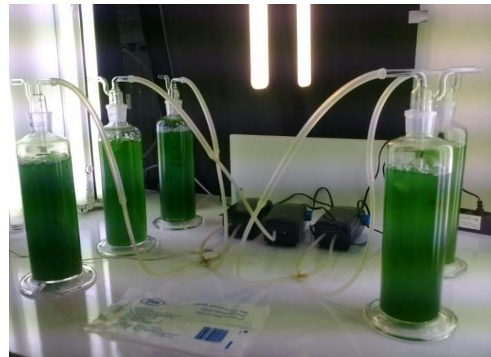
Figure 3-3 PBRs used in wastewater treatment studies
