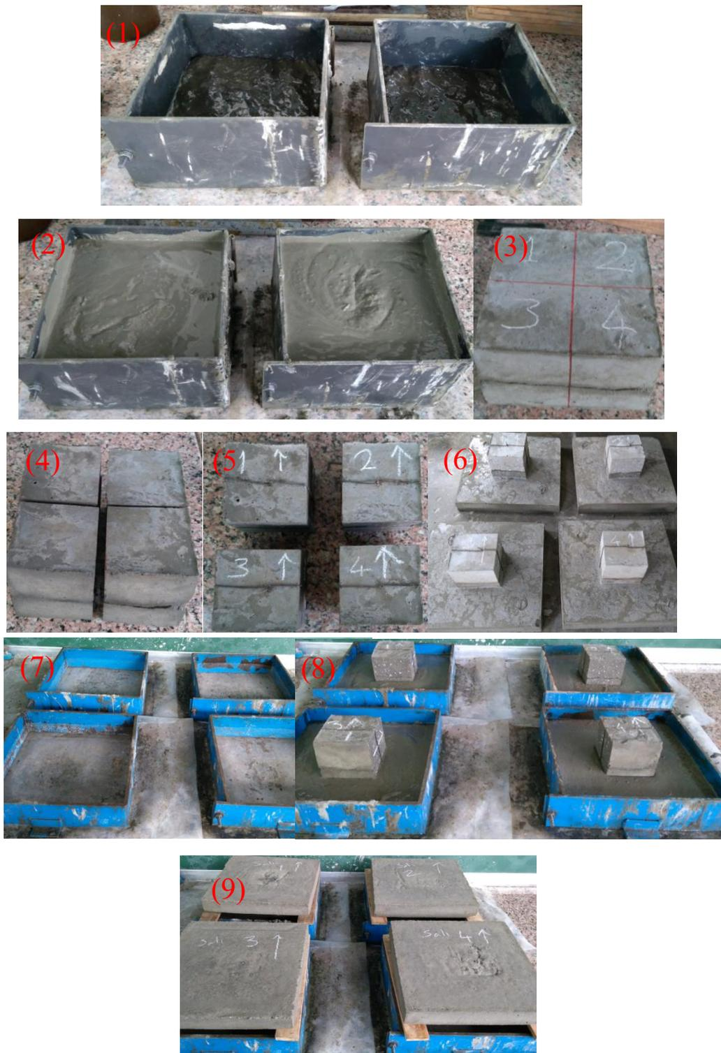
Figure 6.4. Casting 10 cm x 10 cm size specimens
