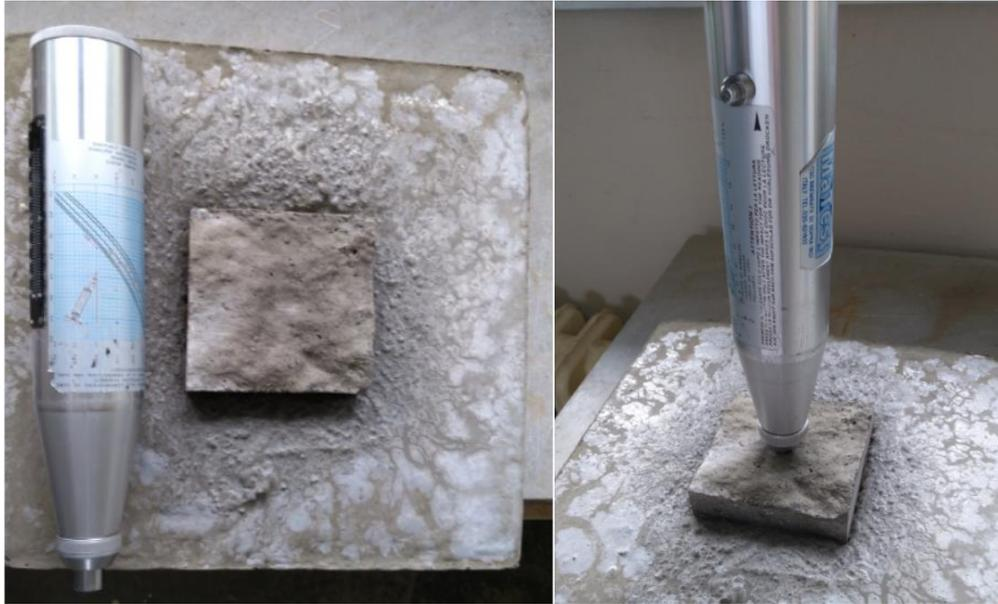
Figure 6.19. Application of Schmidt Hammer
