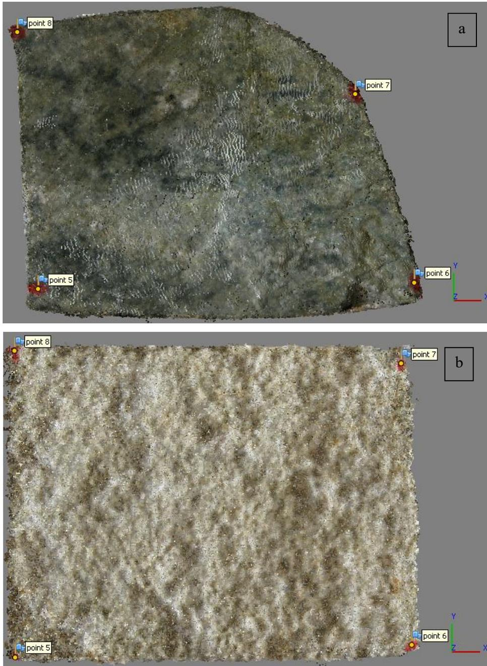
Figure 4.6. Dense clouds of specimens; (a) specimen A, (b) specimen B
