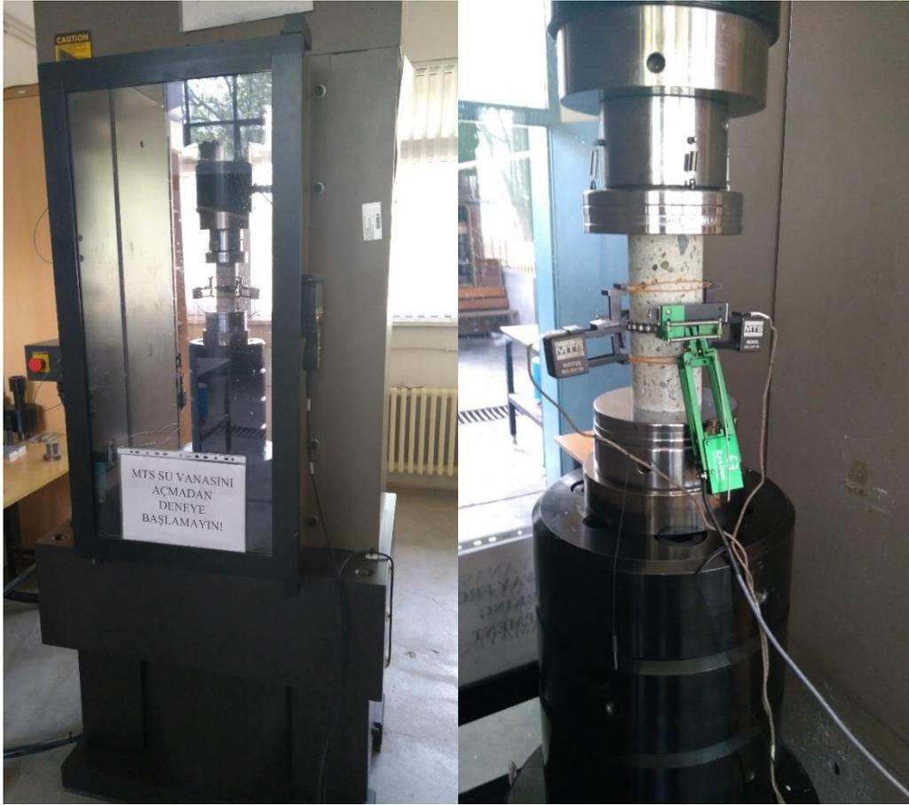
Figure 6.14. Uniaxial compressive strength test
