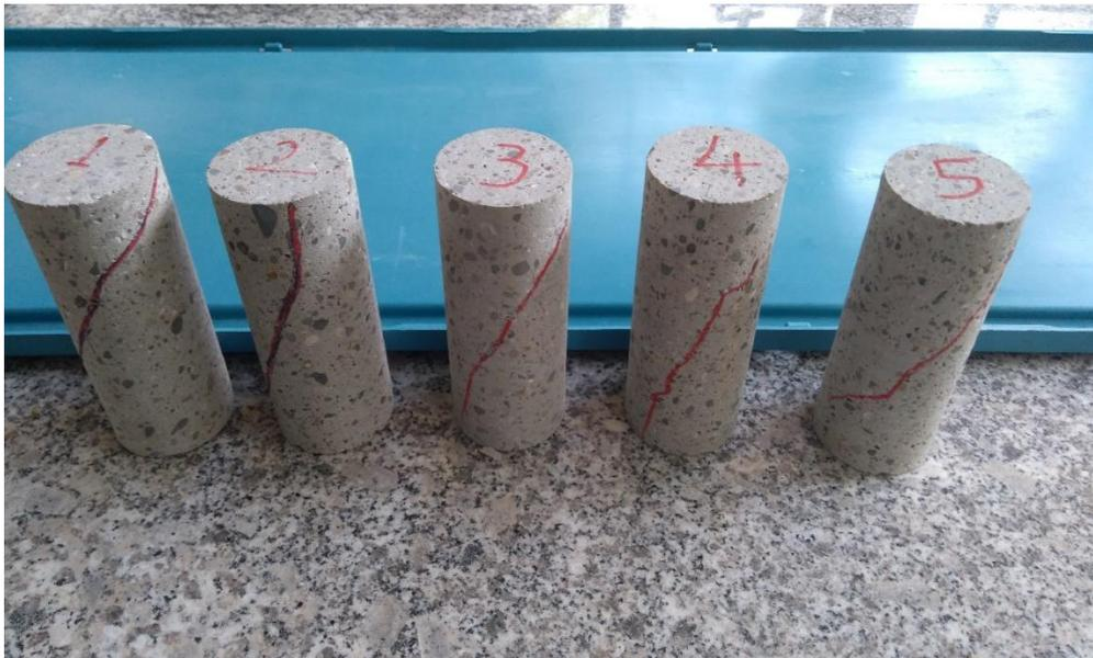
Figure 6.15. Specimens after the UCS test
