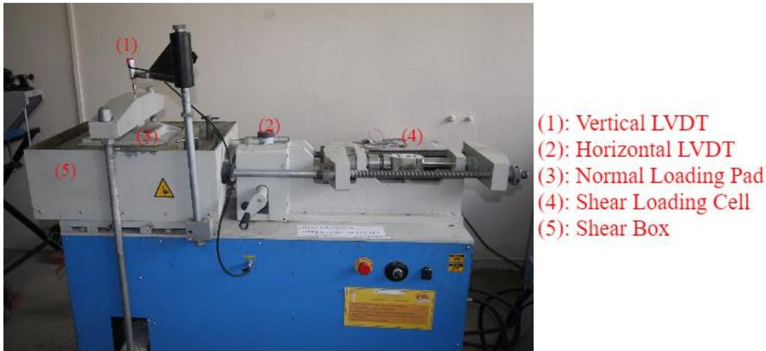
Figure 6.11. Direct Shear Test Equipment
