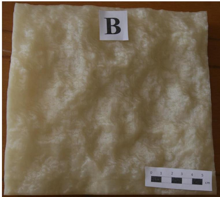
Figure 5.2. 3D printed rock discontinuity surface replicas
