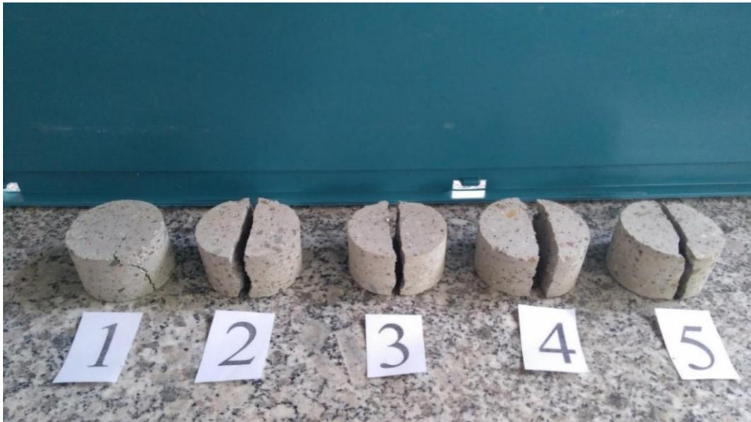
Figure 6.18. Specimens after the Brazilian test
