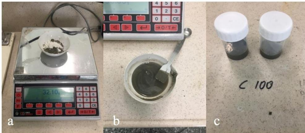
**Figure 5-1: Slurry Preparation for Heat of Hydration Determination**
