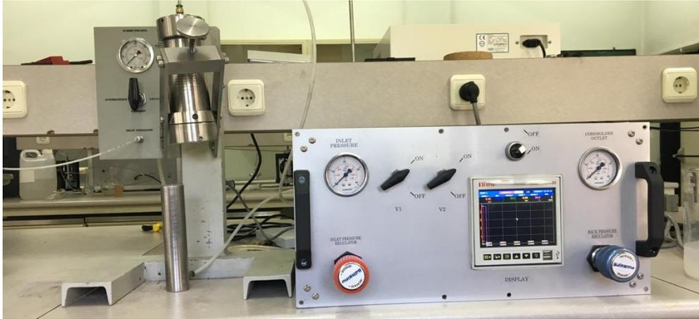
**Figure 5-7: Steady state gas permeameter**
