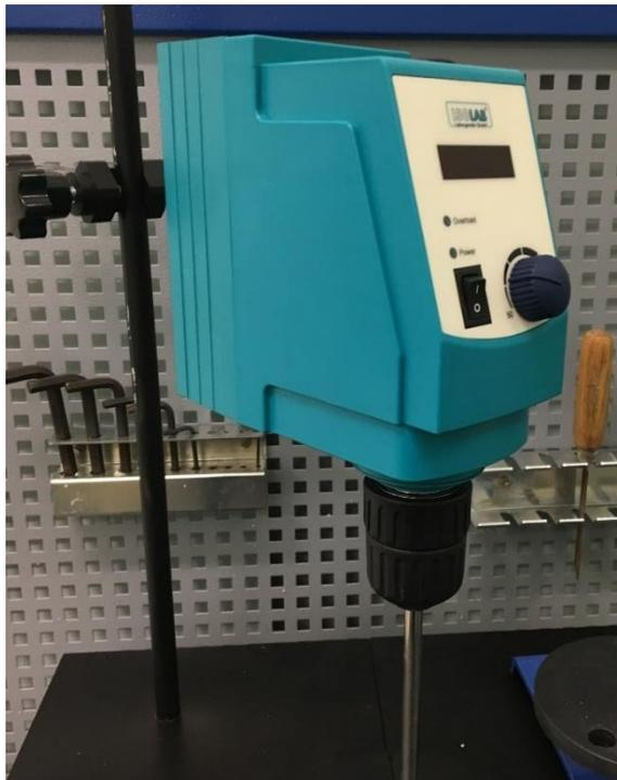
**Figure F-4: Isolab high speed mixer**
