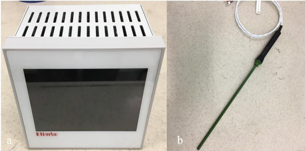
**Figure F-1: a) PR-110 data logger b) Pt-100 thermometer**
