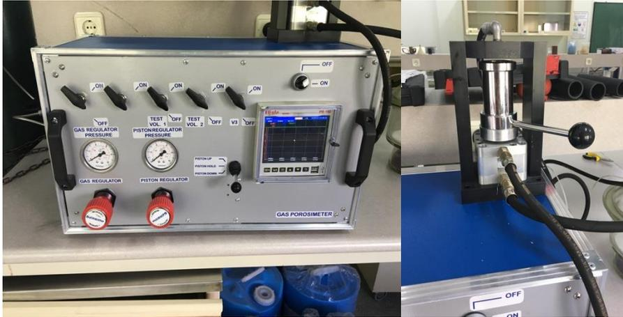
**Figure 5-6: Helium Porosimeter**
