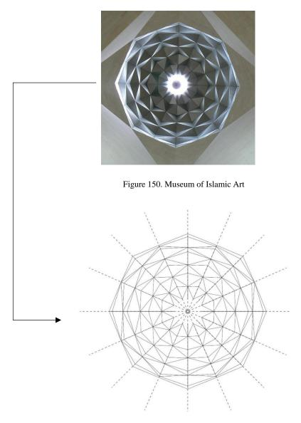
Figure 151. Decomposition of the pattern to its sectors
