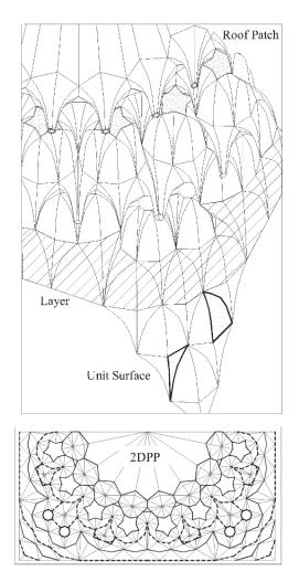
Figure 57. The basic parts of the Muqarnas (Web 37)
