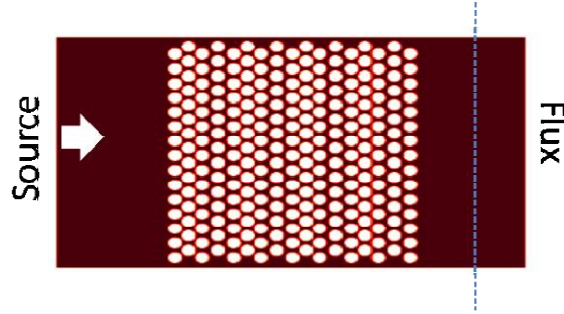
Figure 4.8 - Schematic of Crystal-Crystal superlattice with 3 holes in each side where one column of holes (air) is in common for both sides.
