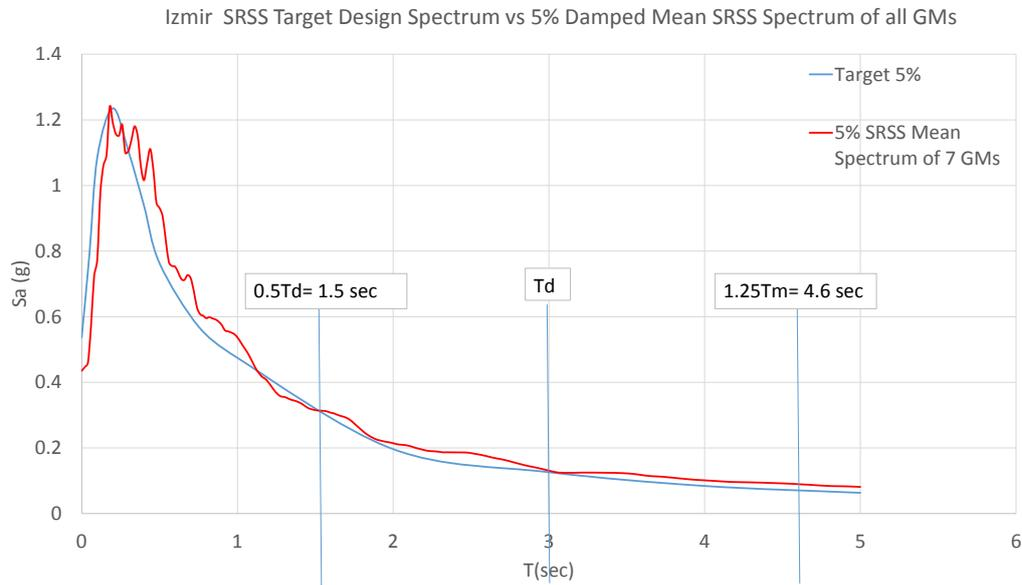
Figure 2.28: Izmir 5% Damped SRSS Target Spectrum vs 5% Damped SRSS Mean Spectrum of 7 GMs
