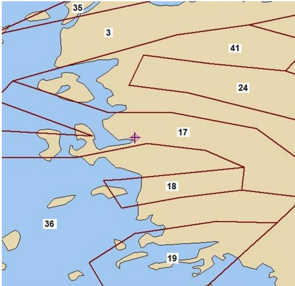
Figure A.1: Dominant seismic sources for Izmir site
